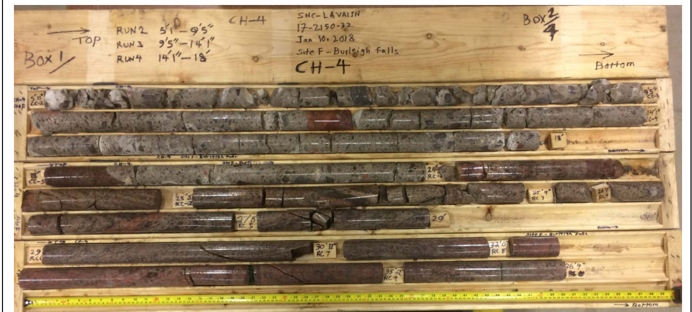
Site F – Burleigh Falls – CH17-104 - Wet rock cores
