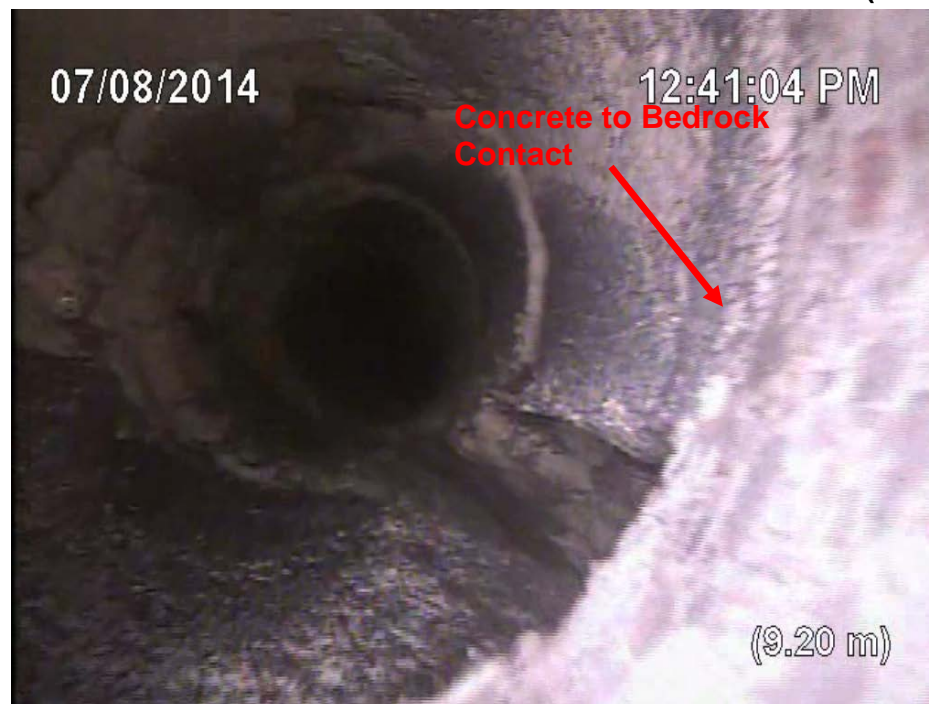
PHOTO 4.1-6 CONCRETE TO BEDROCK CONTACT AT SOUTH ABUTMENT PIER (CH14-101)
