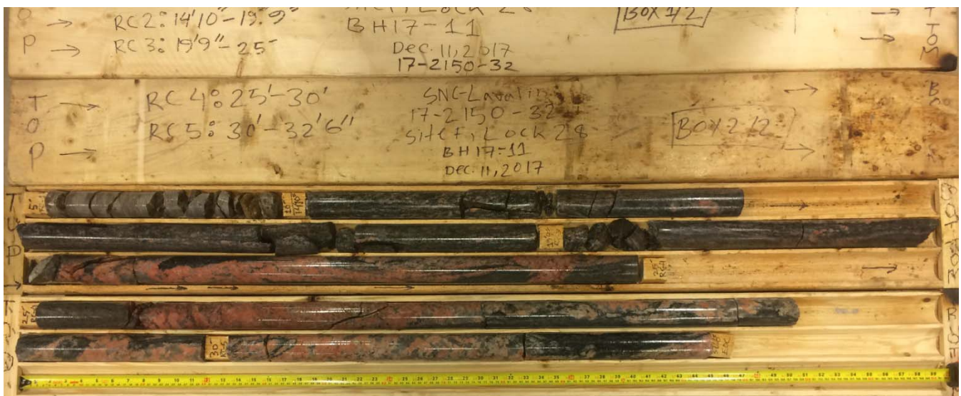
Site F – Burleigh Falls – BH17-11 - Wet rock cores
