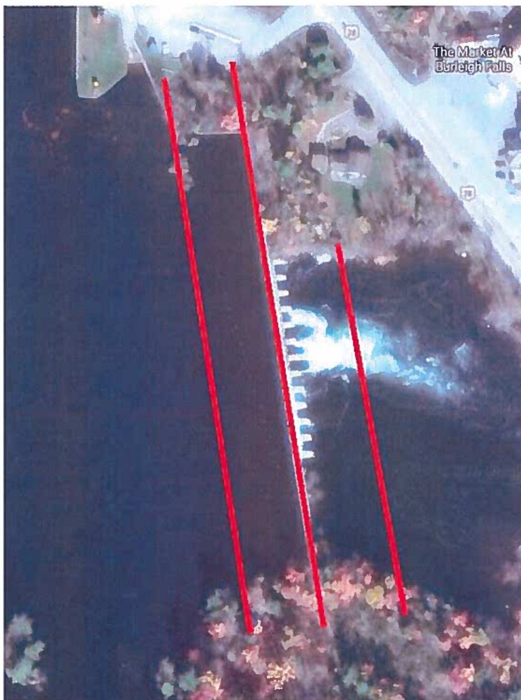
Figure 7. Proposed lines of Geotechnical Investigations at Burleigh Falls Dam at Lock 28 (Burleigh Falls), Kawartha Sector (PCA files).
