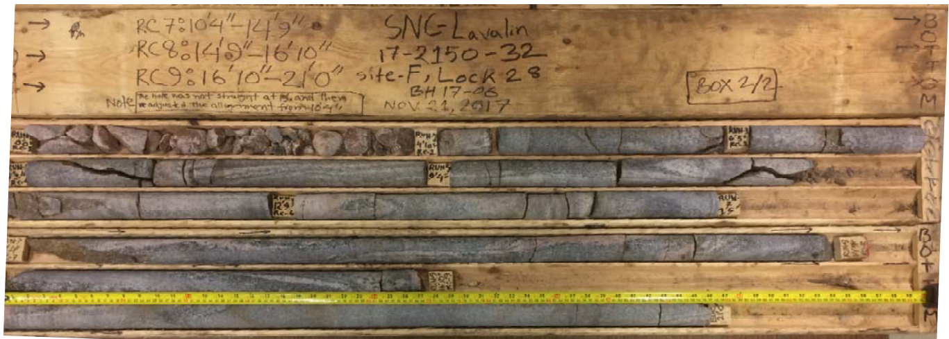
Site F – Burleigh Falls – BH17-06 - Dry rock cores
