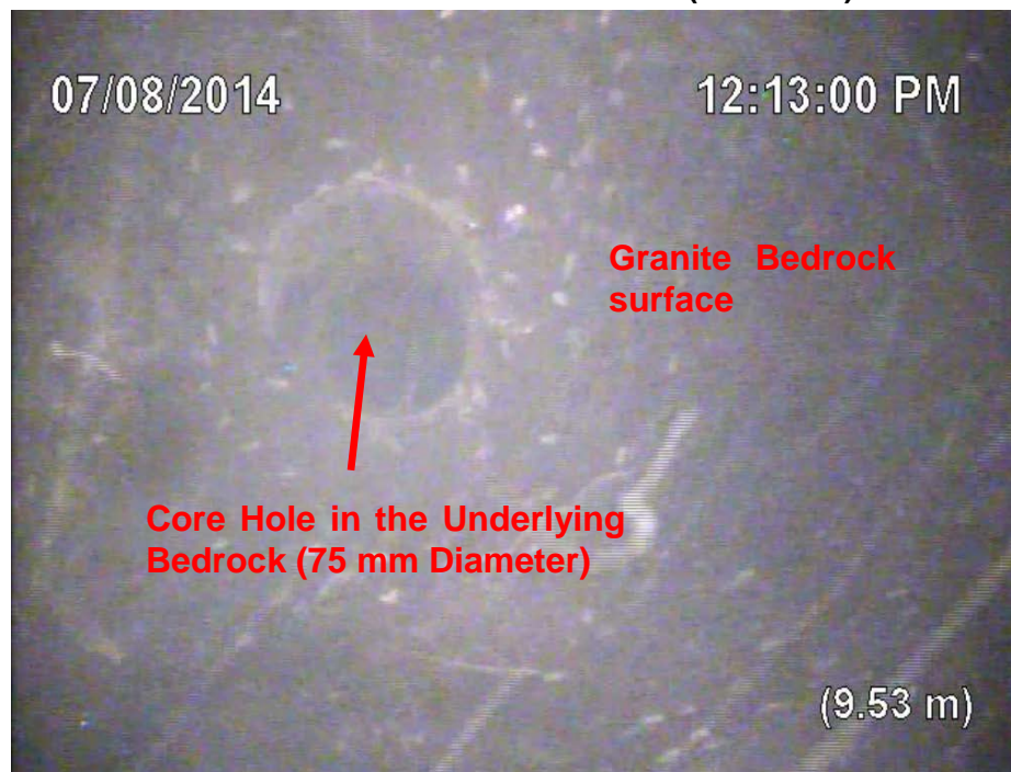
PHOTO 4.1-4 CONDITION OF VOID AT PIER #1 (CH14-103)
