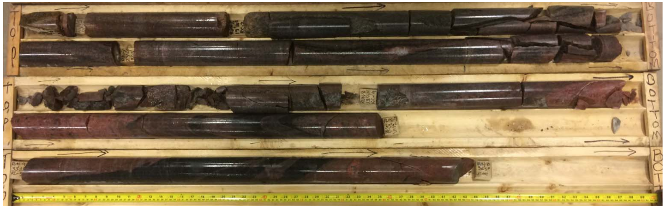
Site F – Perry's Creek – CH17-01 - Wet rock cores
