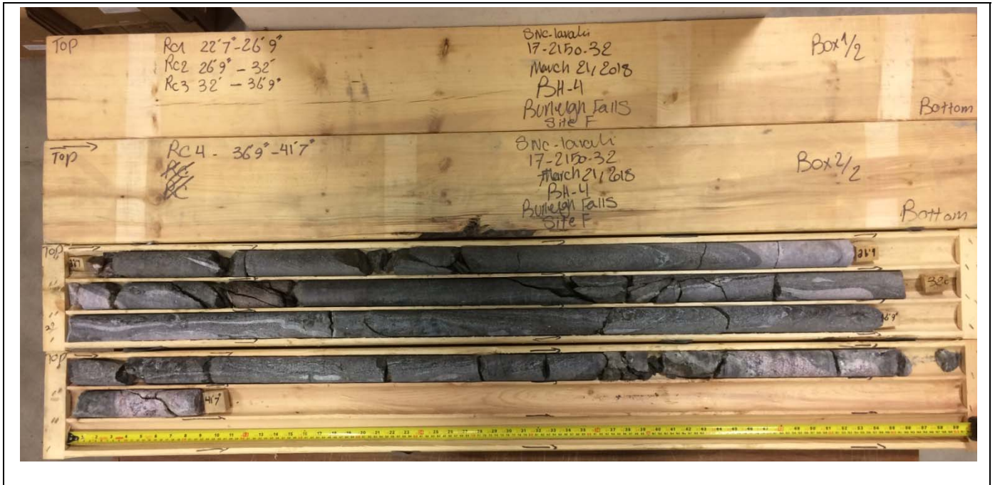
Site F – Burleigh Falls – BH17-104 - Dry rock cores
