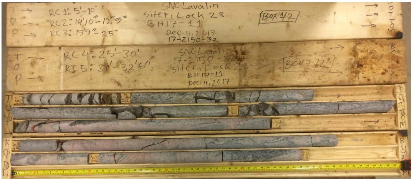
Site F – Burleigh Falls – BH17-11 - Dry rock cores
