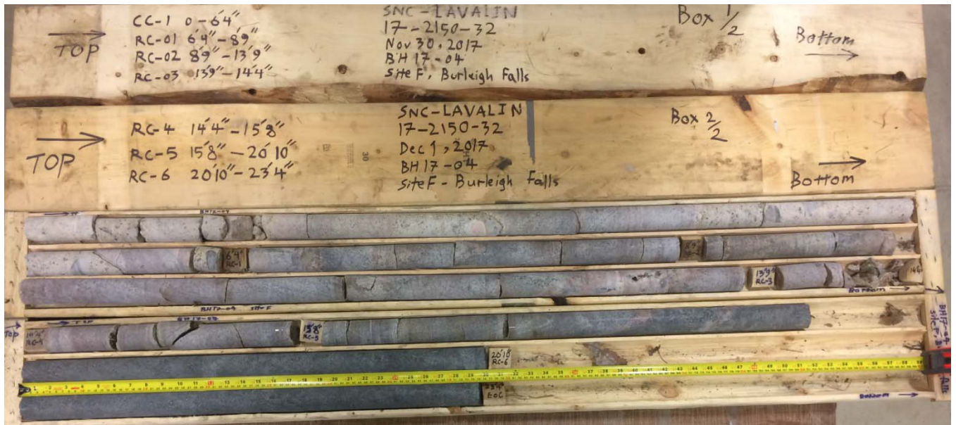
Site F – Burleigh Falls – BH17-04 - Dry rock cores
