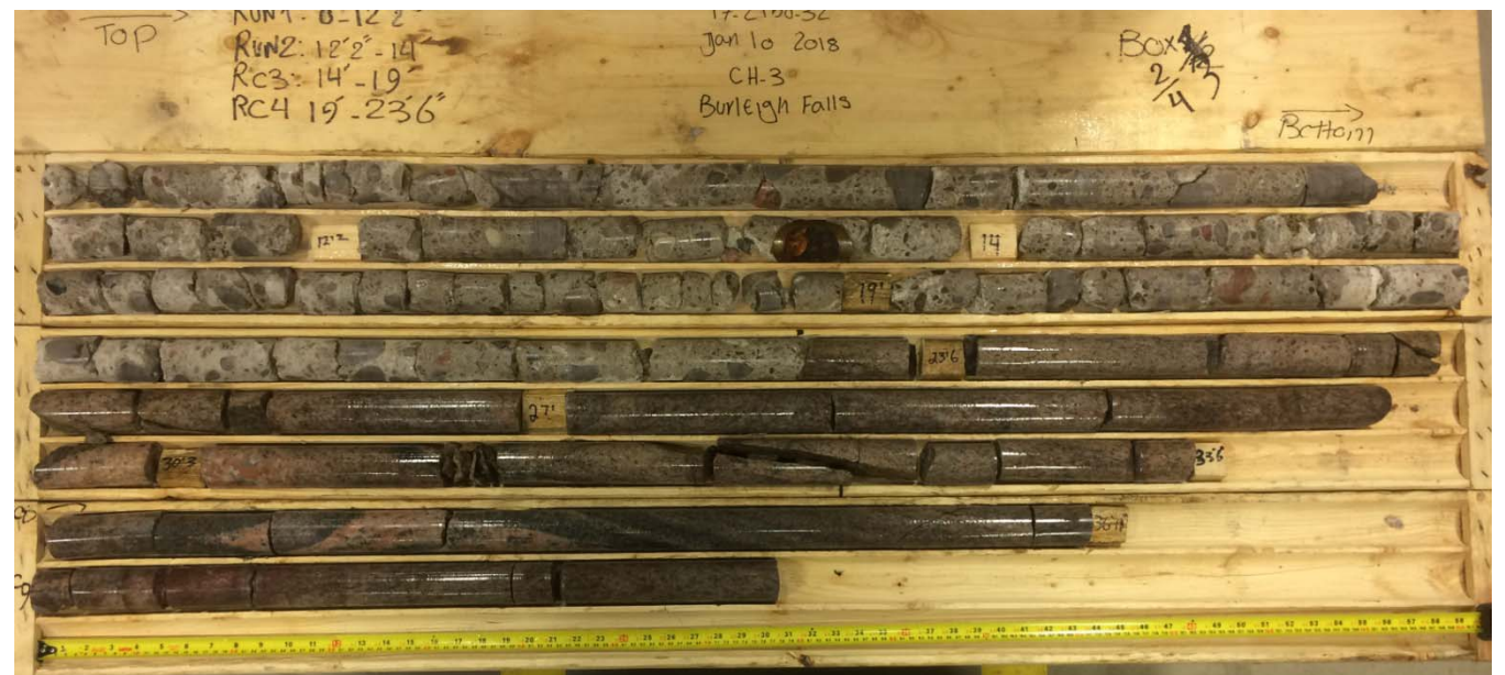
Site F – Burleigh Falls – CH17-103 - Wet rock cores
