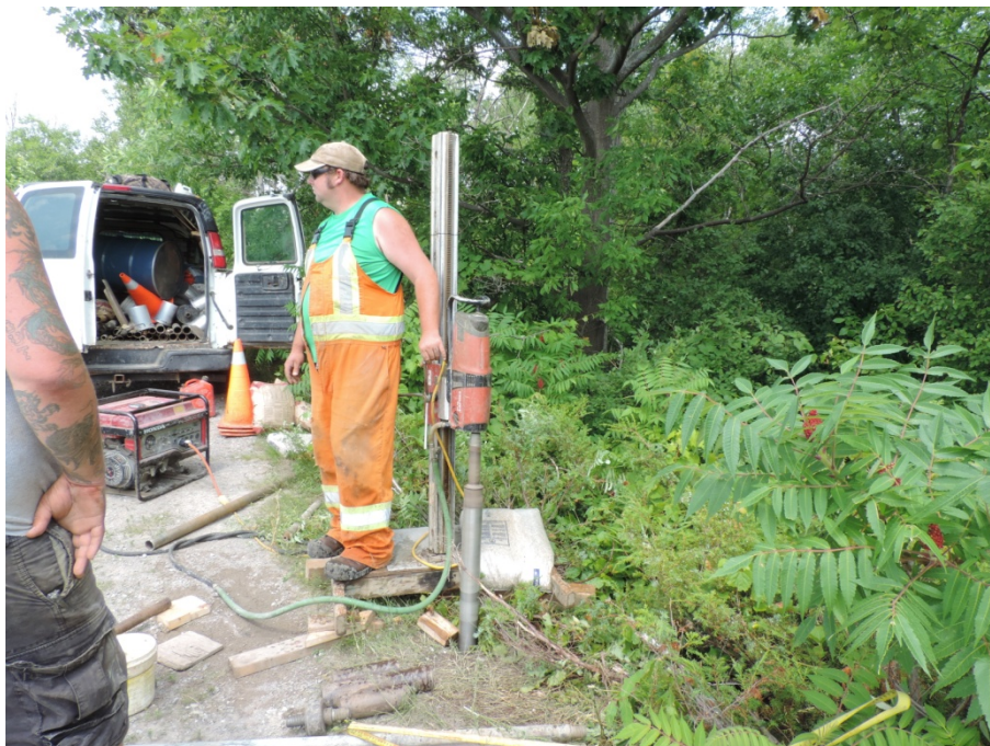
PHOTO 3.1-2 PORTABLE DRILL RIG AT TH14-102
