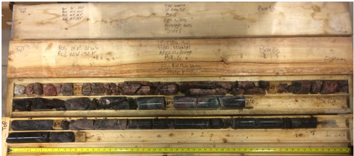
Site F – Burleigh Falls – BH17-106 - Wet rock cores
