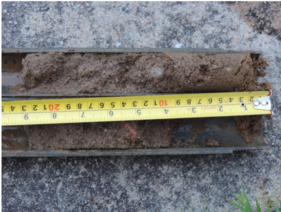
North (Left) Earthfill Embankment Sand Fill
