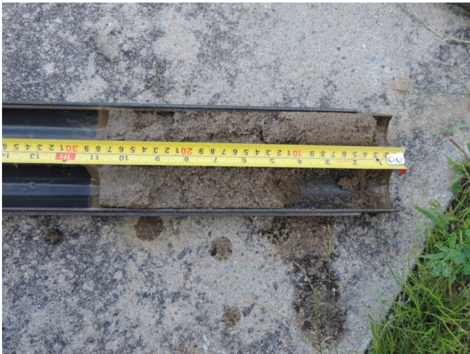
North (Left) Earthfill Embankment Sand Fill
