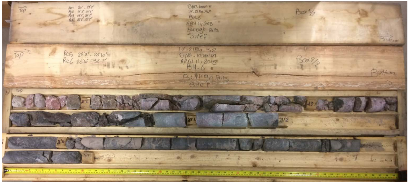
Site F – Burleigh Falls – BH17-106 - Dry rock cores
