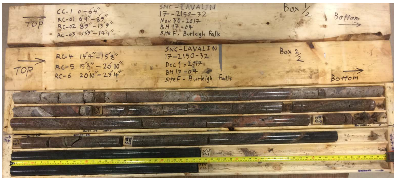
Site F – Burleigh Falls – BH17-04 - Wet rock cores
