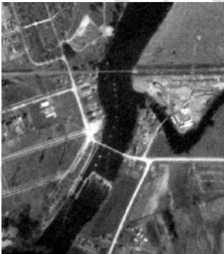
Figure 7: Scott's Mills lock 1929 – note line of timber crib caps in waterway. [National Air Photo Library]
