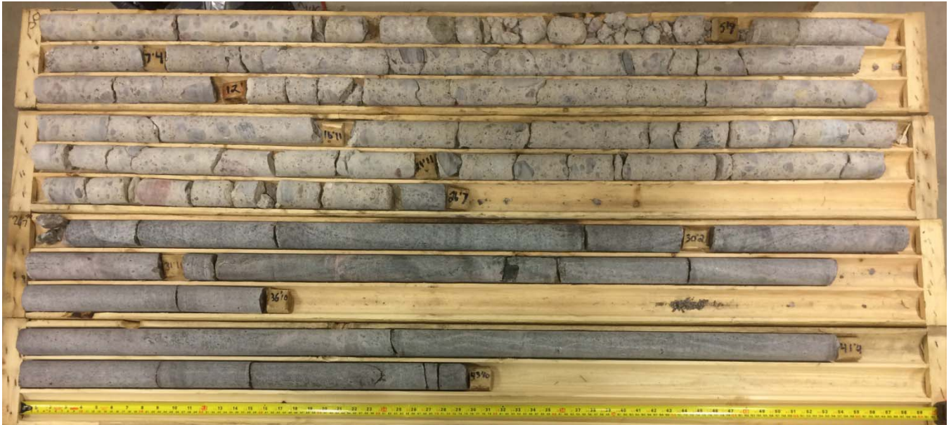
Site F – Burleigh Falls – CH17-102 - Dry rock cores
