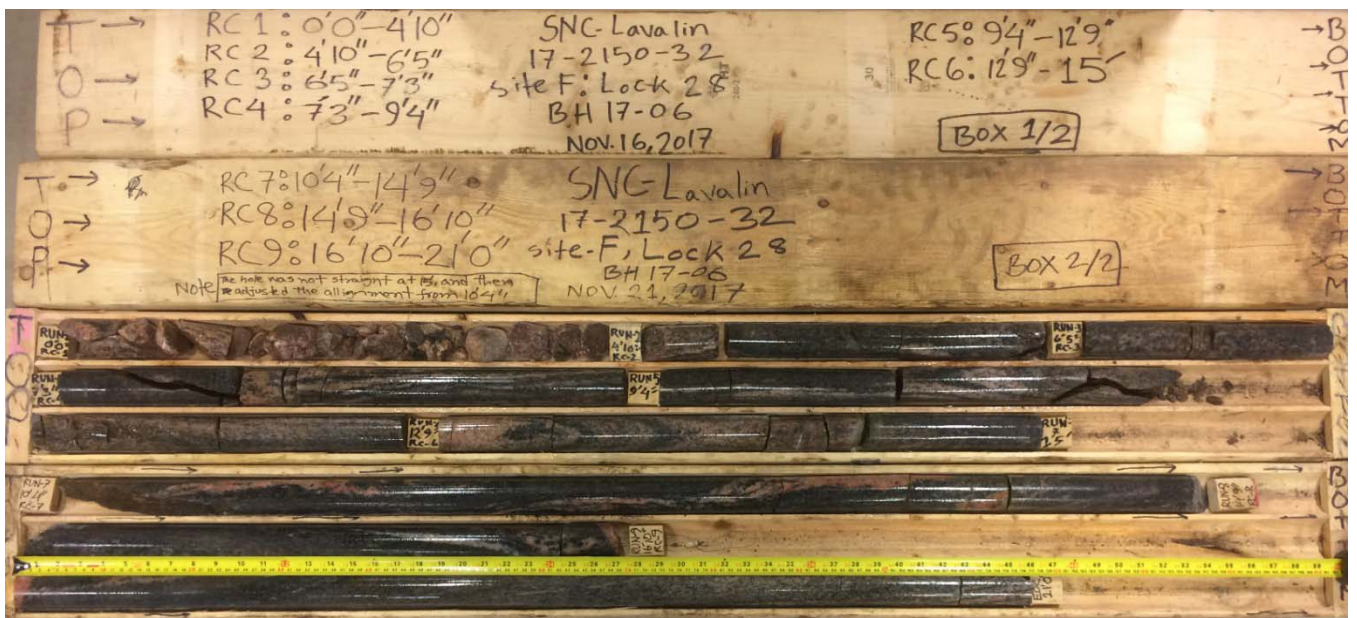
Site F – Burleigh Falls – BH17-06 - Wet rock cores
