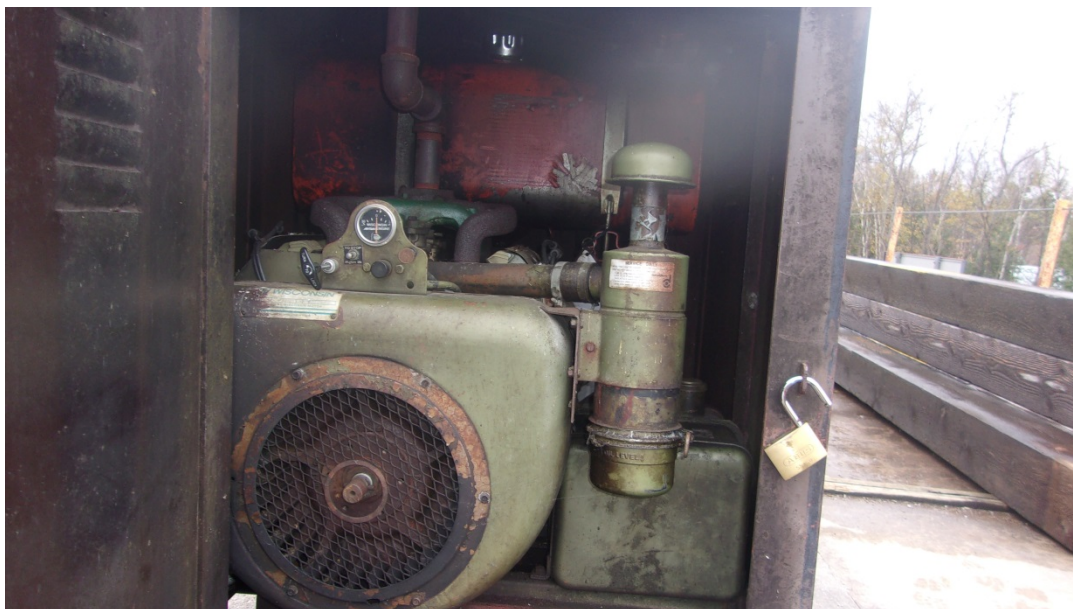
Photograph 6: Petroleum products and battery within hydraulic stop log lifter
