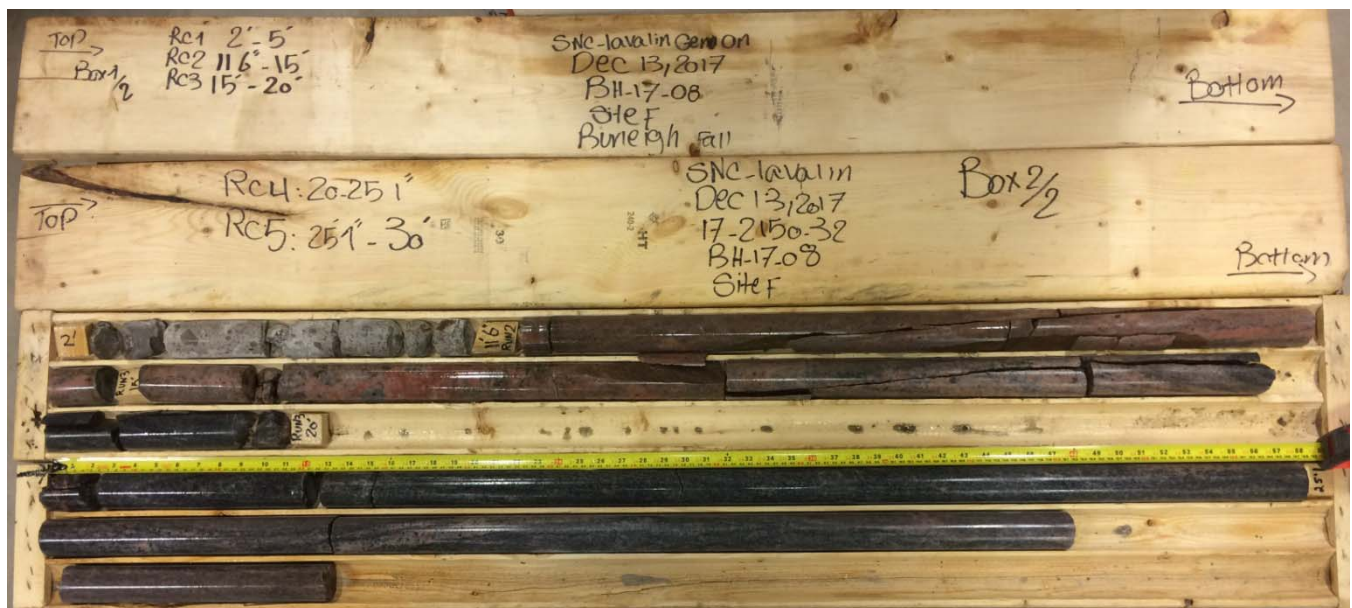
Site F – Burleigh Falls – BH17-08 - Wet rock cores
