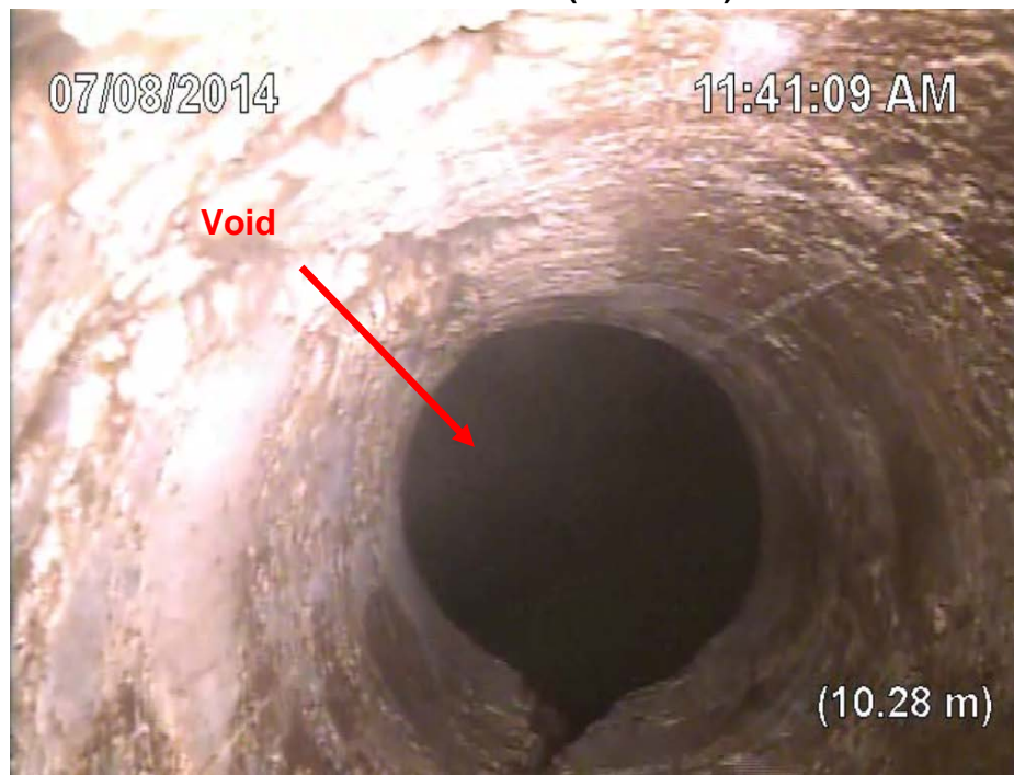
PHOTO 4.1-1 VOID AT PIER #1 (CH14-102)
