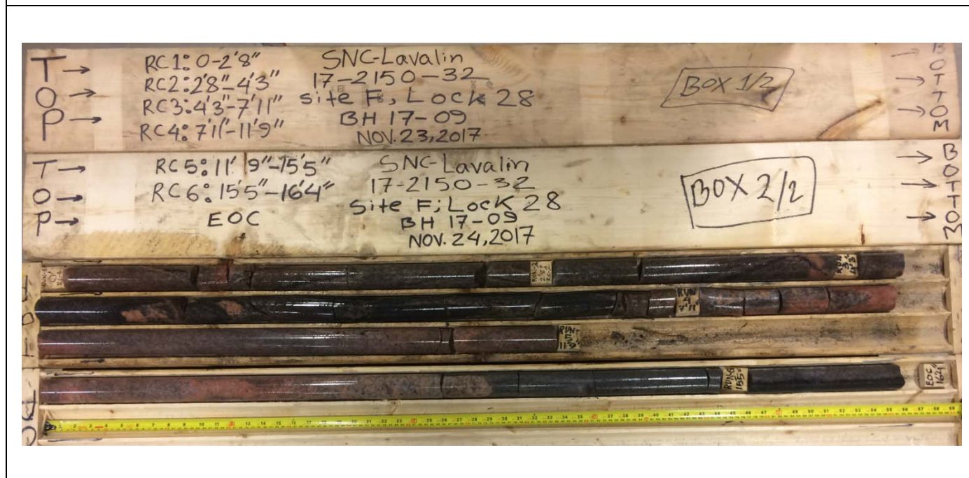
Site F – Burleigh Falls – BH17-09 - Wet rock cores
