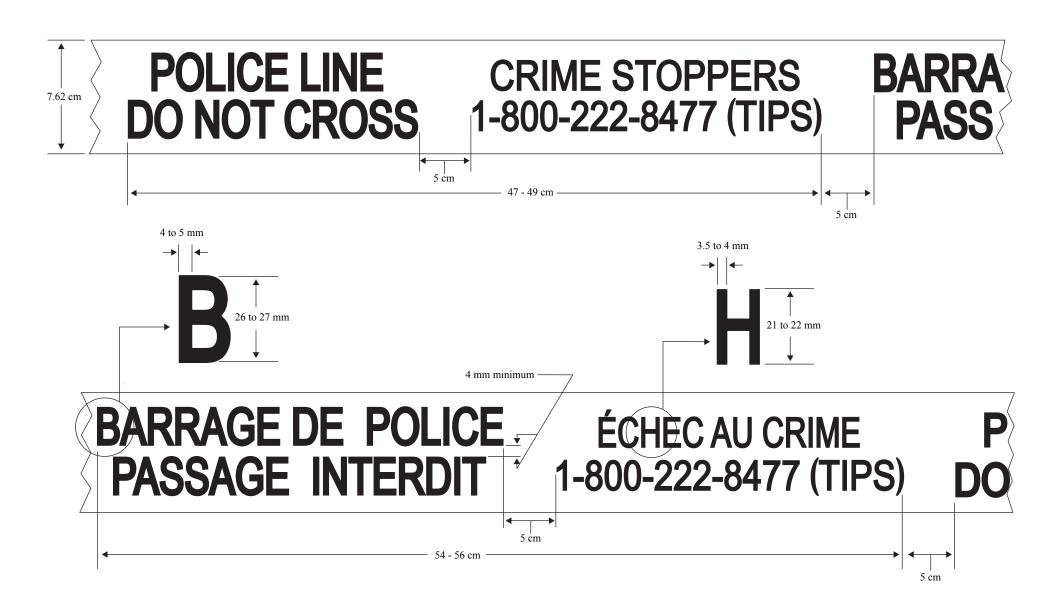
Other than the lettering thickness and the tape width, all measurements are subject to a 5 mm tolerance. Tape width tolerance is  $\pm 2$  mm. NOT TO SCALE
