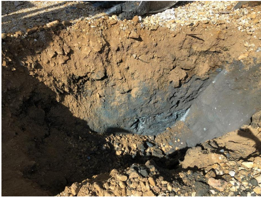
Photo 7: View of the weathered bedrock encountered at 1.7 mbg at test pit TP19-04.
