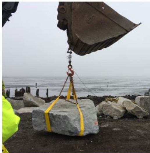
Figure 4: Individual rock weighing using load cell and slings
