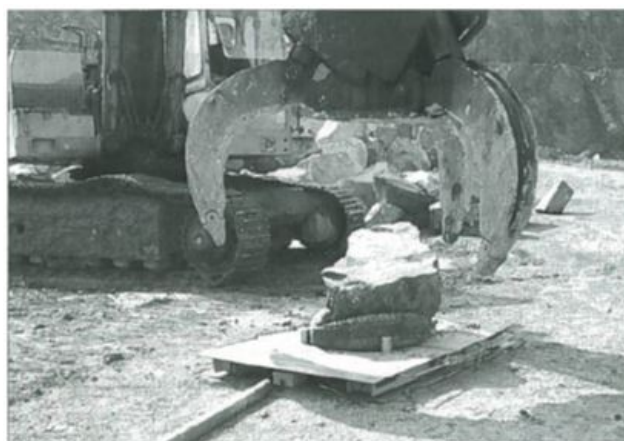
Figure 3: Individual rock weighing at quarry using a floor scale on beams (Ref: CIRIA C683)
