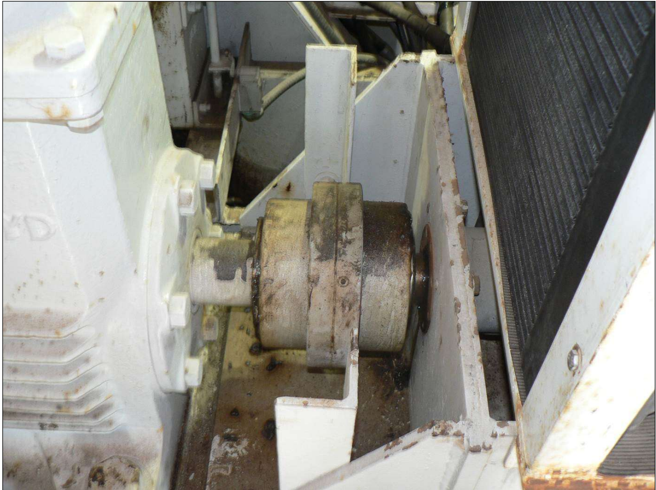
Figure 9: Detail with gearbox at left, oil cooler at right, and coupling on shaft leading to motor at centre.
