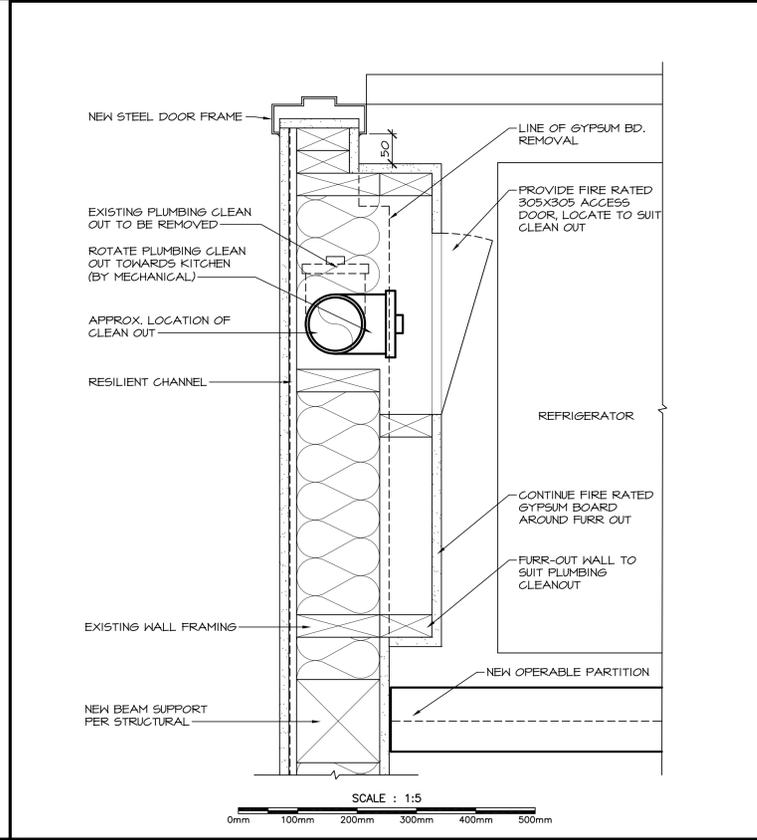
4 PLUMBING CLEAN OUT RELOCATION PLAN DETAIL SCALE 1:5
