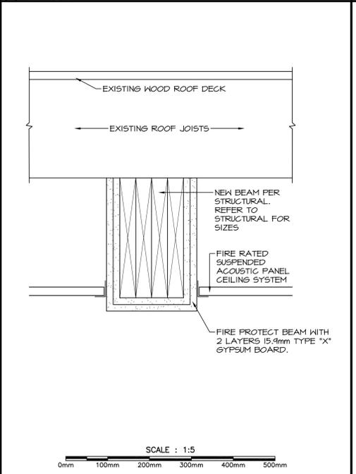
9 TYP. BEAM FIRE PROTECTION DETAIL SCALE 1:5
