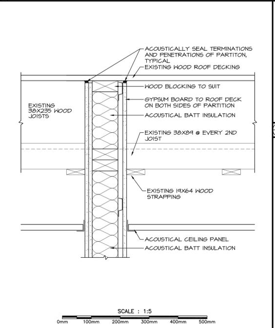
10 PARTITION TO U/S OF DECK DETAIL TYP. SCALE 1:5
