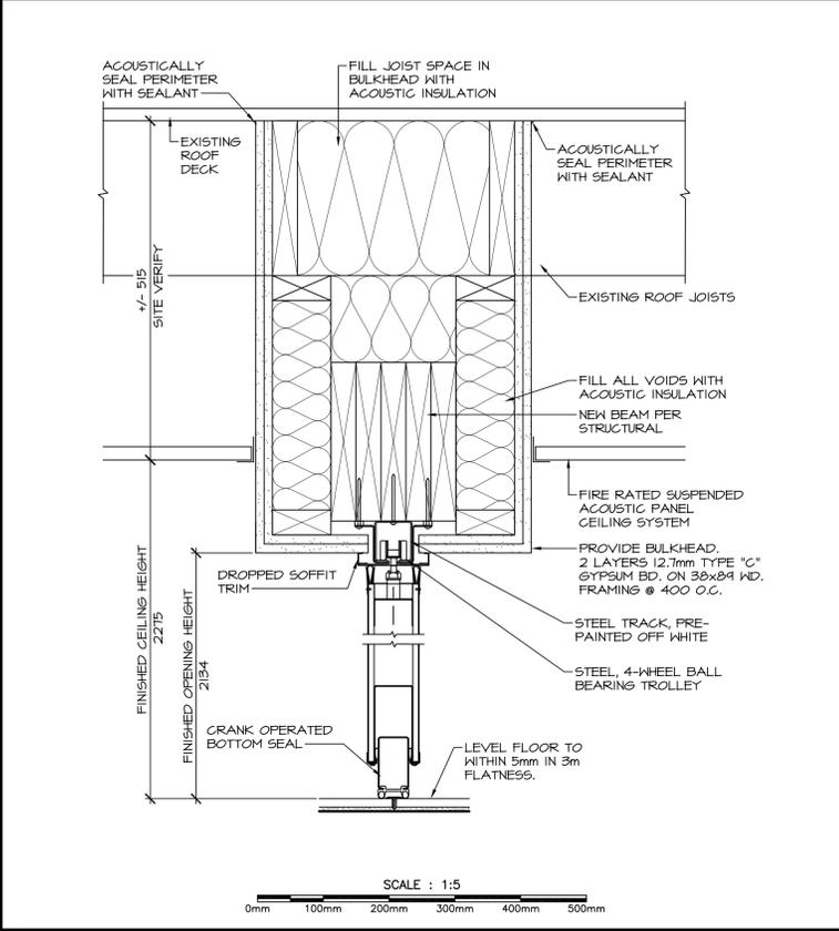
1 FOLDING WALL HEAD AND SILL DETAIL SCALE 1:5
