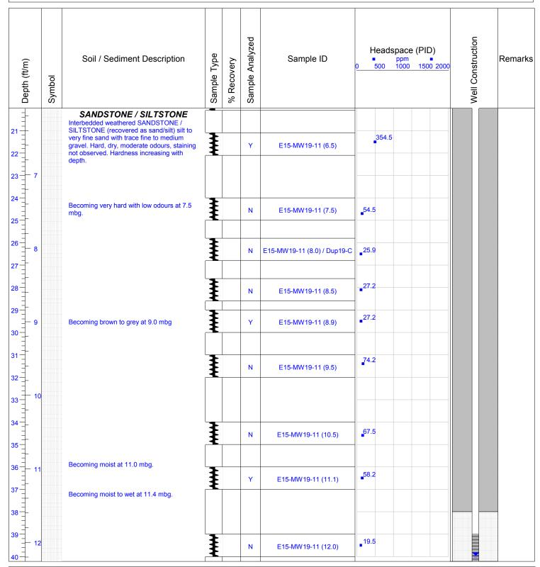
Date of Water Level: January 28, 2019 Water Level (from TOC): 12.08 m Well-Borehole Diameter: 0.20 m Well Casing Diameter: 0.05 m
