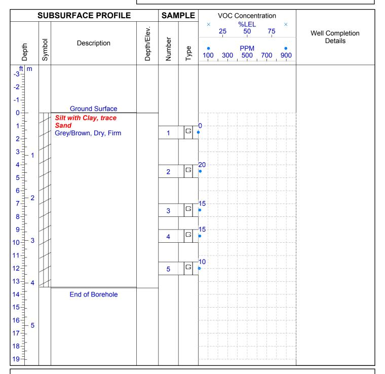
Drilled By: Geotech Well Diameter: 5.08cm (2") Hole Diameter: 11.43cm (4.5")
