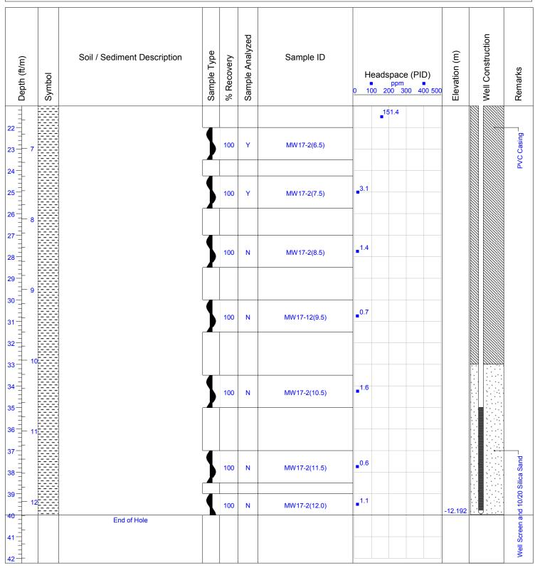
Co-ordinates: n/a Date of Water Level: Water Level (from TOC): Dry Surveyed Water Elevation (m): n/a Well-Borehole Diameter: 0.15 m Well Casing Diameter: 0.05 m Well Casing Material: Schedule 40 PVC Well Screen Slot Size: 0.0025 m
