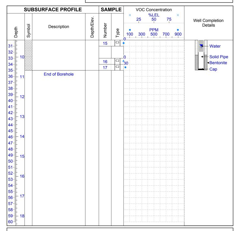
Drilled By: Geotech Well Diameter: 5.08cm (2") Hole Diameter: 10.16cm (4")
