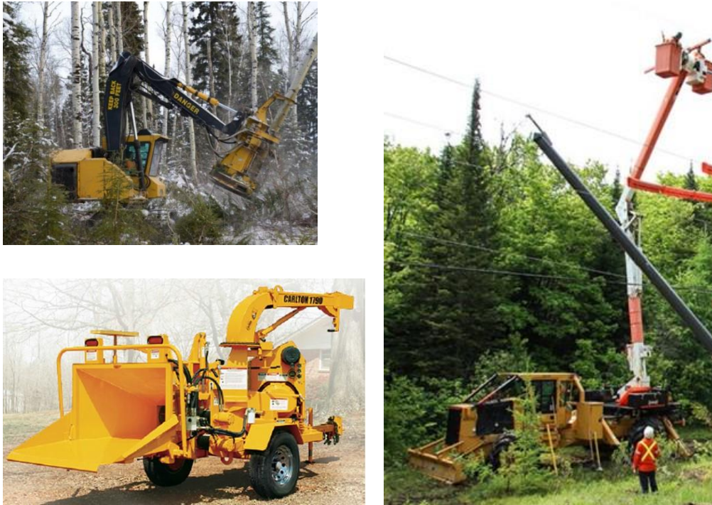
Figure 4. Feller-buncher (top left), Cherry Picker (right) and chipper (bottom)
