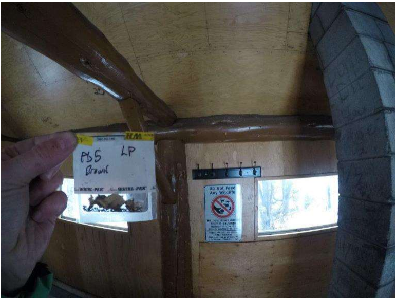
Photograph 9.2-13: Site 9.2 Little Prairie Day Use Area - Akamina Parkway Lead Sample Pb5, 1,500mg/kg.
