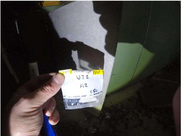
Photograph 7.2-4: Site 7.2 Waterton Townsite Campground Washroom #6 Asbestos Sample A2, Chrysotile, 15%.
