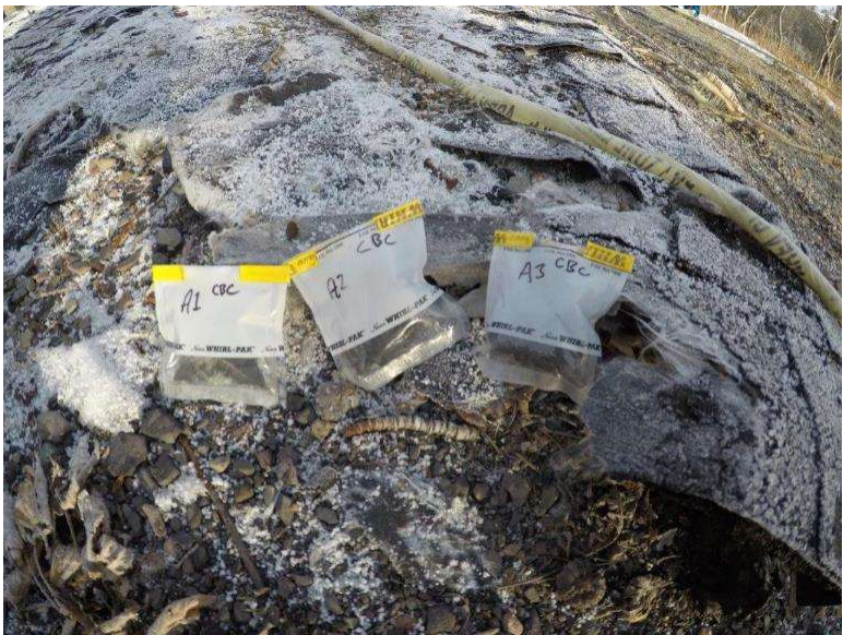
Photograph 2.1-2: Site 2.1 Kitchen Shelter - Crandell Backcountry Asbestos Samples A1-A3, None Detected.
