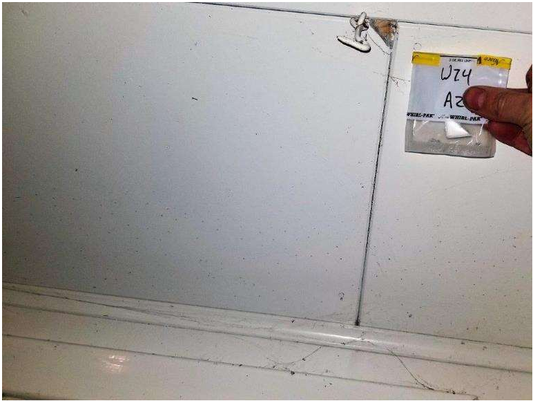
Photograph 7.4-4: Site 7.4 Waterton Townsite Campground Washroom #9 Asbestos Sample A2, Chrysotile, 15%.
