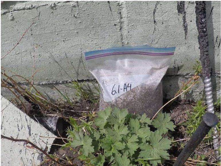
Photograph 6.1-5: Site 6.1 Bear's Hump Seismic Station Asbestos Sample A4, Actinolite, 3%.
