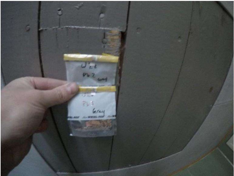
Photograph 7.2-11: Site 7.2 Waterton Townsite Campground Washroom #6 Lead Samples Pb2, 16,000mg/kg and Pb3, 40,000mg/kg.
