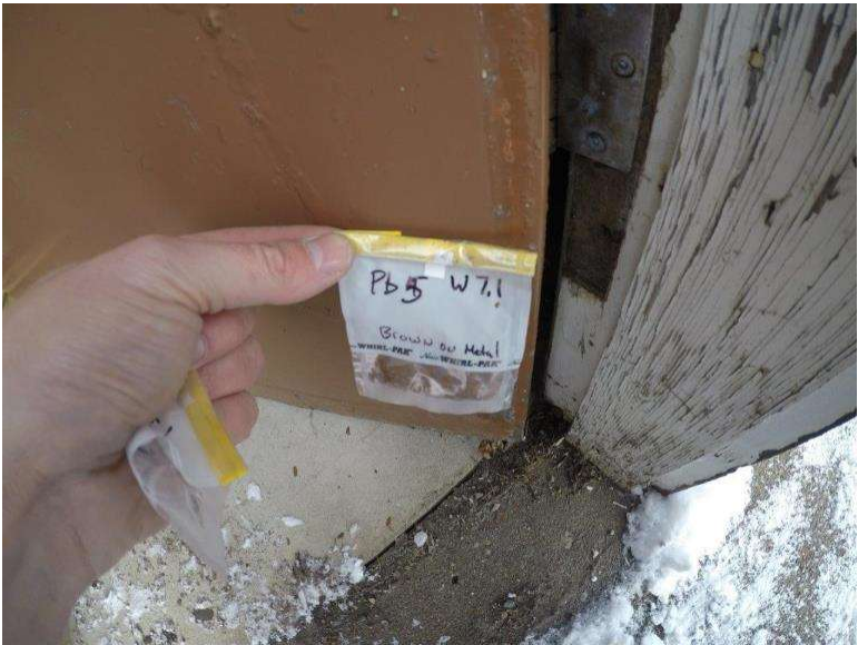
Photograph 7.1-19: Site 7.1 Waterton Townsite Campground Washroom #2 Lead Sample Pb 5, 5,700mg/kg.
