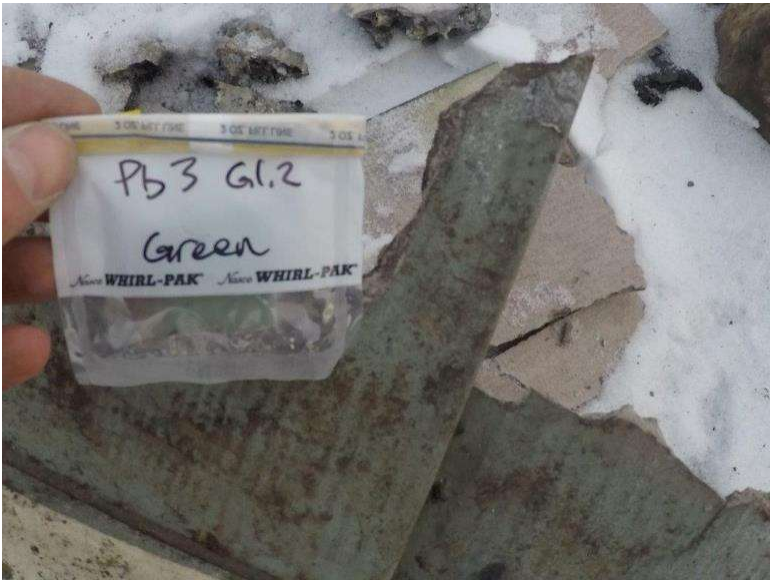
Photograph 1.1-7: Site 1.1 Crandell Campground Generator House Lead Sample Pb3, 14mg/kg.
