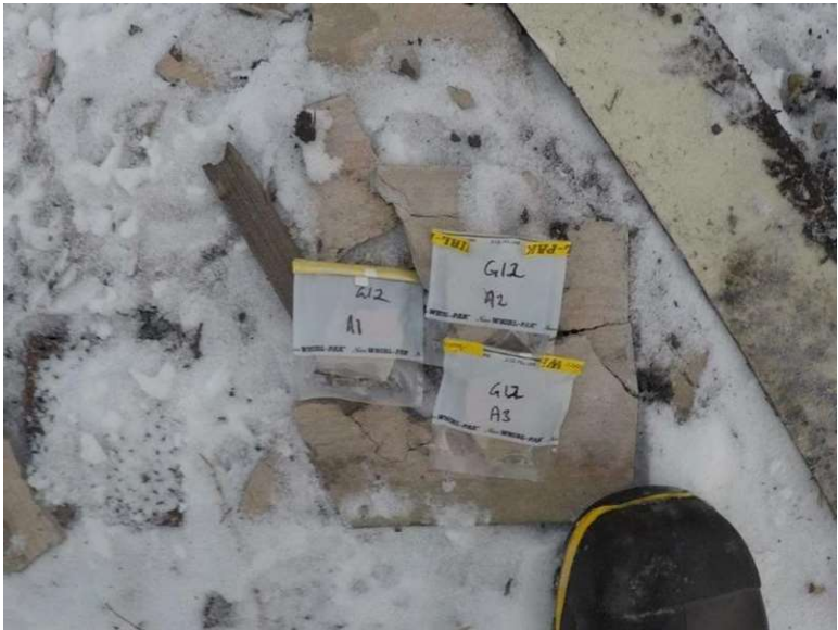
Photograph 1.1-2: Site 1.1 Crandell Campground Generator House Asbestos Samples A1-A3, None Detected.
