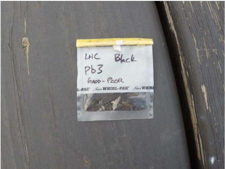
Photograph 8.1-13: Site 8.1 Lost Horse Day Use Area - Red Rock Parkway Lead Paint Sample Pb3, <17mg/kg.
