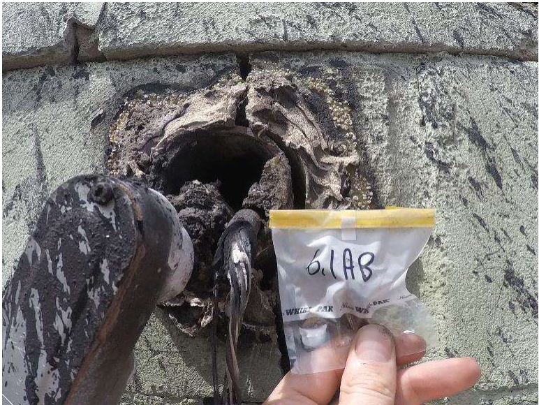
Photograph 6.1-7: Site 6.1 Bear’s Hump Seismic Station Asbestos Sample A8, None Detected.
