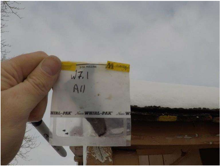
Photograph 7.1-11 Site 7.1 Waterton Townsite Campground Washroom #2 Asbestos Sample A11, None Detected.
