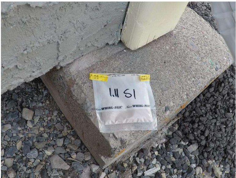
Photograph 1.11-14: Site 1.11 Entrance Kiosk Silica Sample S1, 48.4% SiO 2 .
