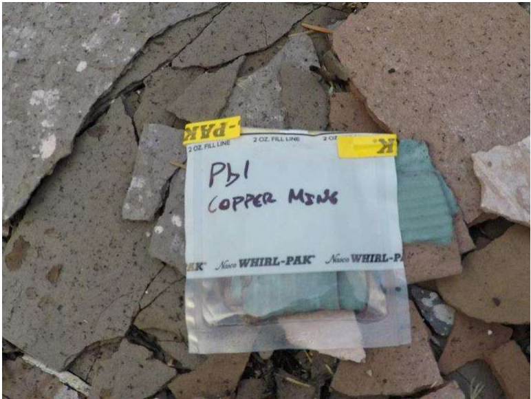
Photograph 8.2-5: Site 8.2 Coppermine Day Use Area - Red Rock Parkway Lead Sample Pb1, <10mg/kg.
