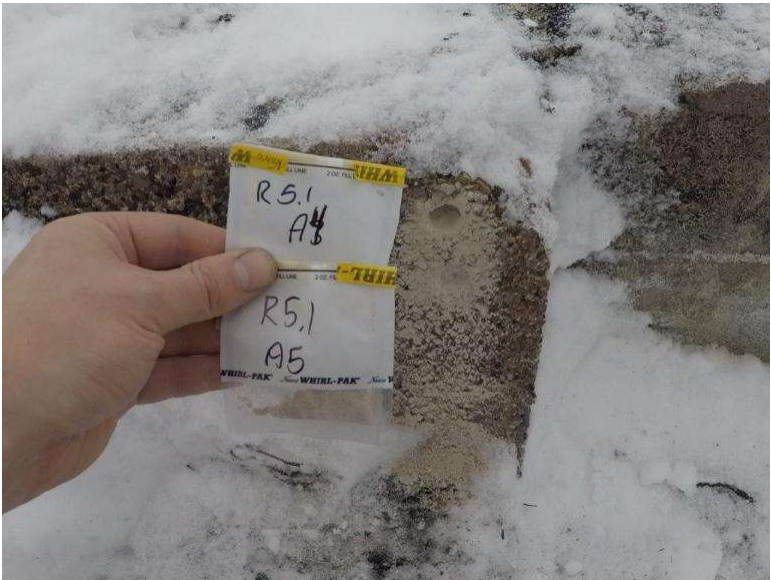
Photograph 5.1-3: Site 5.1 Waterton Golf Course Reservoir Asbestos Samples A4-A5, None Detected.
