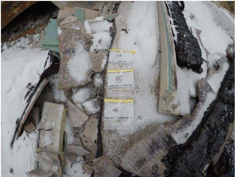
Photograph 9.2-5: Site 9.2 Little Prairie Day Use Area - Akamina Parkway Asbestos Samples A4-A6, None Detected.
