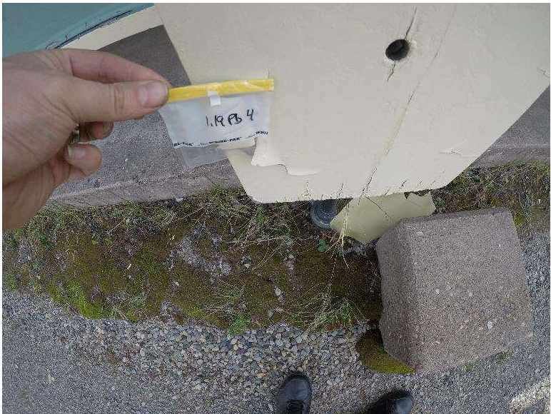
Photograph 1.19-8: Site 1.19 Washroom 4 Lead Sample Pb4, 8,280mg/kg.
