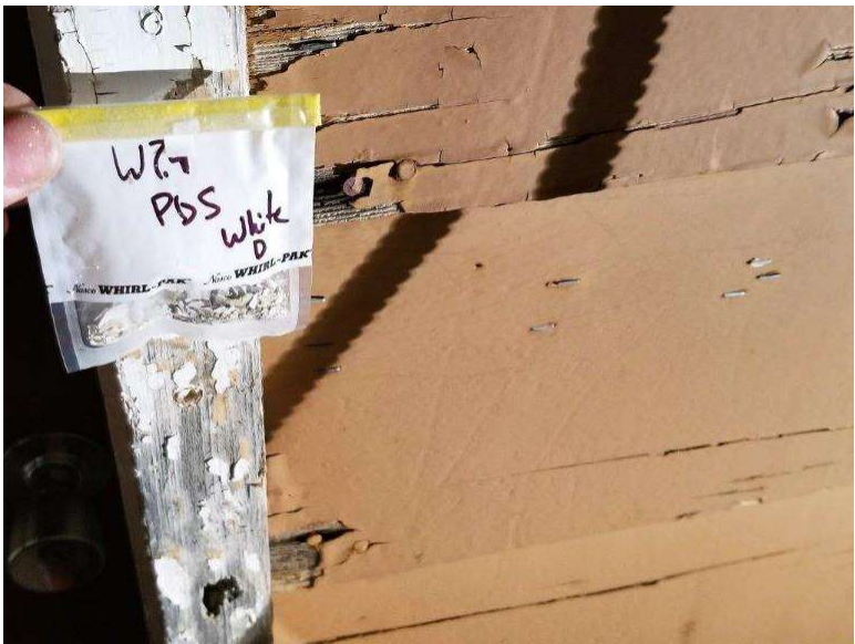
Photograph 7.4-11: Site 7.4 Waterton Townsite Campground Washroom #9 Lead Sample Pb5, 35,000mg/kg.
