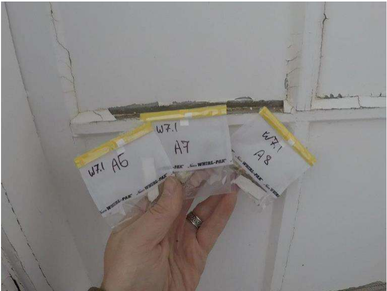
Photograph 7.1-8: Site 7.1 Waterton Townsite Campground Washroom Asbestos Samples A6 – A8, None Detected.
