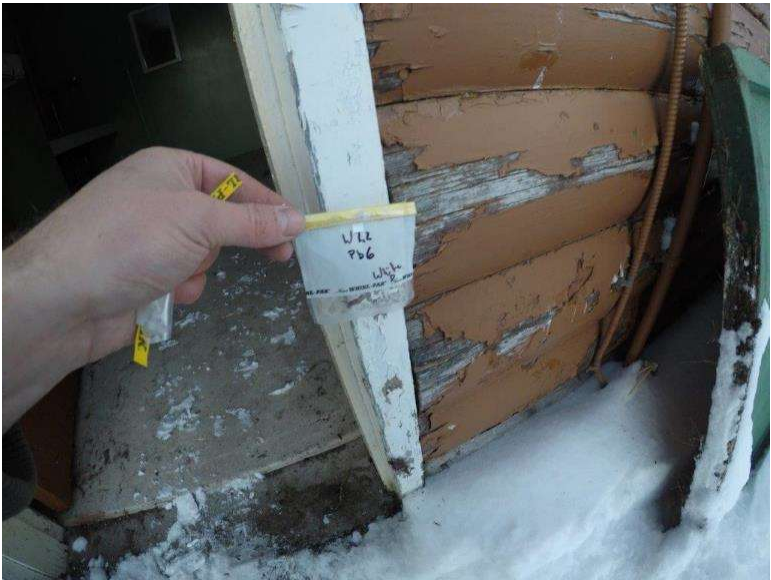
Photograph 7.2-15 Site 7.2 Waterton Townsite Campground Washroom #6 Lead Sample Pb6, 110,000mg/kg.
