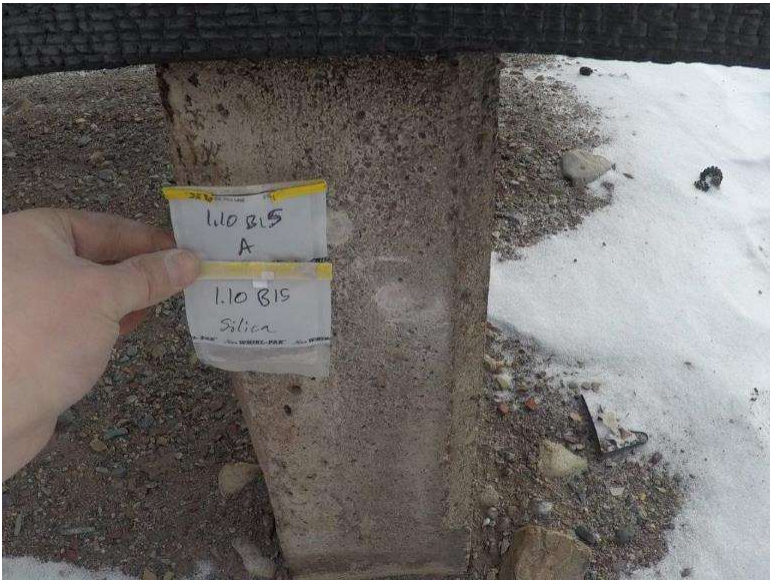
Photograph 1.10-7: Site 1.10 Crandell Campground 129 Campsites (Loop B Campsite 13) Asbestos Sample A2, None Detected. Silica Sample S2 49.94% SiO 2 .
