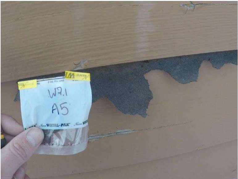
Photograph 7.1-7: Site 7.1 Waterton Townsite Campground Washroom Asbestos Sample A5, None Detected.
