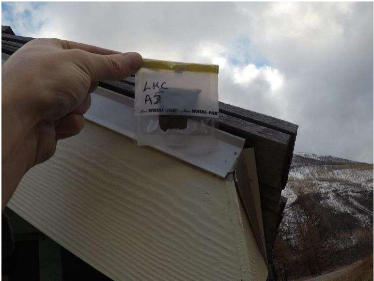
Photograph 8.1-9: Site 8.1 Lost Horse Day Use Area - Red Rock Parkway Asbestos Sample A5, None Detected.
