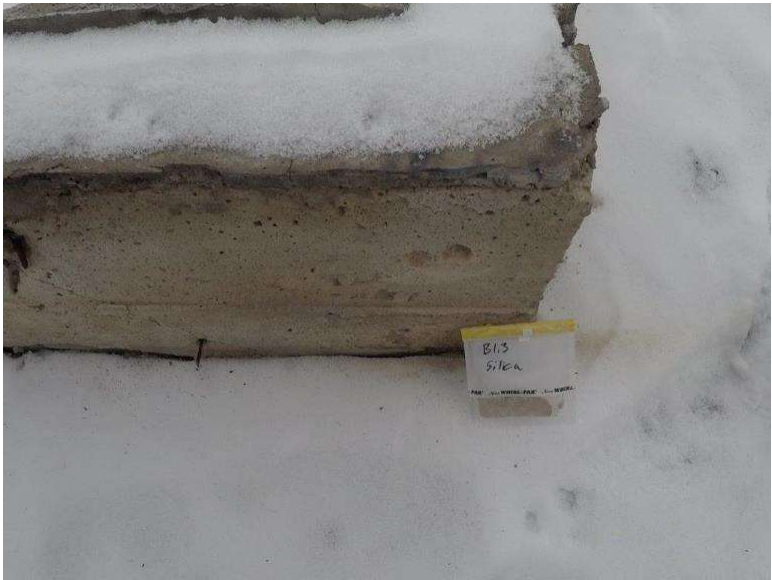
Photograph 1.4-5: Site 1.4 Crandell Campground Washroom 2 Silica Sample 1.3-S1, 48.70% SiO 2 .
