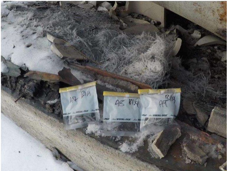
Photograph 1.3-4: Site 1.3 Crandell Campground Washroom 1 Asbestos Samples 1.4-A7 to 1.4-A9, None Detected.
