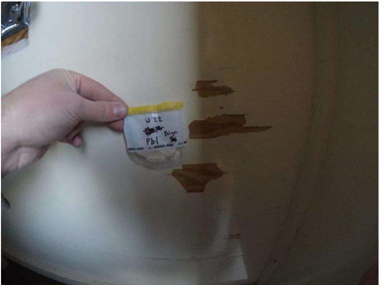
Photograph 7.9-10: Site 7.2 Waterton Townsite Campground Washroom #6 Lead Sample Pb1, 2,000mg/kg.
