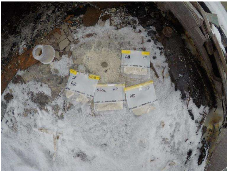
Photograph 9.2-7: Site 9.2 Little Prairie Day Use Area - Akamina Parkway Asbestos Samples A10-A12, None Detected. Silica Sample S1, 76.21% SiO 2 .
