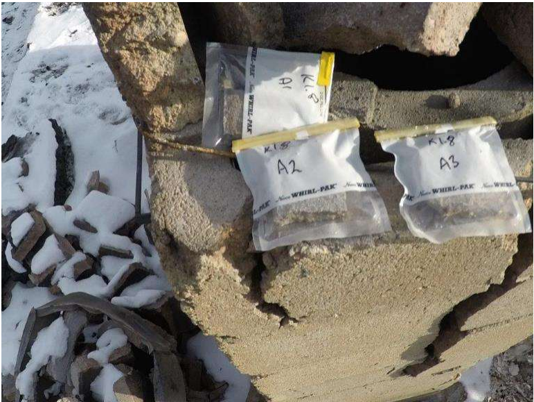
Photograph 1.8-2: Site 1.8 Crandell Campground Kitchen Shelter 4 Asbestos Samples A1-A3, None Detected.
