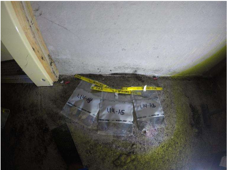
Photograph 1.14-3: Site 1.14 Solar Building #3 Asbestos Sample A4, A5, A6, None Detected.
