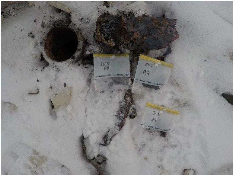
Photograph 1.3-4: Site 1.3 Crandell Campground Washroom 2 Asbestos Samples 1.3-A7 to 1.3-A9, None Detected.
