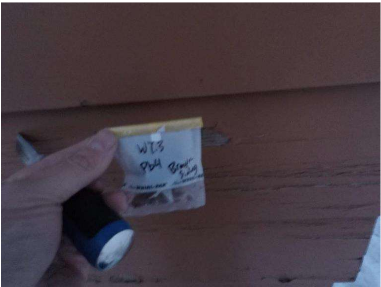
Photograph 7.3-9 Site 7.3 Waterton Townsite Campground Washroom #8 Lead Sample Pb4, 88,000mg/kg.
