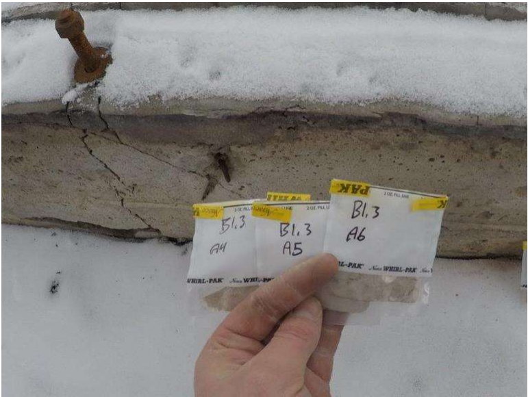
Photograph 1.4-3: Site 1.4 Crandell Campground Washroom 2 Asbestos Samples 1.3-A4 to 1.3-A6, None Detected.
