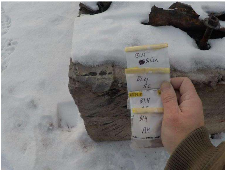
Photograph 1.3-3: Site 1.3 Crandell Campground Washroom 1 Asbestos Samples 1.4-A4 to 1.4-A6, None Detected. Silica Sample 1.4-S1, 50.14% SiO 2 .
