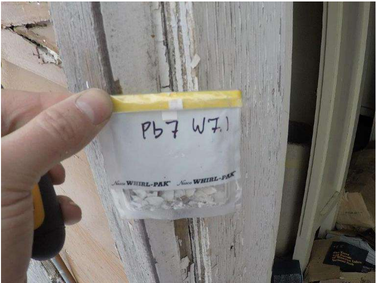
Photograph 7.1-21: Site 7.1 Waterton Townsite Campground Washroom #2 Lead Sample Pb7, 73,000mg/kg.
