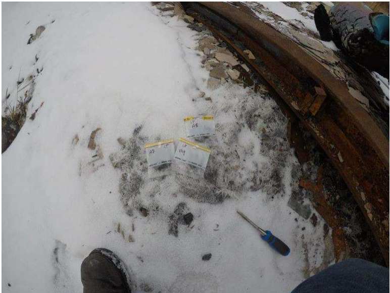
Photograph 9.2-6: Site 9.2 Little Prairie Day Use Area - Akamina Parkway Asbestos Samples A7-A9, None Detected.
