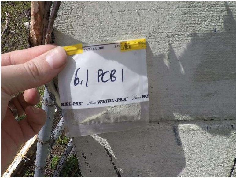
Photograph 6.1-13: Site 6.1 Bear’s Hump Seismic Station PCB Sample PCB1, <0.02mg/kg.
