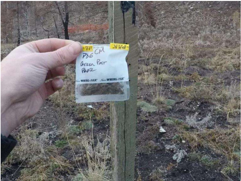
Photograph 8.2-9: Site 8.2 Coppermine Day Use Area - Red Rock Parkway Lead Sample Pb6, 4,800mg/kg.
