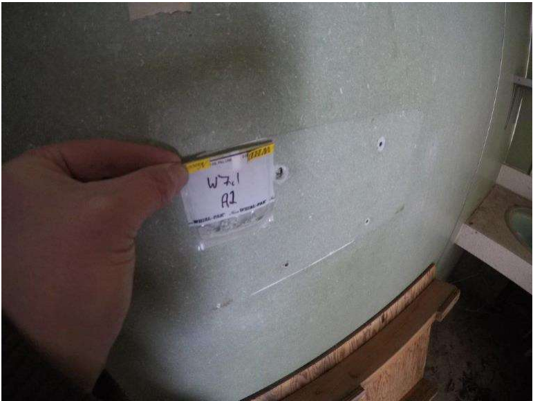
Photograph 7.1-3: Site 7.1 Waterton Townsite Campground Washroom #2 Asbestos Sample A1, Chrysotile, 12%.
