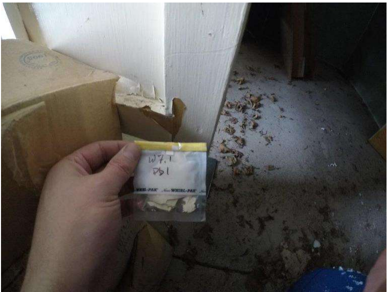
Photograph 7.1-16: Site 7.1 Waterton Townsite Campground Washroom #2 Lead Sample Pb1, 2,900mg/kg.
