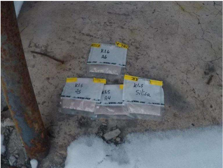
Photograph 1.5-3: Site 1.5 Crandell Campground Kitchen Shelter 1 Asbestos Samples A4-A6, None Detected. Silica Sample S1 47.35% SiO 2 .
