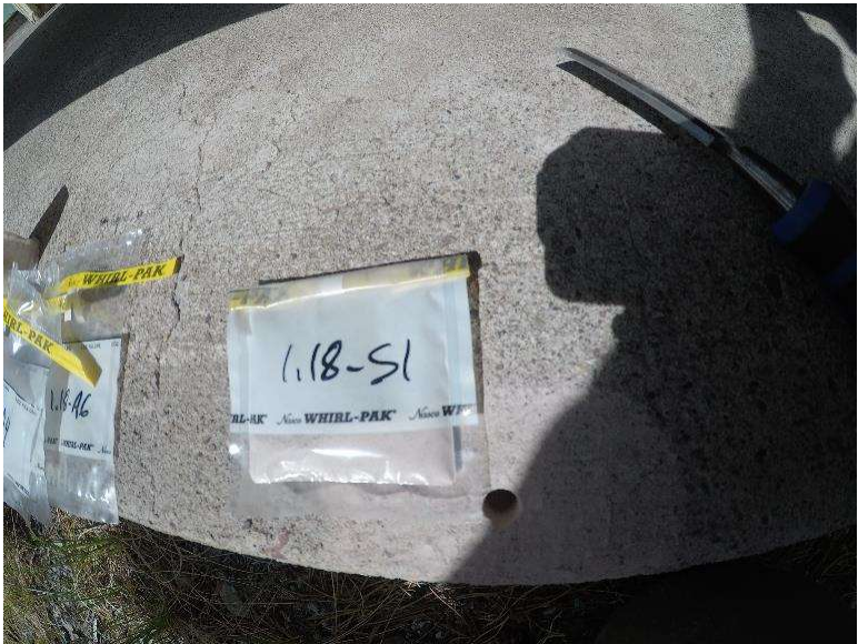
Photograph 1.18-10: Site 1.18 Washroom 3 Silica Sample S1, 52.8% SiO 2 .
