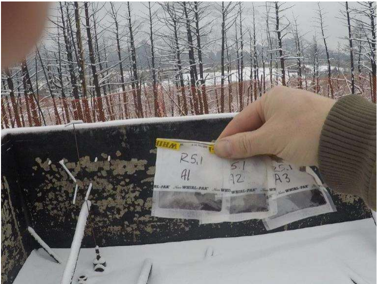
Photograph 5.1-2: Site 5.1 Waterton Golf Course Reservoir Asbestos Samples A1-A3, None Detected.
