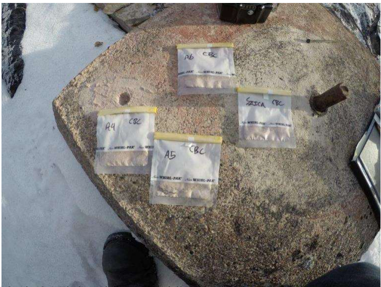
Photograph 2.1-3: Site 2.1 Kitchen Shelter - Crandell Backcountry Asbestos Samples A4-A6, None Detected. Silica Sample S1, 51.49% SiO 2 .
