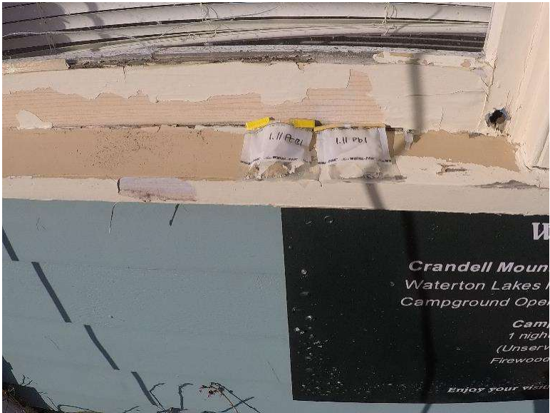
Photograph 1.11-8: Site 1.11 Entrance Kiosk Lead Sample Pb1, 11,400mg/kg. PCB Sample PCB1, <0.02mg/kg
