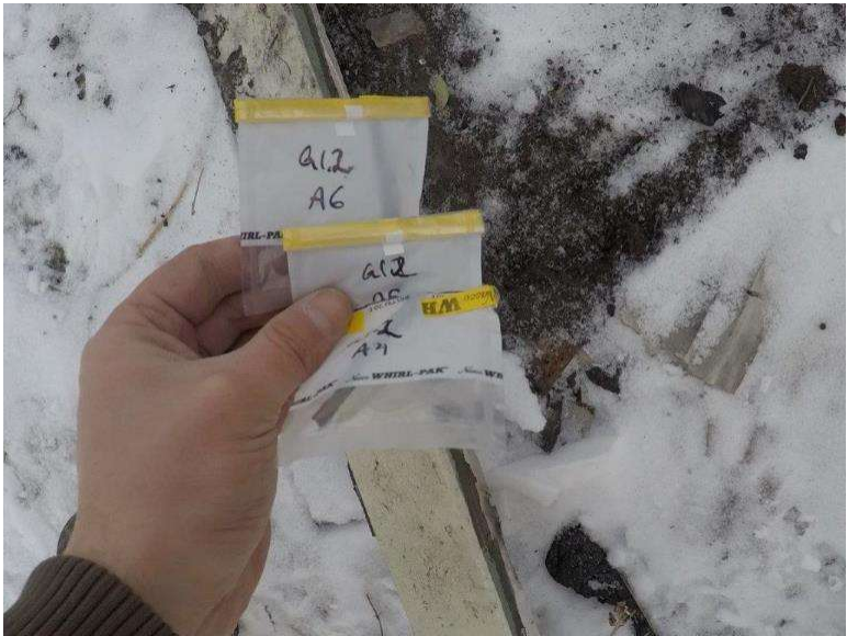
Photograph 1.1-3: Site 1.1 Crandell Campground Generator House Asbestos Samples A4-A6, None Detected.
