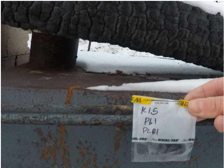
Photograph 1.5-5: Site 1.5 Crandell Campground Kitchen Shelter 1 Lead Sample Pb1, <10mg/kg, and Pb2, 60mg/kg..
