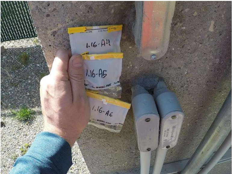
Photograph 1.16-6: Site 1.16 Solar Building #5 Asbestos Sample A4, A5, A6, None Detected.
