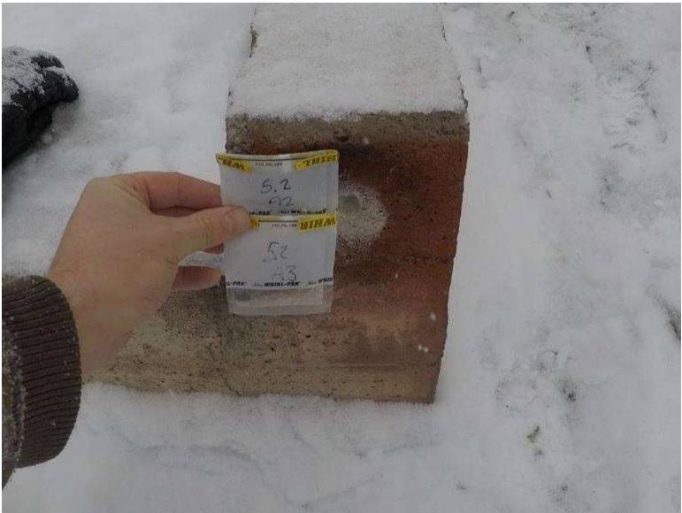
Photograph 5.2-2: Site 5.2 Waterton Golf Course Lightning Shelter Shed Asbestos Samples A2-A3, None Detected.
