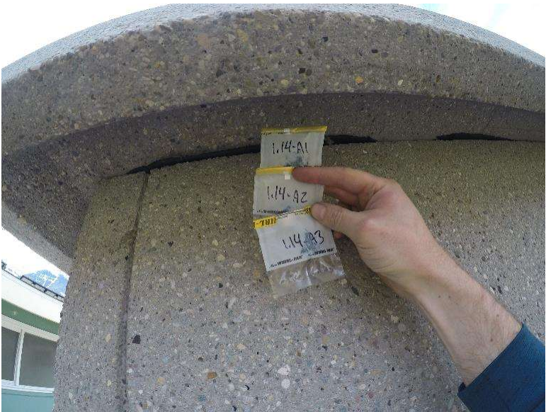
Photograph 1.14-2: Site 1.14 Solar Building #3 Asbestos Sample A1, A2, A3, None Detected.
