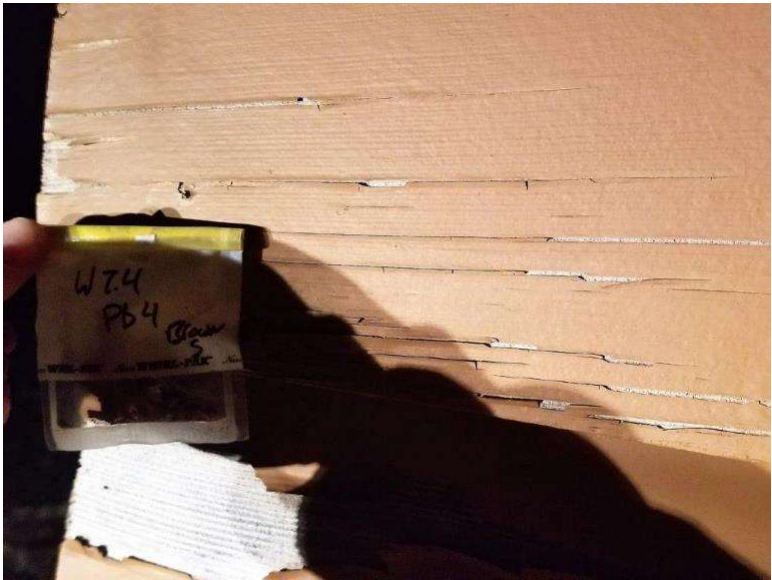
Photograph 7.4-10: Site 7.4 Waterton Townsite Campground Washroom #9 Lead Sample Pb4, 110,000mg/kg.
