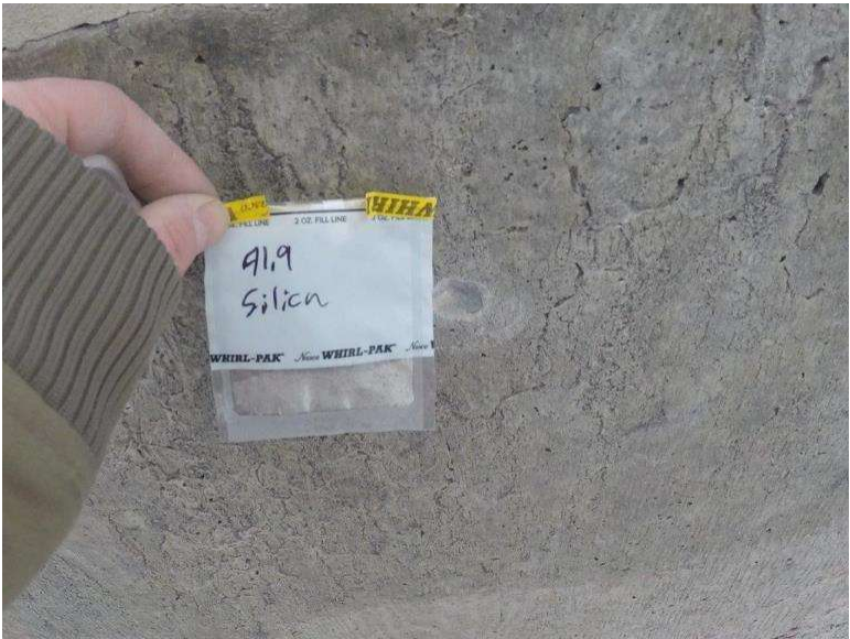
Photograph 1.9-10: - Site 1.9 Crandell Campground Interpretive Theatre Silica Sample S1 49.72% SiO 2 .
