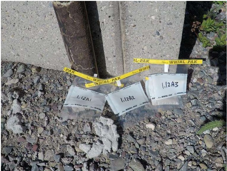
Photograph 1.11-2: Site 1.12 Solar Building #1 Asbestos Sample A1, A2, A3, None Detected.
