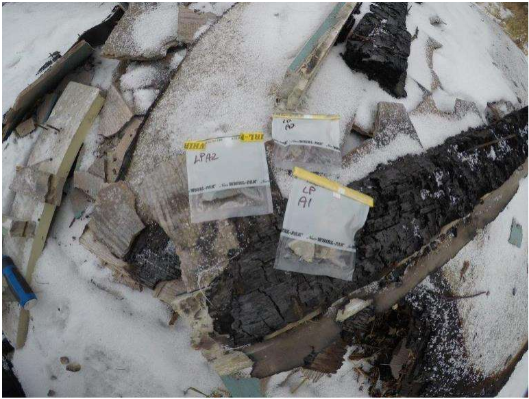
Photograph 9.2-4: Site 9.2 Little Prairie Day Use Area - Akamina Parkway Asbestos Samples A1-A3, None Detected.
