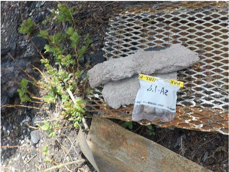
Photograph 6.1-3: Site 6.1 Bear's Hump Seismic Station Asbestos Sample A2, None Detected.
