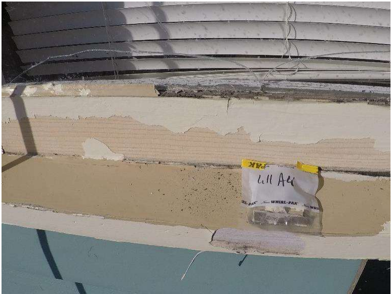
Photograph 1.11-5: Site 1.11 Entrance Kiosk Asbestos Sample A4, None Detected.
