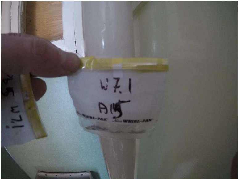
Photograph 7.1-15: Site 7.1 Waterton Townsite Campground Washroom #2 Asbestos Sample A15, None Detected.
