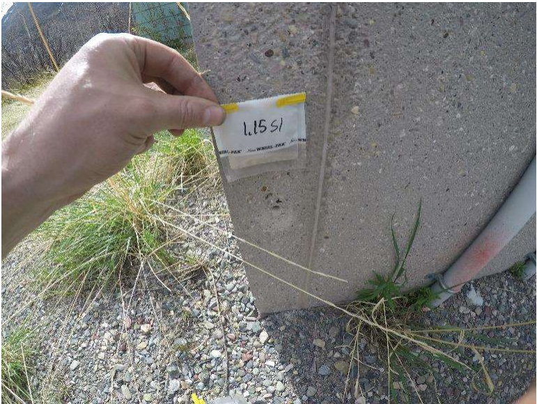
Photograph 1.15-5: Site 1.15 Solar Building #4 Silica Sample S1, 55.4% SiO 2 .
