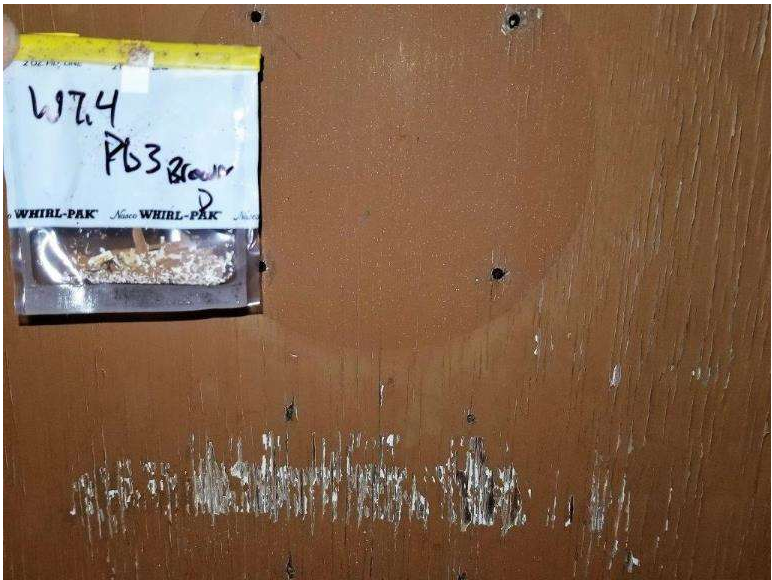
Photograph 7.4-9: Site 7.4 Waterton Townsite Campground Washroom #9 Lead Sample Pb3, 110,000mg/kg.
