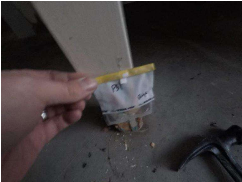
Photograph 7.3-6: Site 7.3 Waterton Townsite Campground Washroom #8 Lead Sample Pb1, 15,000mg/kg.
