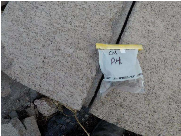
Photograph 8.2-4 Site 8.2 Coppermine Day Use Area - Red Rock Parkway Asbestos Sample A4, None Detected.
