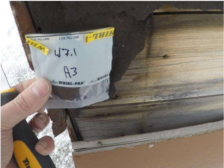
Photograph 7.1-5: Site 7.1 Waterton Townsite Campground Washroom Asbestos Sample A3, None Detected.
