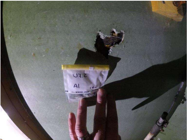
Photograph 7.2-3: Site 7.2 Waterton Townsite Campground Washroom #6 Asbestos Sample A1, Chrysotile, 15%.
