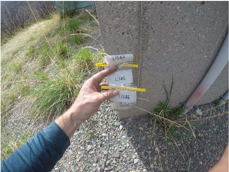
Photograph 1.15-3: Site 1.15 Solar Building #4 Asbestos Sample A4, A5, A6, None Detected.
