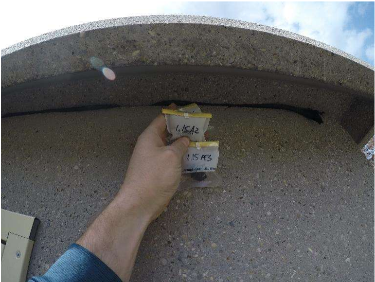
Photograph 1.15-2: Site 1.15 Solar Building #4 Asbestos Sample A1, A2, A3, None Detected.
