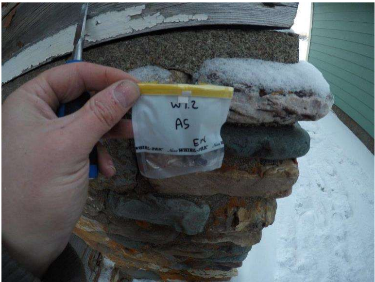
Photograph 7.2-7: Site 7.2 Waterton Townsite Campground Washroom #6 Asbestos Sample A5, None Detected.
