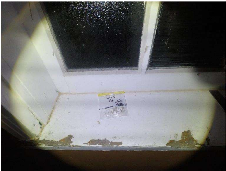
Photograph 7.3-11: Site 7.3 Waterton Townsite Campground Washroom #8 Lead Sample Pb6, 1,200mg/kg.
