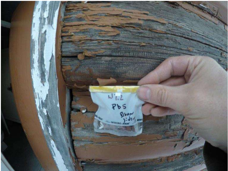
Photograph 7.2-13: Site 7.2 Waterton Townsite Campground Washroom #6 Lead Sample Pb 5, 4,800mg/kg.
