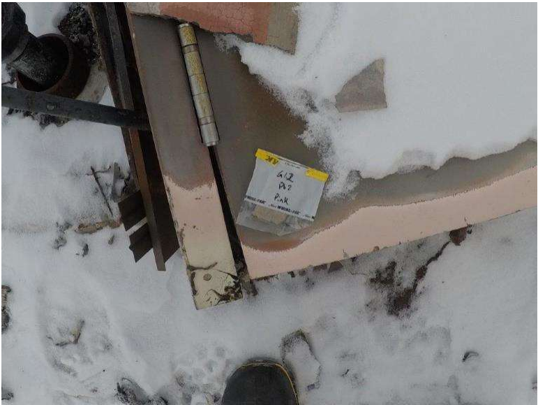
Photograph 1.1-6: Site 1.1 Crandell Campground Generator House Lead Sample Pb2, 300mg/kg.
