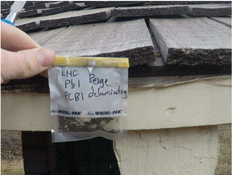
Photograph 8.1-11: Site 8.1 Lost Horse Day Use Area - Red Rock Parkway Lead Sample Pb1, 800mg/kg, PCB Sample PCB1, 0.43mg/kg.
