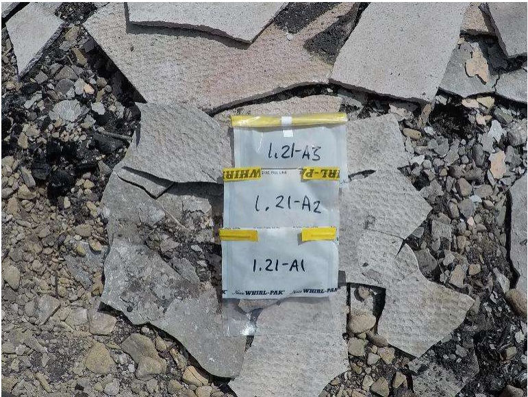
Photograph 1.21-2: Site 1.17 Host Campground Asbestos Sample A1, A2, A3, None Detected.
