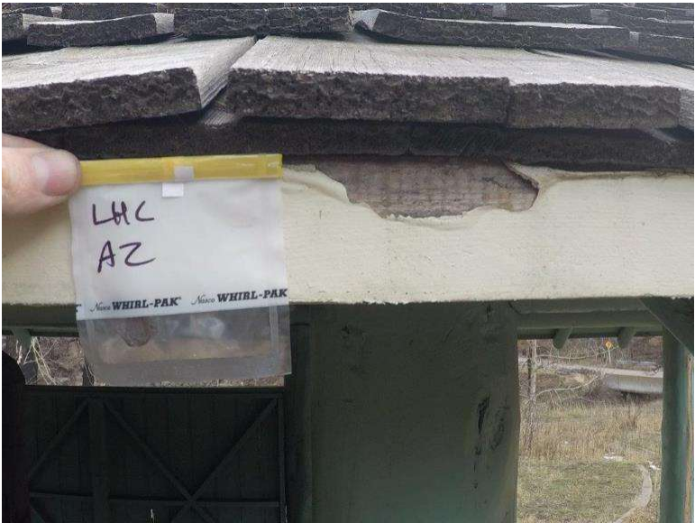
Photograph 8.1-6: Site 8.1 Lost Horse Day Use Area - Red Rock Parkway Asbestos Sample A2, None Detected.
