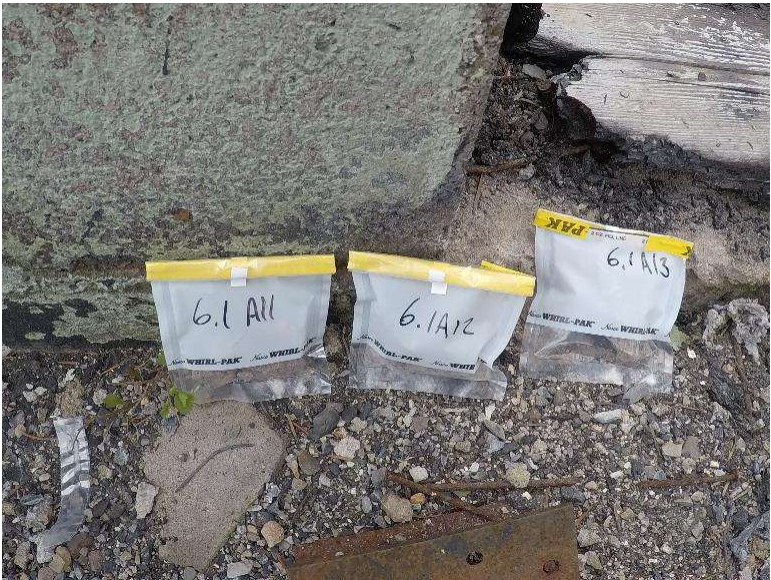
Photograph 6.1-10: Site 6.1 Bear’s Hump Seismic Station Asbestos Sample A11 & A12, None Detected, A13, Chrysotile, <1%.
