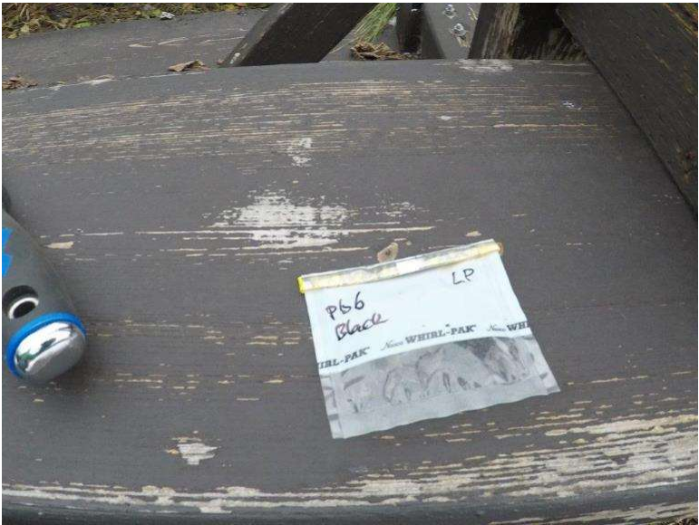
Photograph 9.2-14: Site 9.2 Little Prairie Day Use Area - Akamina Parkway Lead Sample Pb6, <28mg/kg.
