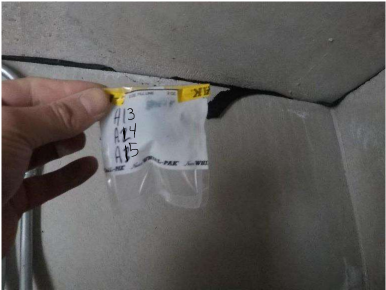
Photograph 1.12-2: Site 1.12 Solar Building #1 Asbestos Samples 1.4-A13, 1.4-A14, 1.4-A15, None Detected.
