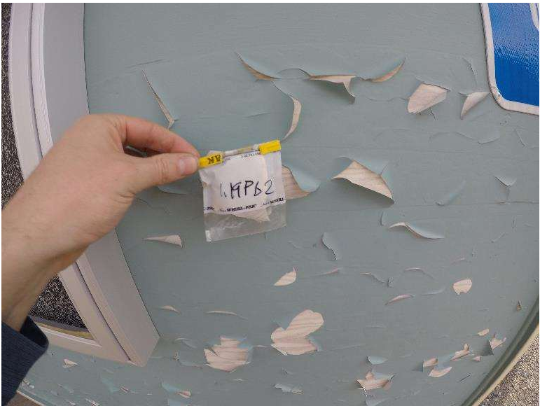
Photograph 1.19-6: Site 1.19 Washroom 4 Lead Sample Pb2, 9,140mg/kg.
