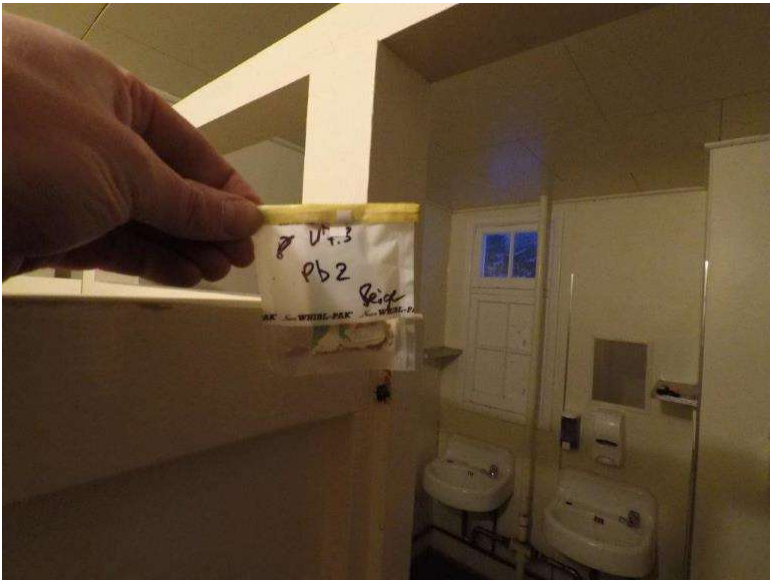
Photograph 7.3-7: Site 7.3 Waterton Townsite Campground Washroom #8 Lead Sample Pb2, 23,000mg/kg.
