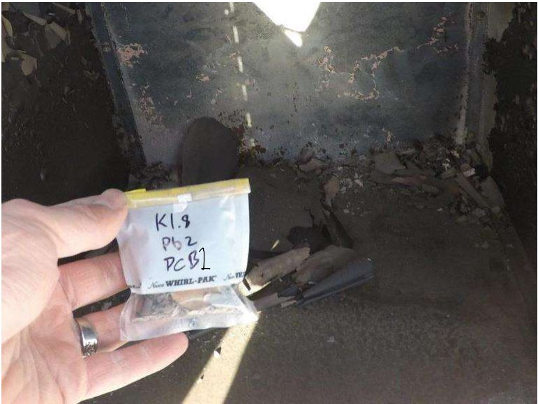
Photograph 1.8-6: Site 1.8 Crandell Campground Kitchen Shelter 4 Lead Sample Pb2, 56mg/kg. PCB Sample PCB1, <0.02mg/kg.
