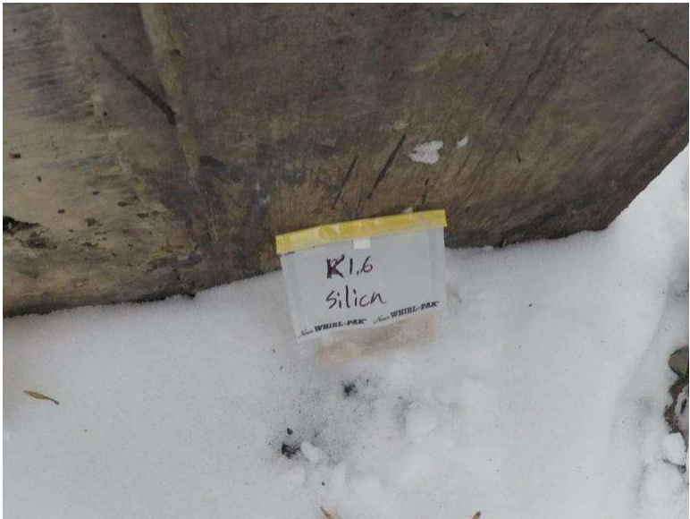
Photograph 1.6-6: Site 1.6 Crandell Campground Kitchen Shelter 2 Silica Sample S1 48.22% SiO 2 .
