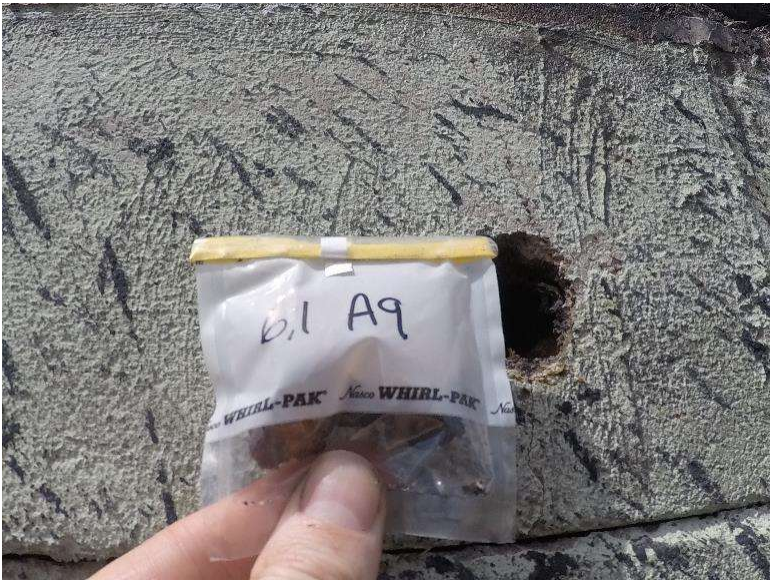
Photograph 6.1-8: Site 6.1 Bear’s Hump Seismic Station Asbestos Sample A9, Chrysotile, <1%.
