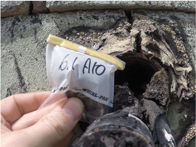
Photograph 6.1-9: Site 6.1 Bear’s Hump Seismic Station Asbestos Sample A10, Chrysotile, <1%.
