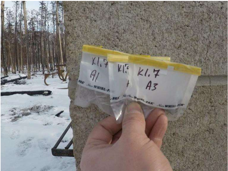
Photograph 1.7-2: Site 1.7 Crandell Campground Kitchen Shelter 3 Asbestos Samples A1-A3, None Detected.
