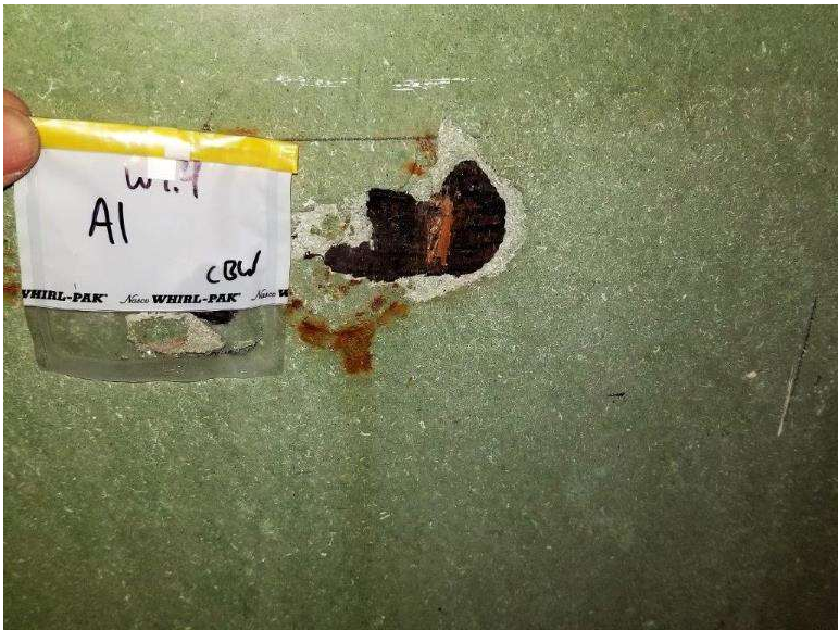
Photograph 7.4-3 Site 7.4 Waterton Townsite Campground Washroom #9 Asbestos Sample A1, Chrysotile, 15%.
