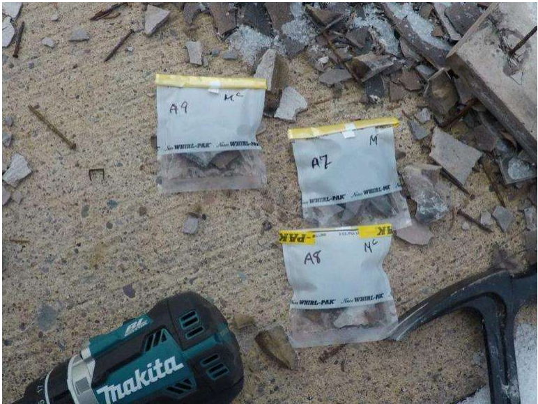
Photograph 9.1-3: Site 9.1 McNealy's Day Use Area - Akamina Parkway Asbestos Samples A7-A9, None Detected.
