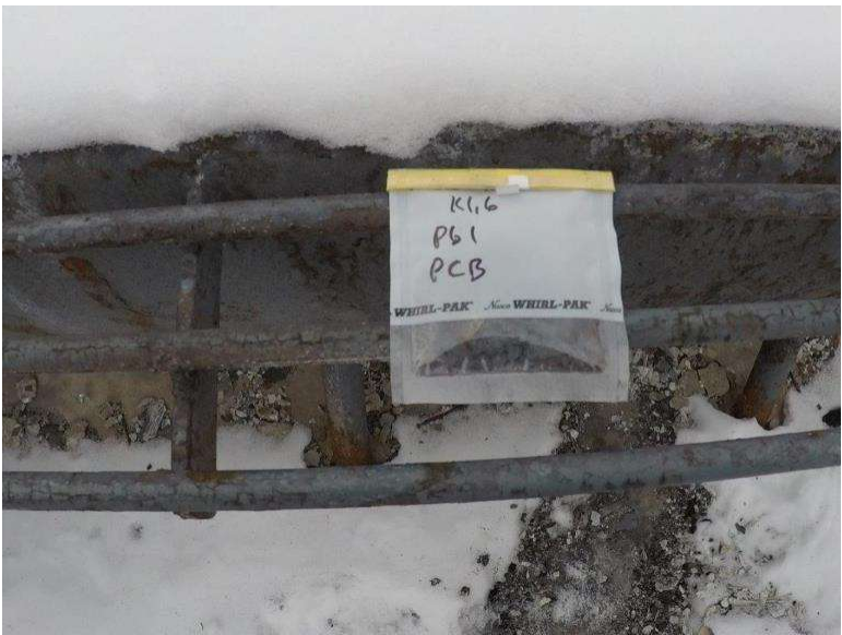
Photograph 1.6-7: Site 1.6 Crandell Campground Kitchen Shelter 2 Lead Sample Pb1, 10mg/kg. PCB sample PCB1, <0.2mg/kg.
