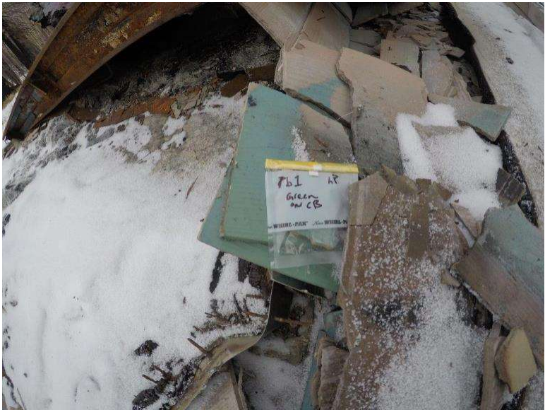
Photograph 9.2-9: Site 9.2 Little Prairie Day Use Area - Akamina Parkway Lead Sample Pb1, <10mg/kg.
