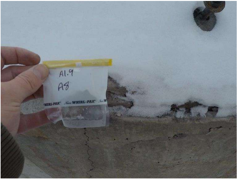
Photograph 1.9-8: Site 1.9 Crandell Campground Interpretive Theatre Asbestos Sample A8, None Detected.
