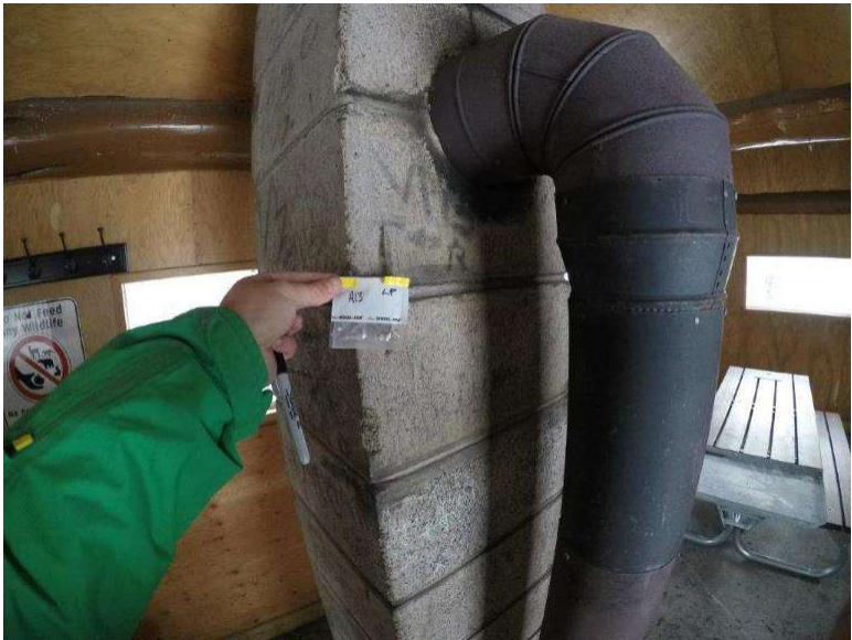
Photograph 9.2-8 Site 9.2 Little Prairie Day Use Area - Akamina Parkway Asbestos Sample A13, None Detected.
