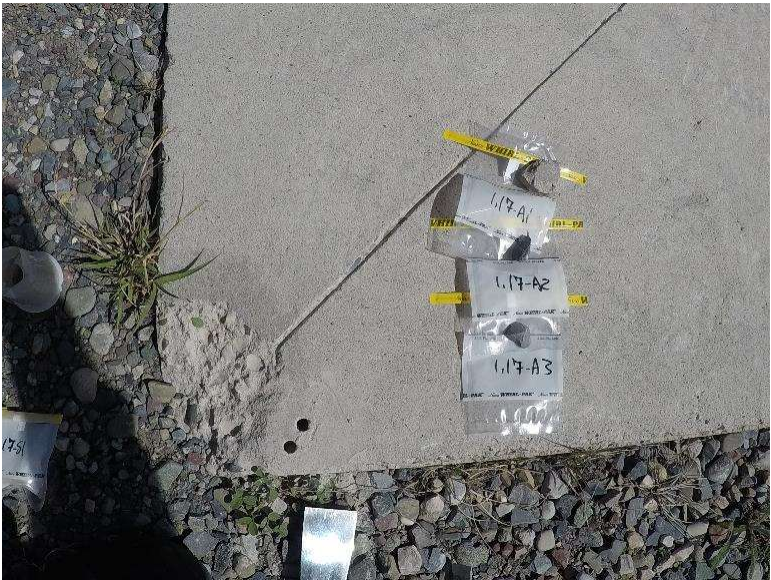
Photograph 1.17-2: Site 1.17 Sani-Dump Station Asbestos Sample A1, A2, A3, None Detected.
