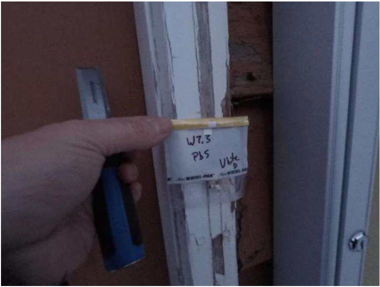
Photograph 7.3-10: Site 7.3 Waterton Townsite Campground Washroom #8 Lead Sample Pb5, 1,800mg/kg.
