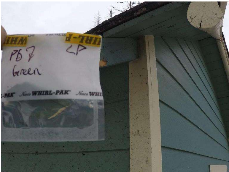
Photograph 9.2-15: Site 9.2 Little Prairie Day Use Area - Akamina Parkway Lead Sample Pb7, 660mg/kg.
