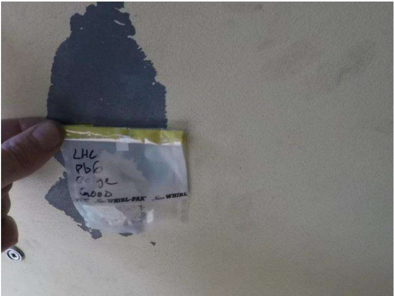
Photograph 8.1-16: Site 8.1 Lost Horse Day Use Area - Red Rock Parkway Lead Sample Pb6, <18mg/kg.
