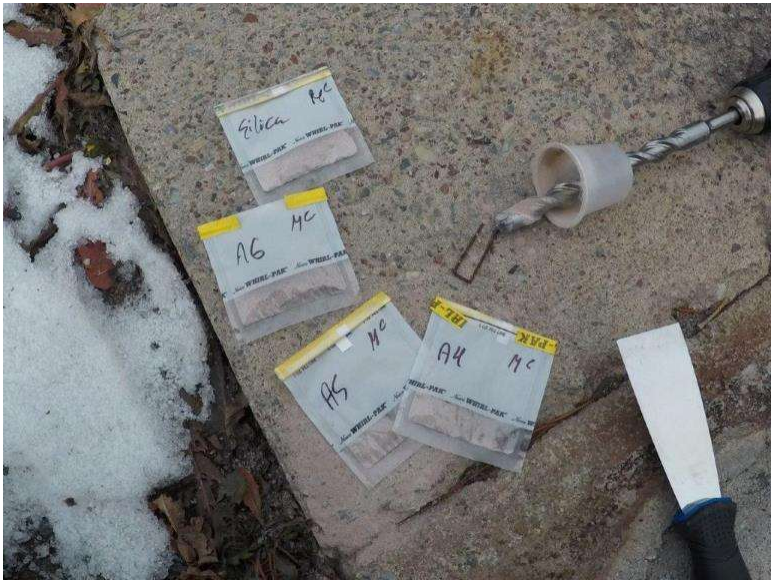
Photograph 9.1-2: Site 9.1 McNealy's Day Use Area - Akamina Parkway Asbestos Samples A4-A6, None Detected. Silica sample S1, 49.67% SiO 2 .
