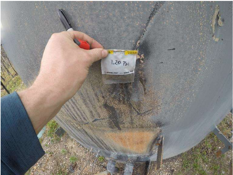
Photograph 1.20-1: Site 1.20 Water Tower Lead Sample Pb1, 6,890mg/kg.
