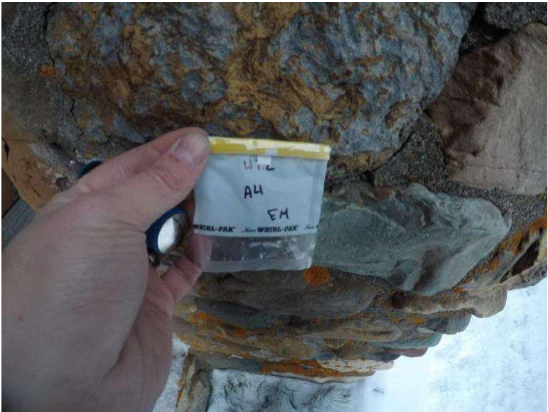
Photograph 7.2-6: Site 7.2 Waterton Townsite Campground Washroom #6 Asbestos Sample A4, None Detected.
