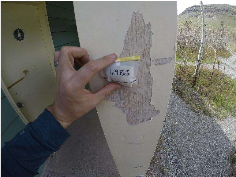
Photograph 1.19-7: Site 1.19 Washroom 4 Lead Sample Pb3, 9,360mg/kg.
