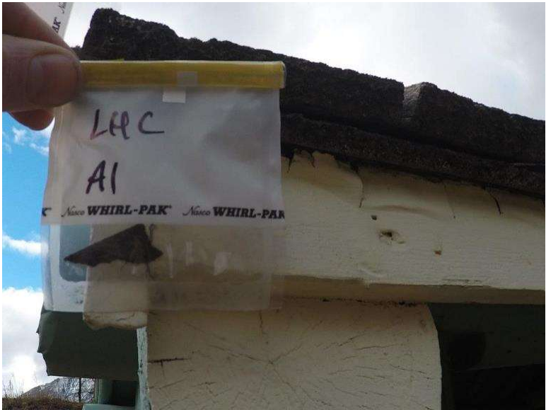
Photograph 8.1-5: Site 8.1 Lost Horse Day Use Area - Red Rock Parkway Asbestos Sample A1, None Detected.
