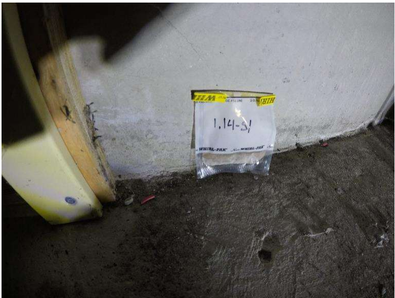
Photograph 1.14-4: Site 1.14 Solar Building #3 Silica Sample S1, 52.2% SiO 2 .
