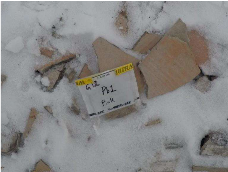
Photograph 1.1-5: Site 1.1 Crandell Campground Generator House Lead Sample Pb1, 11mg/kg.
