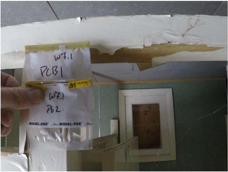
Photograph 7.1-17 Site 7.1 Waterton Townsite Campground Washroom #2 Lead Sample Pb2, 2,900mg/kg. PCB Sample PCB1, 0.21mg/kg
