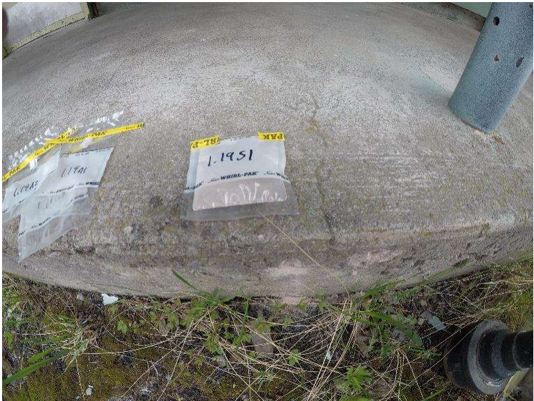
Photograph 1.19-10: Site 1.19 Washroom 4 Silica Sample S1, 52.8% SiO 2 .
