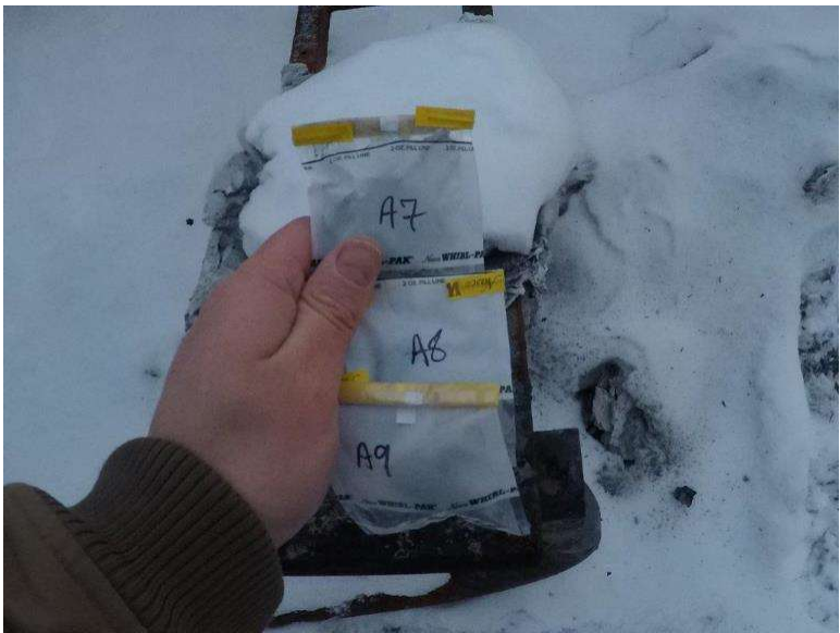
Photograph 1.5-4: Site 1.5 Crandell Campground Kitchen Shelter 1 Asbestos Samples A7-A9, None Detected.
