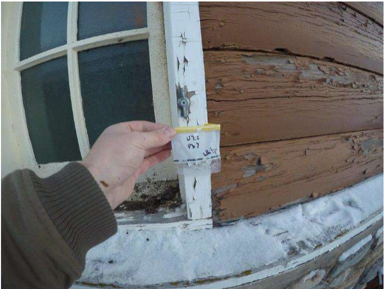
Photograph 7.2-16: Site 7.2 Waterton Townsite Campground Washroom #6 Lead Sample Pb7, 130,000mg/kg.
