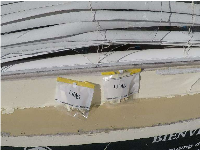
Photograph 1.11-6: Site 1.11 Entrance Kiosk Asbestos Sample A5, A6, None Detected.
