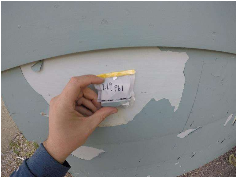
Photograph 1.19-5: Site 1.19 Washroom 4 Lead Sample Pb1, 11,100mg/kg.
