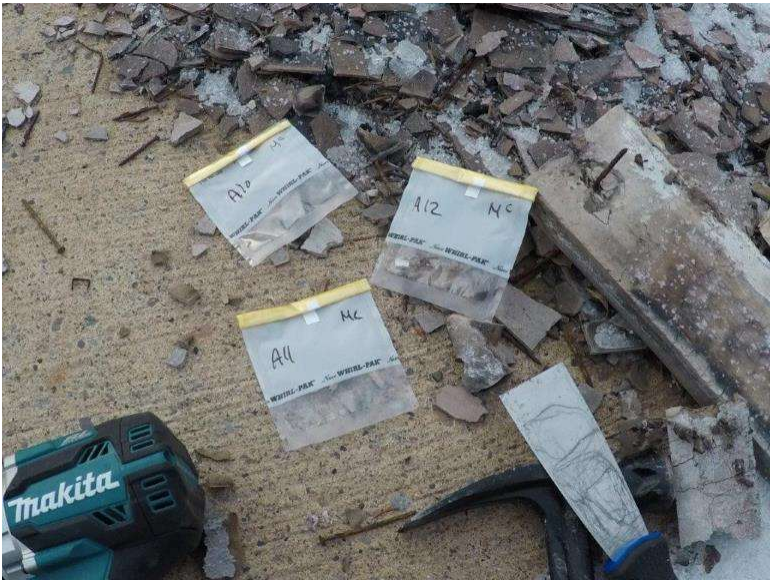
Photograph 9.1-4: Site 9.1 McNealy's Day Use Area - Akamina Parkway Asbestos Samples A10-A12, None Detected.
