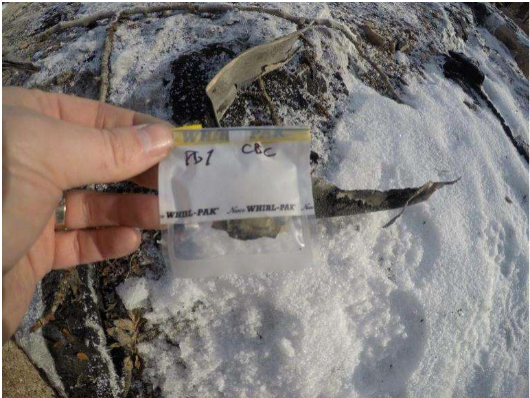
Photograph 2.1-4: Site 2.1 Kitchen Shelter - Crandell Backcountry Lead Sample Pb1, 86mg/kg.
