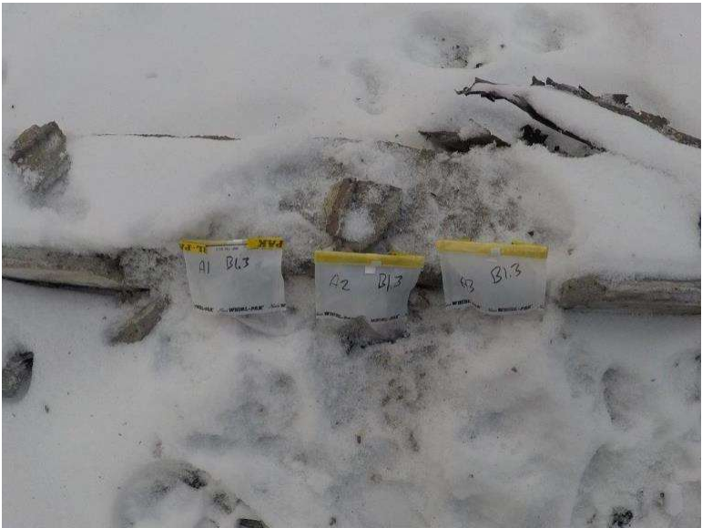
Photograph 1.4-2: Site 1.4 Crandell Campground Washroom 2 Asbestos Samples 1.3-A1 to 1.3-A3, None Detected.
