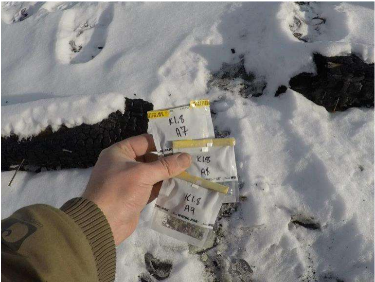
Photograph 1.8-4: Site 1.8 Crandell Campground Kitchen Shelter 4 Asbestos Samples A7-A9, None Detected.
