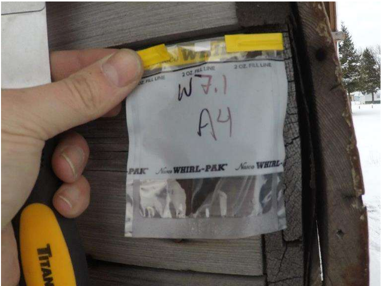
Photograph 7.1-6: Site 7.1 Waterton Townsite Campground Washroom #2 Asbestos Sample A4, None Detected.
