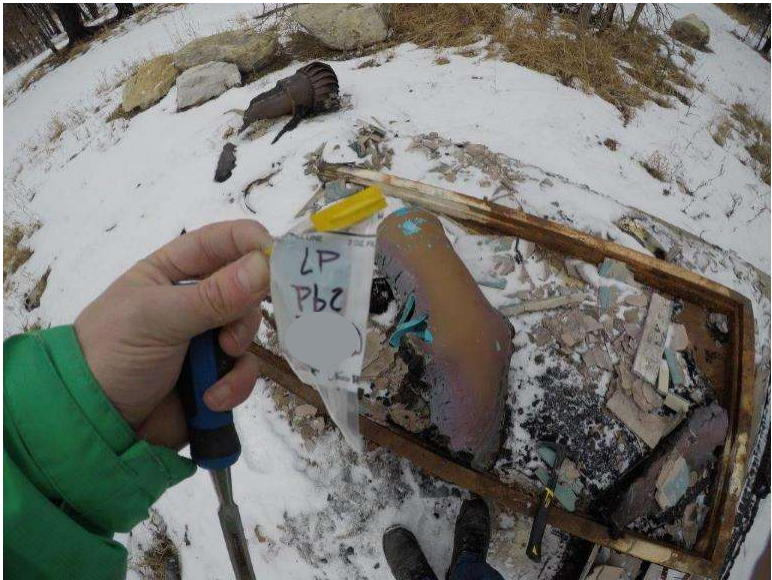
Photograph 9.2-10: Site 9.2 Little Prairie Day Use Area - Akamina Parkway Lead Sample Pb2, <10mg/kg.
