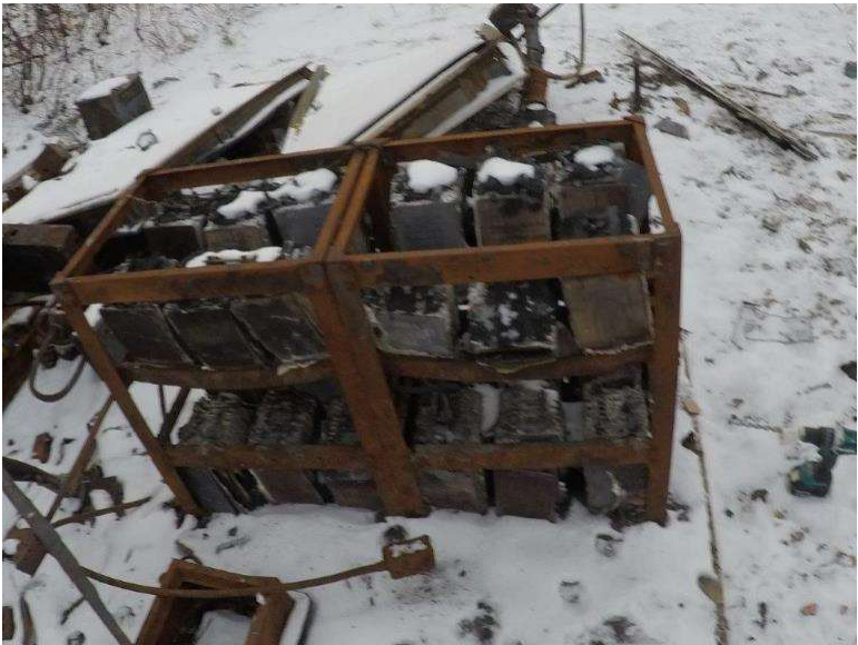
Photograph 1.1-8: Site 1.1 Crandell Campground Generator House, Example of Melted Battery Bank.
