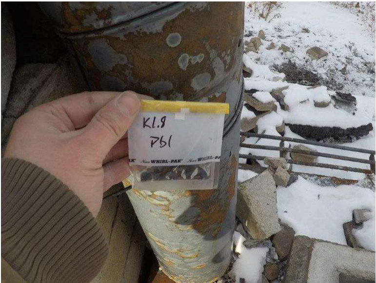
Photograph 1.8-5: Site 1.8 Crandell Campground Kitchen Shelter 4 Lead Sample Pb1, <10mg/kg.
