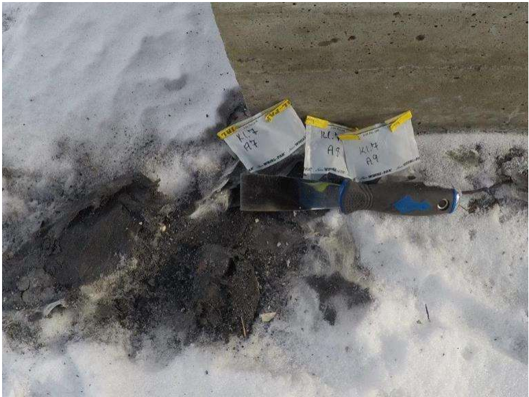
Photograph 1.7-4: Site 1.7 Crandell Campground Kitchen Shelter 3 Asbestos Samples A7-A9, None Detected.
