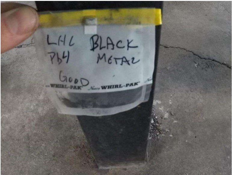
Photograph 8.1-14: Site 8.1 Lost Horse Day Use Area - Red Rock Parkway Lead Sample Pb4, <210mg/kg.
