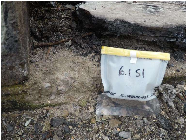
Photograph 6.1-14: Site 6.1 Bear's Hump Seismic Station Silica Sample S1, 46.4% SiO 2 .
