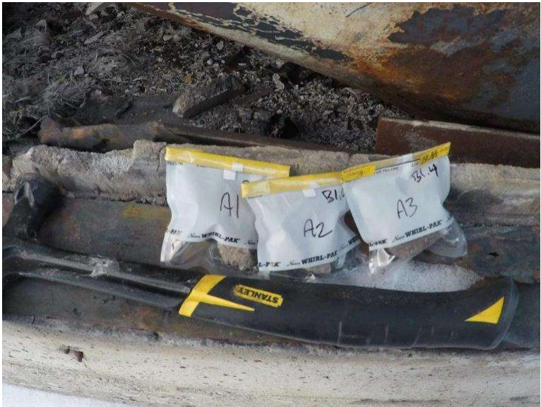
Photograph 1.3-2: Site 1.3 Crandell Campground Washroom 1 Asbestos Samples 1.4-A1 to 1.4-A3, None Detected.
