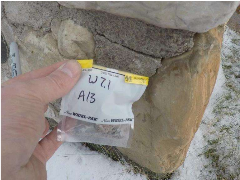
Photograph 7.1-13 Site 7.1 Waterton Townsite Campground Washroom #2 Asbestos Sample A13, None Detected.
