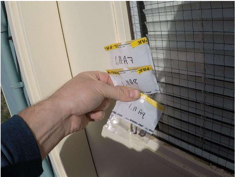
Photograph 1.11-7: Site 1.11 Entrance Kiosk Asbestos Sample A7, A8, A9, None Detected.
