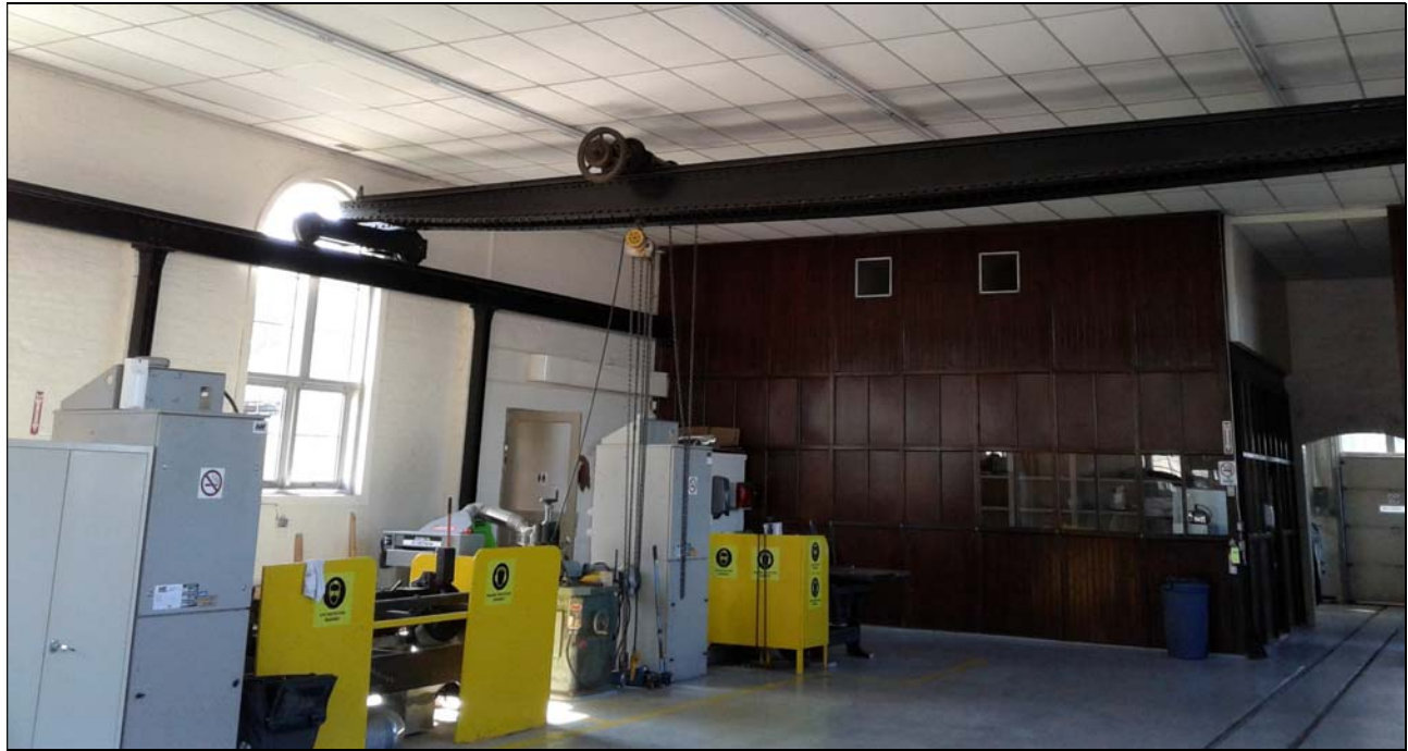
Figure 34: Overhead crane in carpentry shop, showing electric chain hoist
