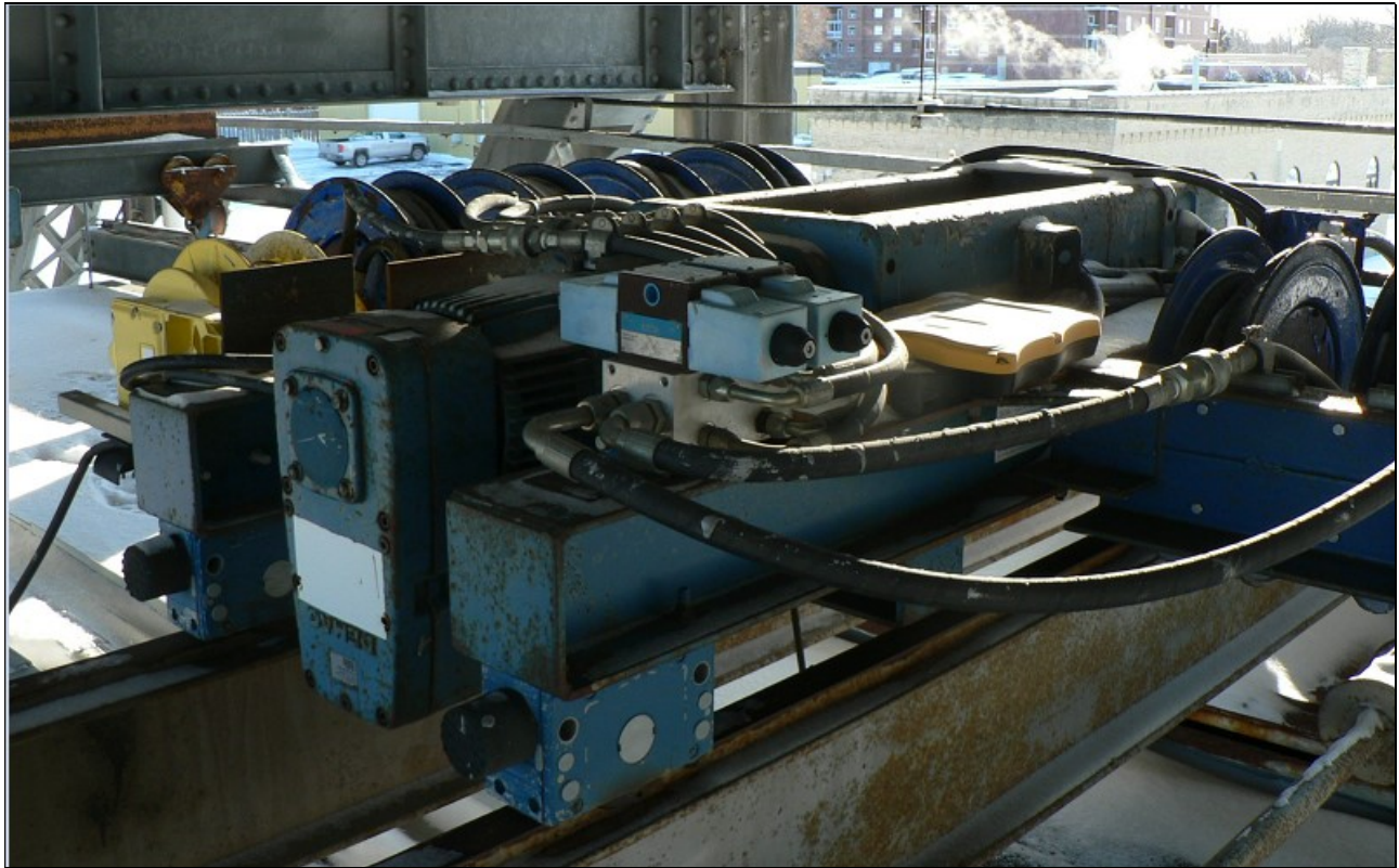
Figure 28: Double-girder overhead crane on operating deck, detail of 5-ton hoist.
