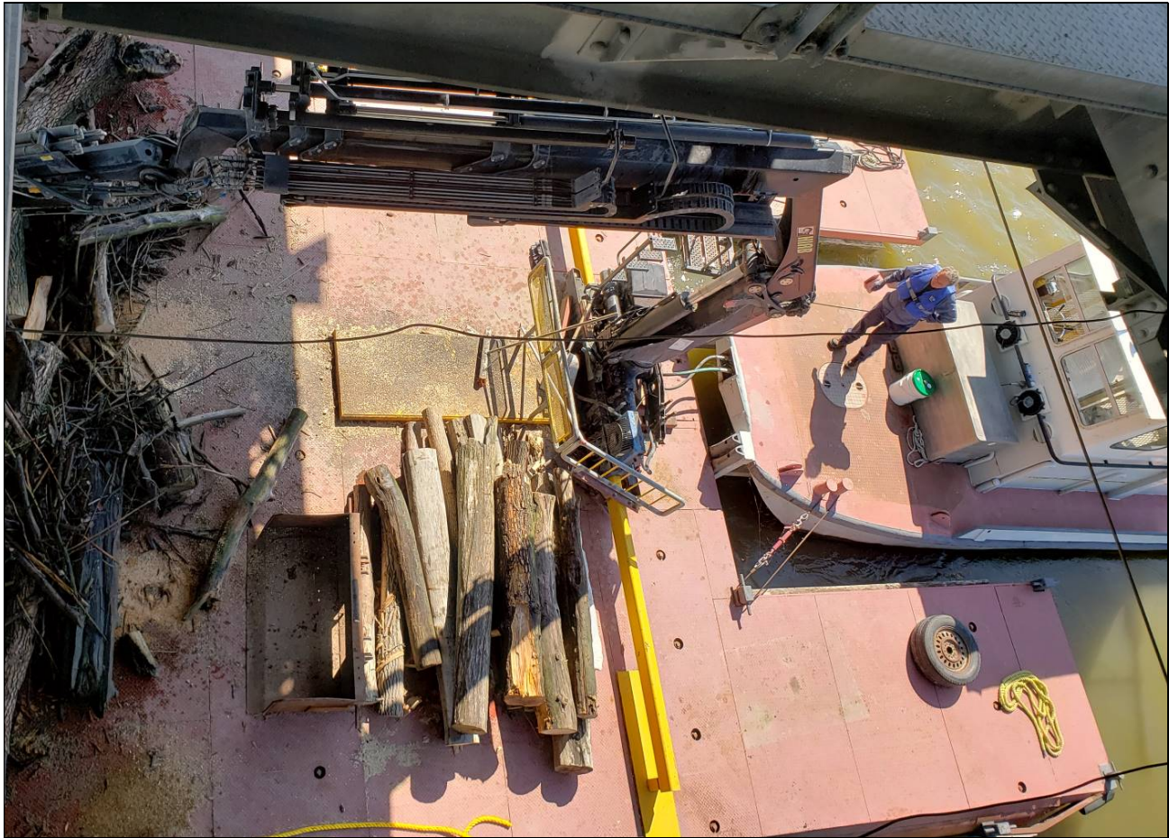
Figure 37: Another view of HIAB 288 articulating crane on SPOONBILL's debris barge.
