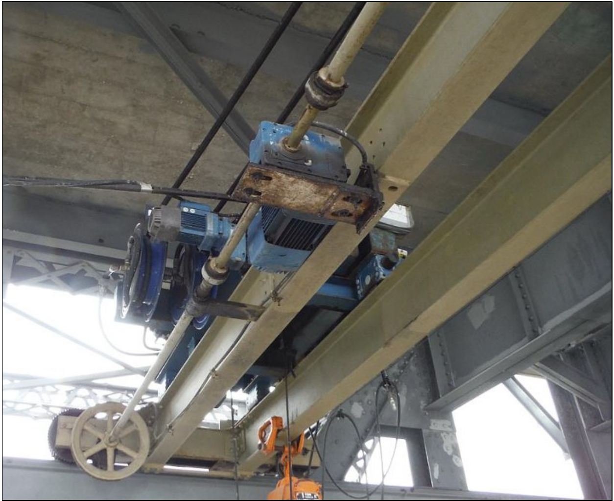
Figure 31: Double-girder overhead crane on dam deck, detail of end truck and underside of 5-ton hoist.
