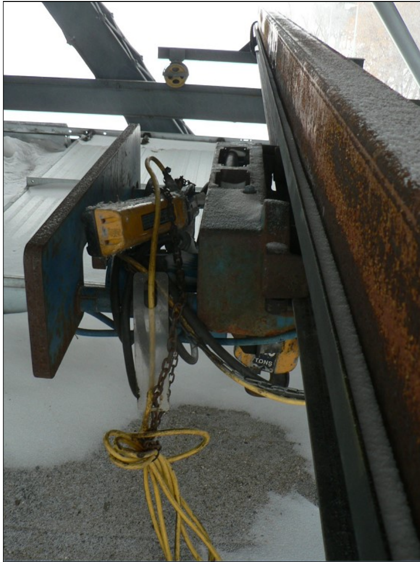
Figure 32: Single-girder overhead crane on operations deck, detail showing 3.5-ton wire rope hoist.
