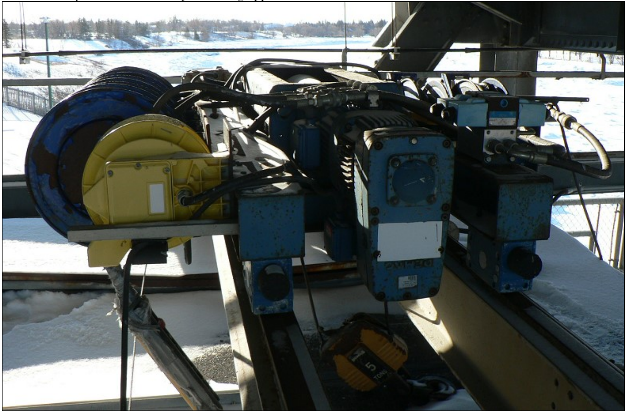
Figure 27: Double-girder overhead crane on operating deck, detail of 5-ton hoist.
