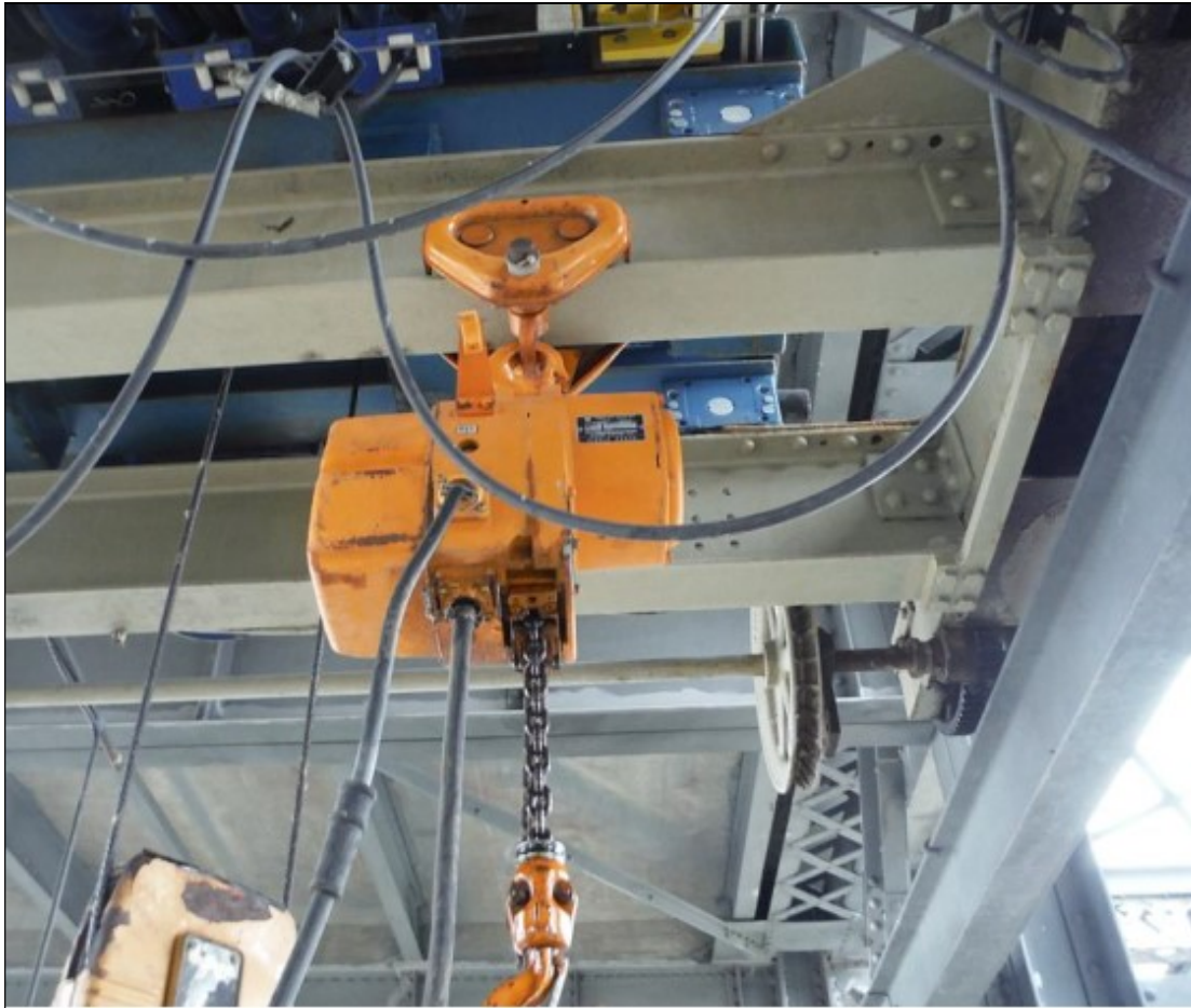
Figure 29: Double-girder overhead crane on operating deck, detail of 1-ton chain hoist and end truck.
