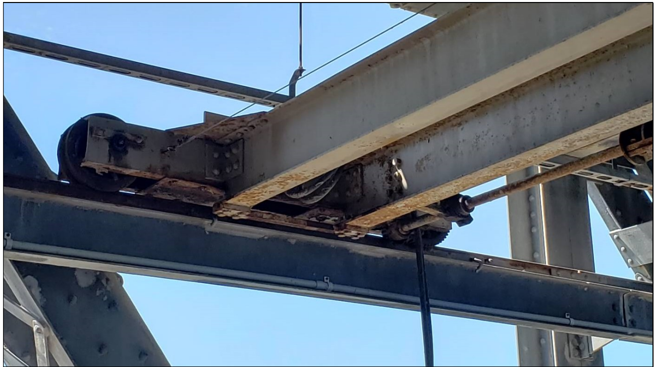
Figure 25: Double-girder overhead crane on operating deck, detail of end truck.
