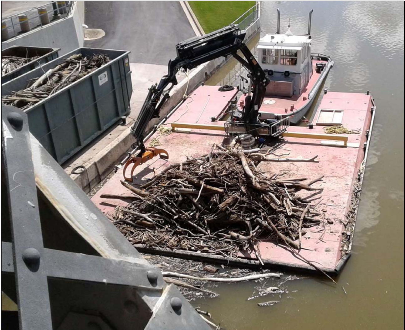
Figure 36: HIAB 288 articulating crane on SPOONBILL's debris barge. Tug SPOONBILL seen behind.
