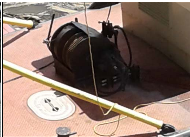
Figure 40: Deck-mounted winch on EMBARRAS, detail
