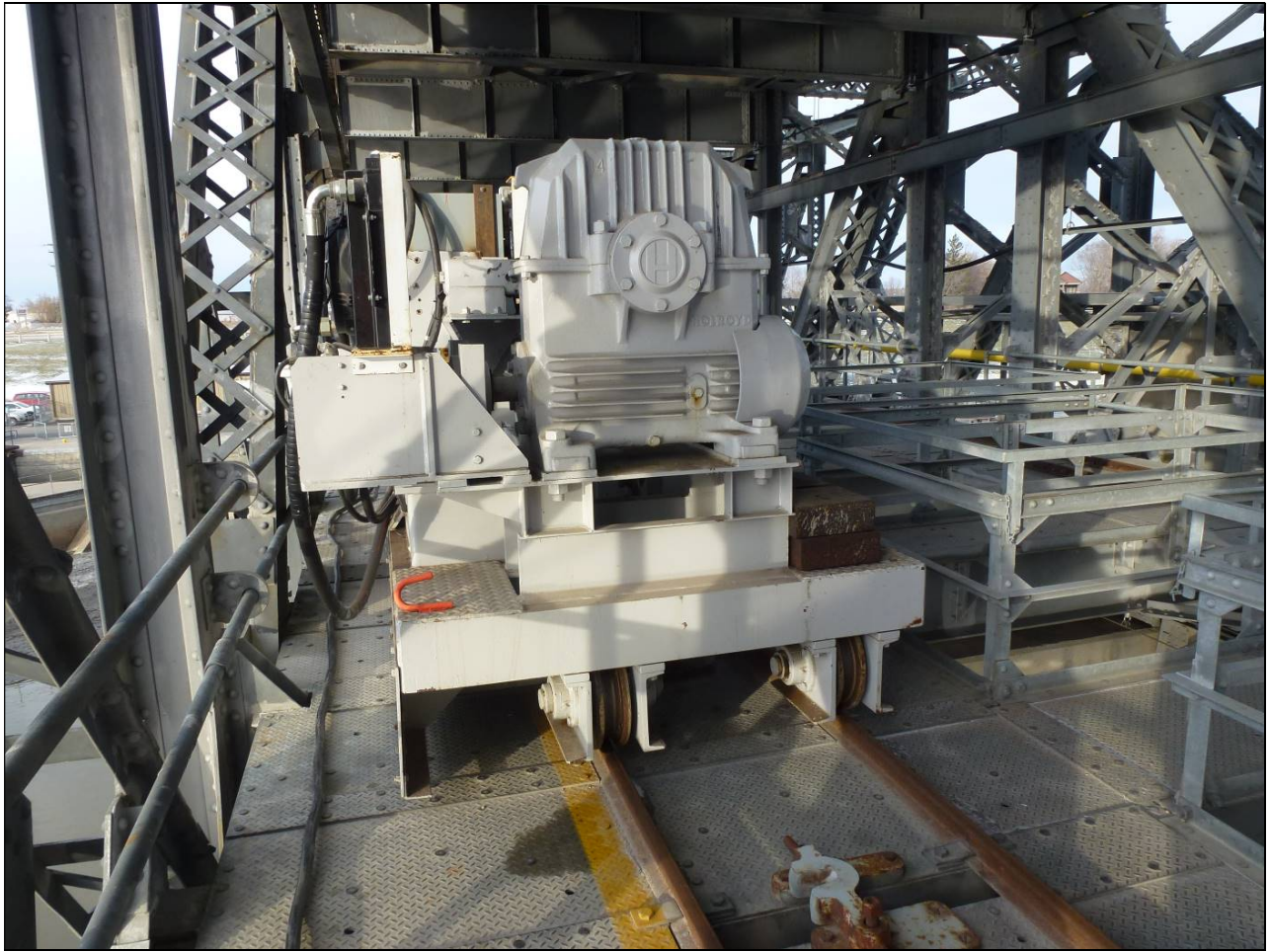
Figure 11: Main frame crane on operating deck, end view.
