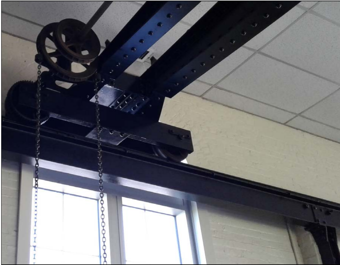
Figure 35: Overhead crane in carpentry shop, detail of end truck
