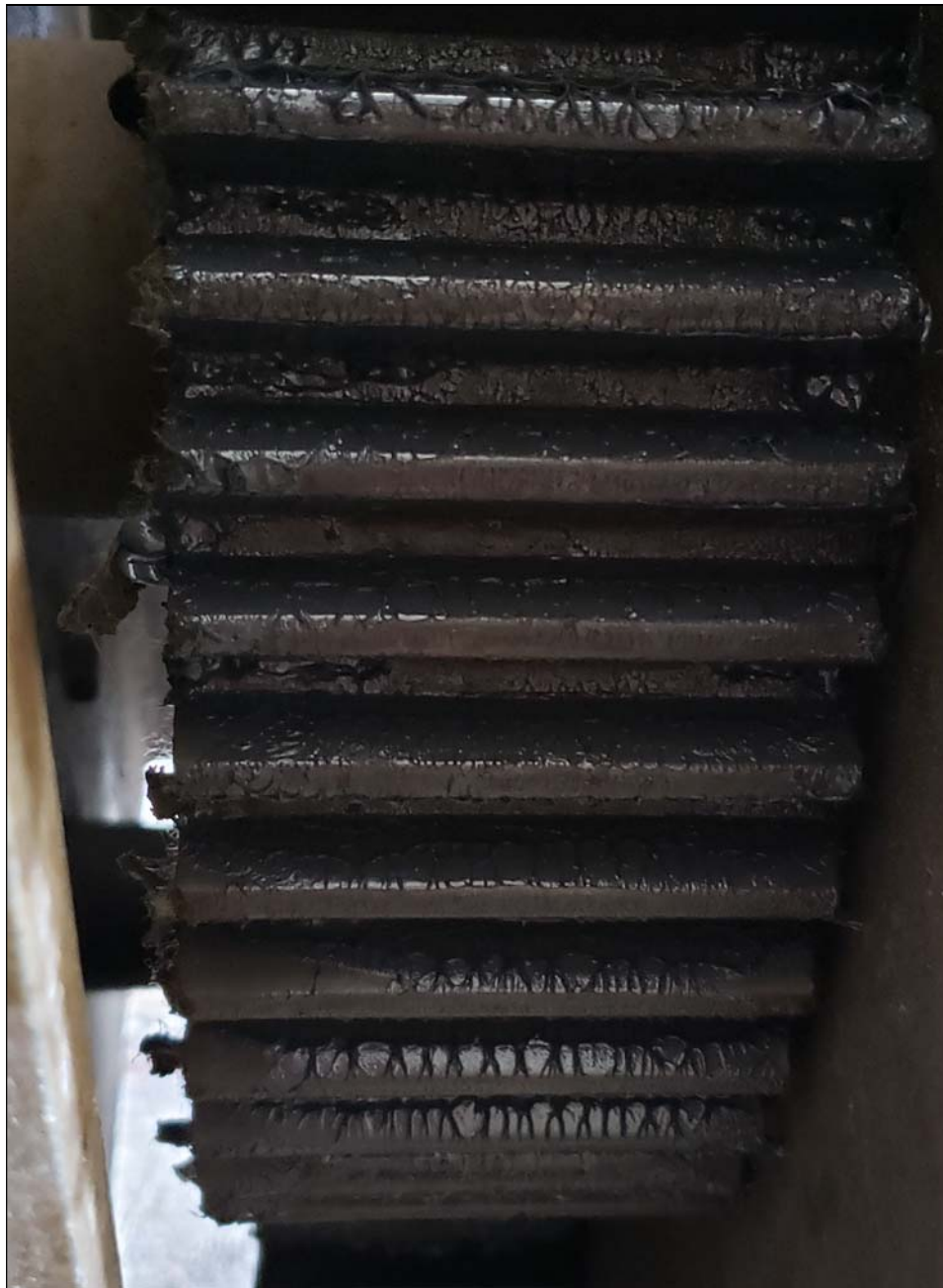
Figure 21: Curtain crane, spur gear detail
