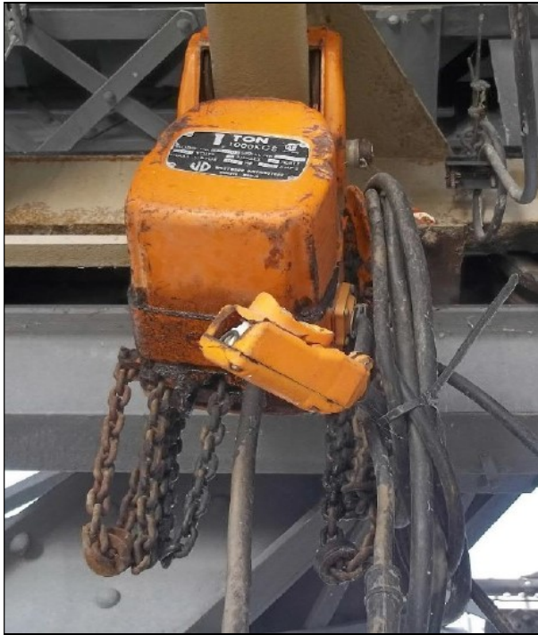
Figure 30: Double-girder overhead crane on operating deck, detail of 1-ton chain hoist.
