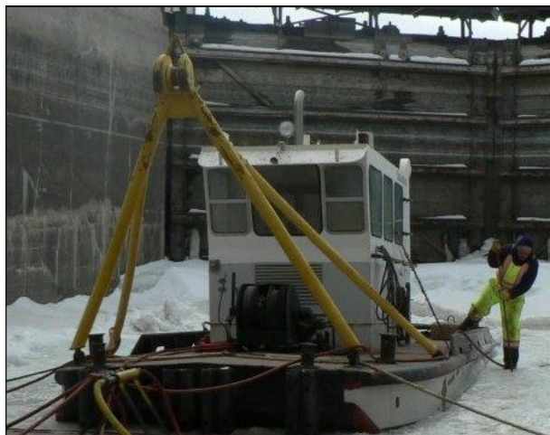
Figure 39: Deck-mounted winch on EMBARRAS
