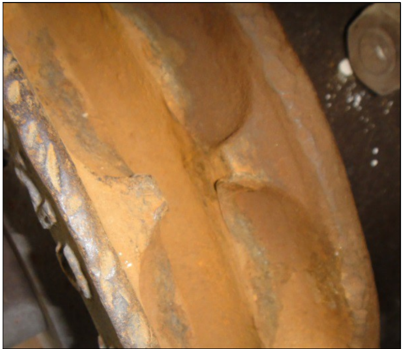
Figure 23: Curtain crane, worn pocket wheel in 2015.
