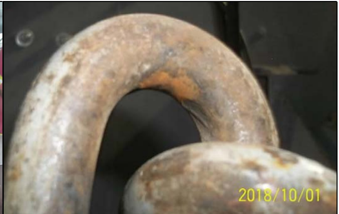
Figure 14: Frame cranes, lifting chain, typical condition from 2018 General Inspection report.
