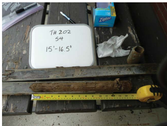
Photo 5: Lock 39 Earthfill Embankment (TH13-202, S4 and depth 15'-16.5') Note: clayey silt to silty clay
