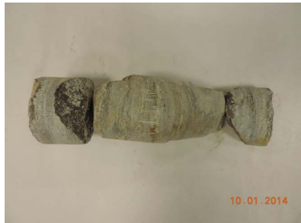
Photo 2: Right Earthfill Embankment (TH13-101, Bedrock Core and depth 21.0') Note: limestone bedrock
