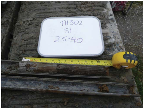
Photo 7: Northwest Canal Embankment (TH13-302, S1, and depth 2.5'-4.0') Note: clayey silt to silty clay
