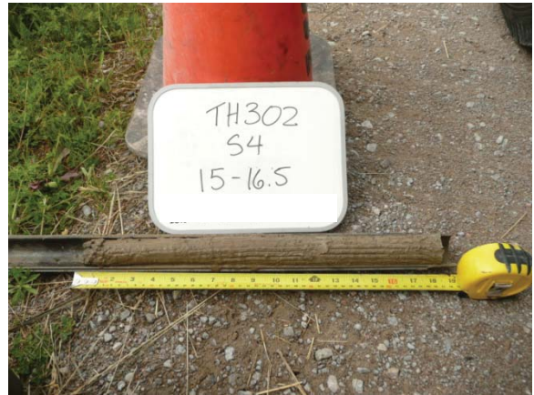
Photo 9: Northwest Canal Embankment (TH13-302, S4, and depth 15'-16.5') Note: clayey silt to silty clay
