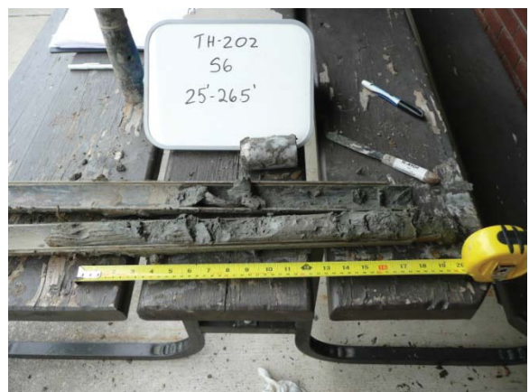
Photo 6: Lock 39:Earthfill Embankment (TH13-202, S6, and depth 25'-26.5') Note: clayey silt to silty clay
