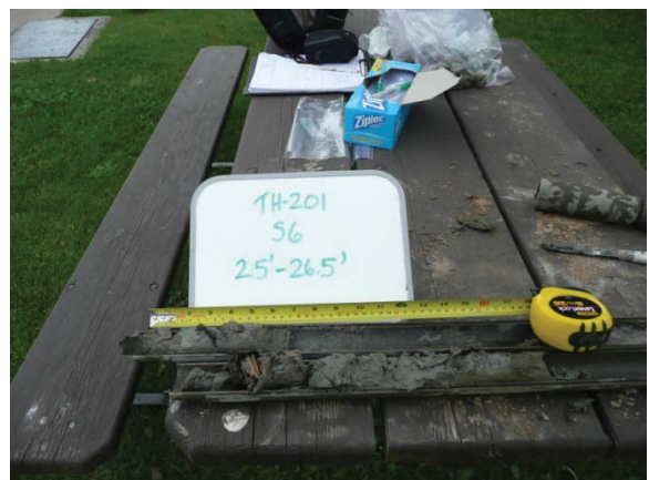
Photo 4: Lock 39 Earthfill Embankment (TH13-201, S6, and depth 25'-26.5') Note: clayey silt to silty clay
