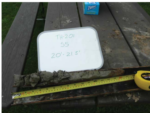
Photo 3: Lock 39 Earthfill Embankment (TH13-201, S5, and depth 20'-21.5') Note: clayey silt to silty clay
