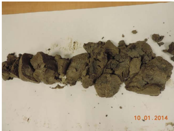
Photo 1: Right Earthfill Embankment (TH13-103, S8, and depth 14'-16') Note: sandy silt to silty sand
