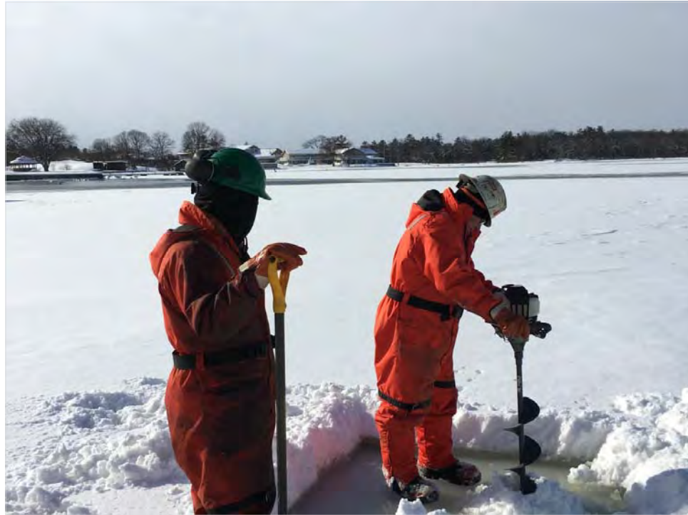
Photo 13: Dam C, drilling through ice, February 2018. Same technique used in all sampling locations at Dam C.
