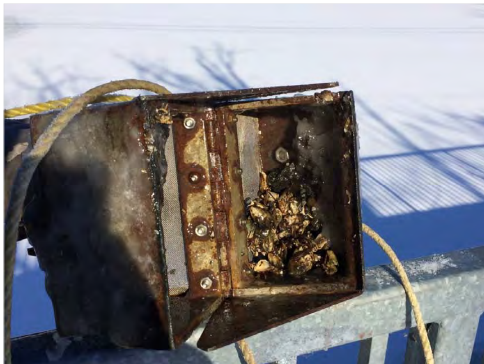
Photo 10: Dam E, Sampling Location 2, absence of sediment using ponar, December 2017.
