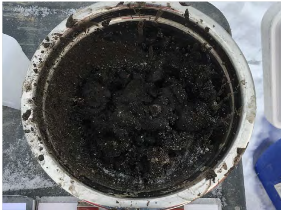
Photo 14: Dam C, Sample Location 101, surface sediment sample, February 2018. Similar to other sediment samples collected at Dam C.
