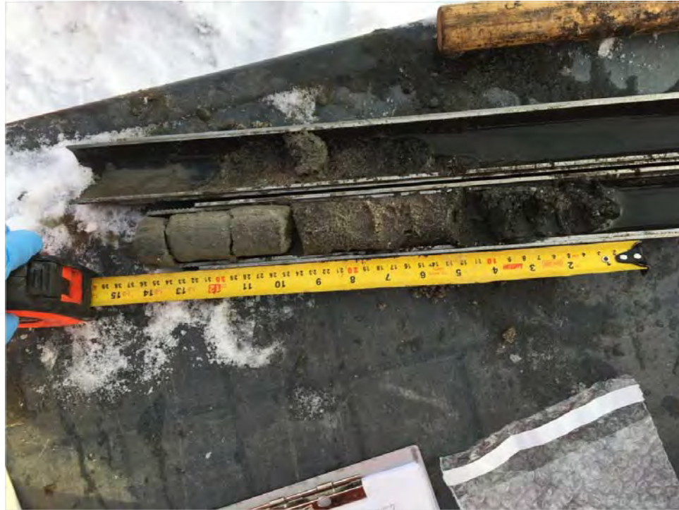
Photo 17: Dam G, Sampling Location 101, shallow sediment sample in split spoon, February 2018.
