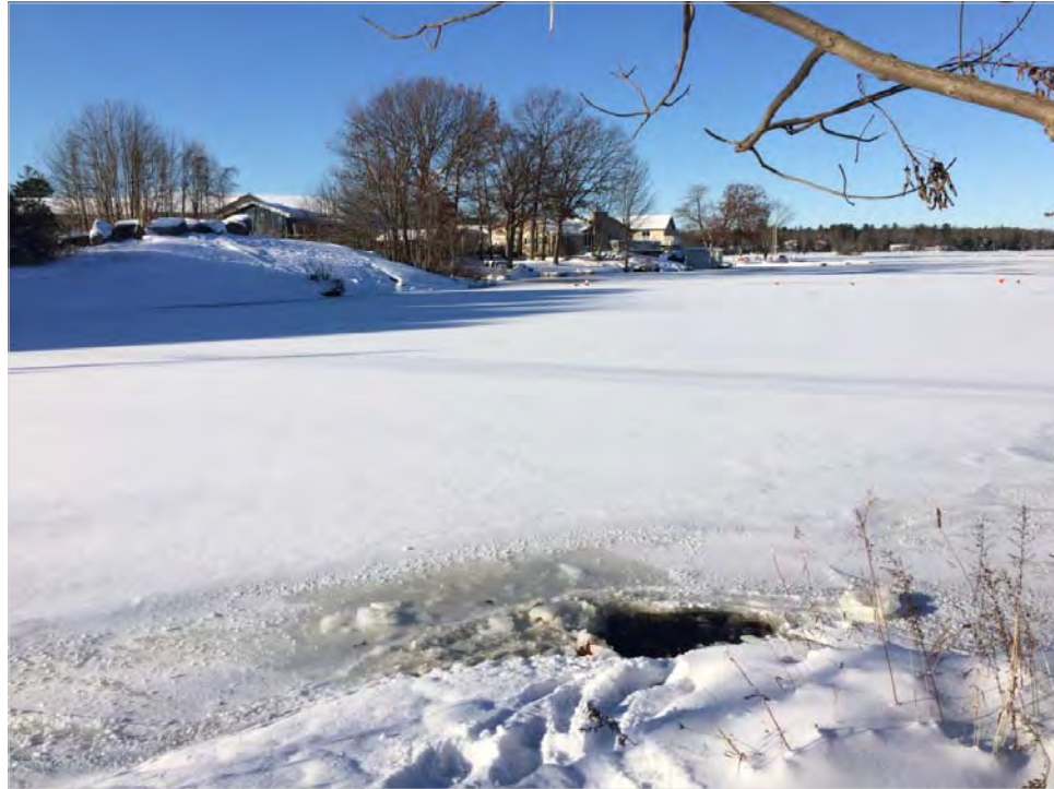
Photo 7: Dam E, Sampling Location 6, hole following sample collection using manual corer, December 2017.
