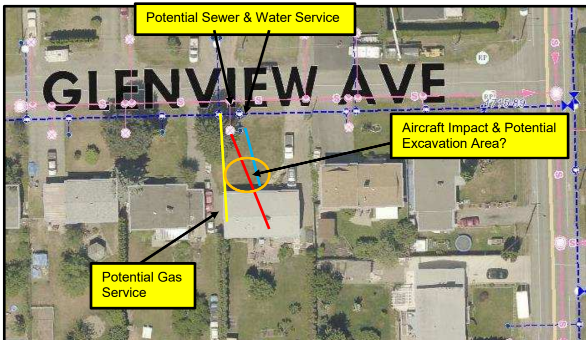
Photo 2: Kamloops GIS Location Map of 2425 Glenview Drive. Note Estimated Locations For Building Services Below Grade.
