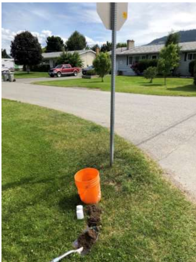
Photo 13: Background soil sample obtained 0.05 - 0.15 m below ground surface on 19 June 2020
