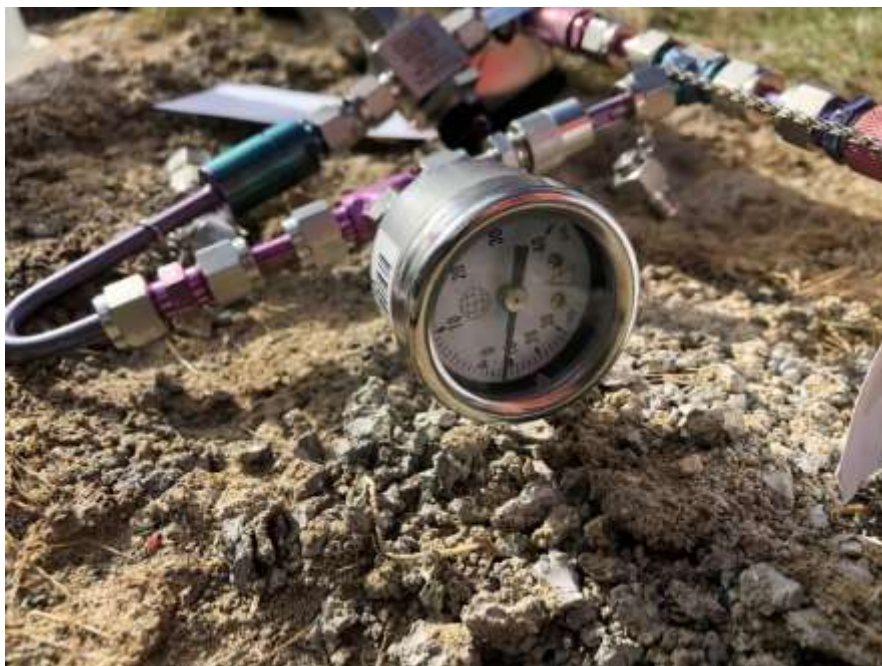
Photo 12: Flow regulator and vacuum gauge of Summa Cannister samples.
