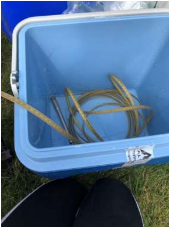
Photo 10: Equipment decontamination with PFAS-free water bath 18 June 2020.
