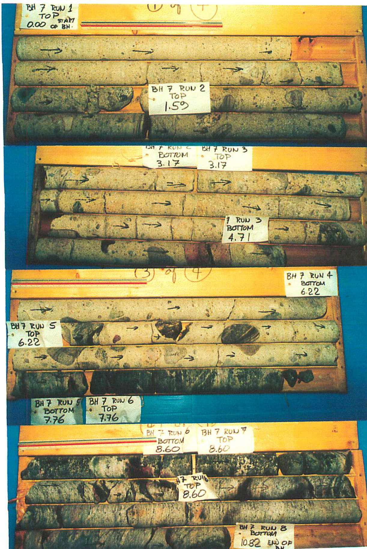
Port Severn Dam Concrete and Rock Core Borehole No. 7
