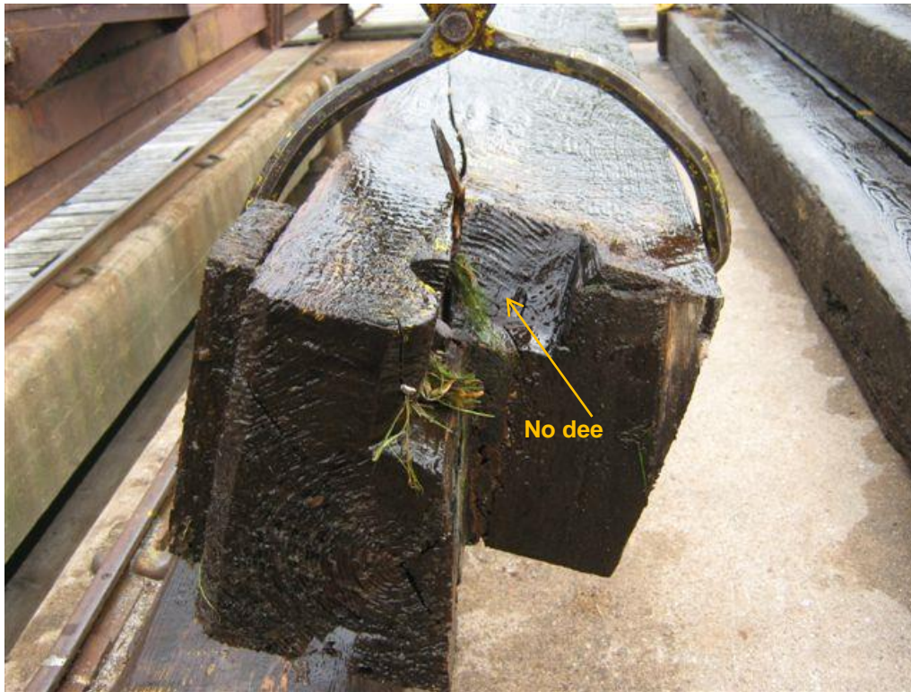
Photo 43: Use of tongs to remove a log with a broken dee
