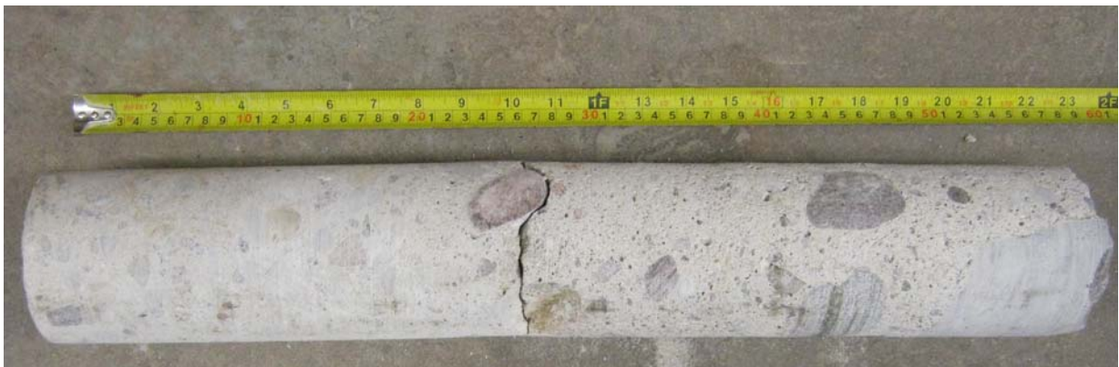
Picture 18: Dam G: Concrete core from Corehole CH-G03. Upper patch/ repair.
