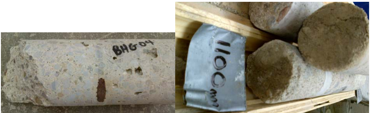
Picture 20: Dam G: Corehole CH-G04, Left photo , Upper patch/ repair Corehole CH-G04. 10M reinforcing steel shown. Right photo , soil deposits on fracture at 1100mm depth.
