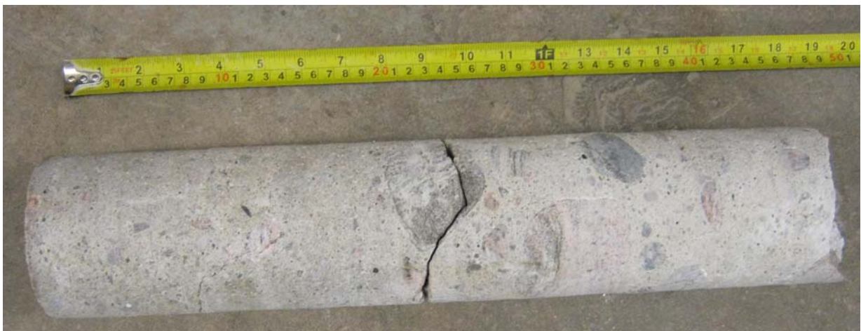
Picture 2: Dam C: Concrete core from Corehole CH-C02.
