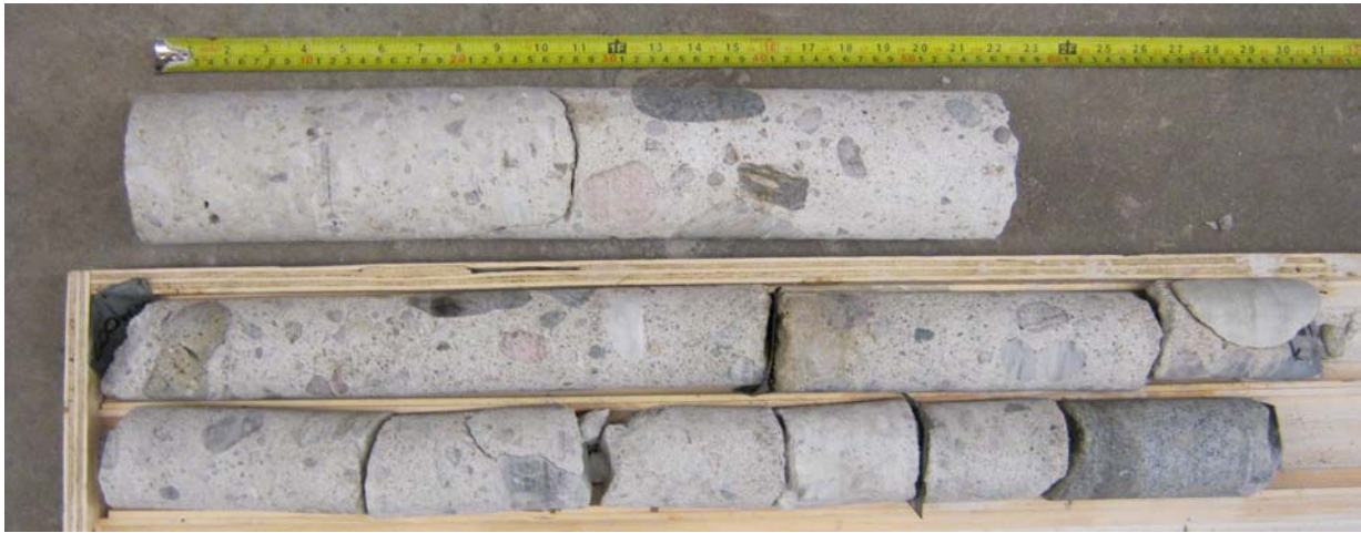
Picture 19: Dam G: Concrete core from Corehole CH-G04. Upper portion patch/ repair.
