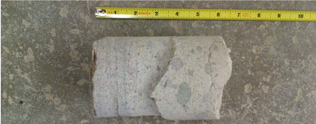
Picture 4: Dam C: Last section of 100mm diameter concrete core at 550mm depth Corehole CH-C03. A 50mm portion of Schist cobble shown, pyrite present along fracture.
