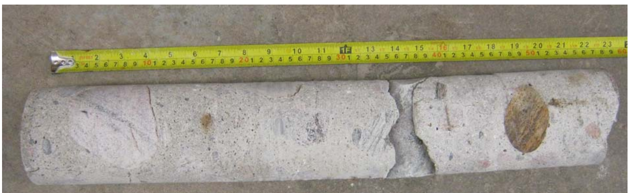
Picture 3: Dam C: Upper portion of concrete core from Corehole CH-C03.
