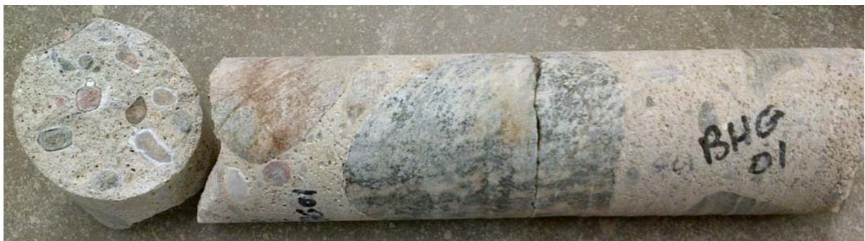
Picture 21: Dam G: Corehole CH-G01. Large diameter aggregates shown along with white chalky paste around aggregates. 100mm diameter core.
