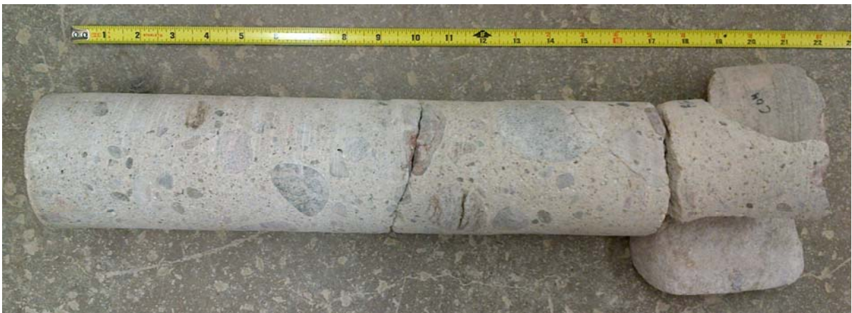
Picture 6: Dam C: Concrete core from Corehole CH-C04.
