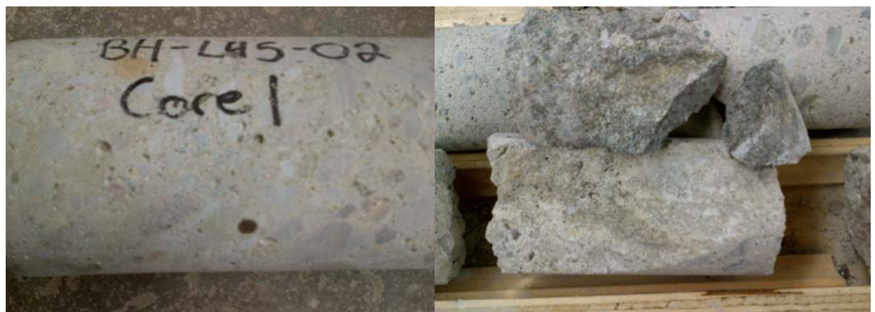
Picture 15: Lock 45: Corehole CH-L45-02, photo on the left showing 6mm diameter steel, photo on the right showing aggregate containing pyrite.
