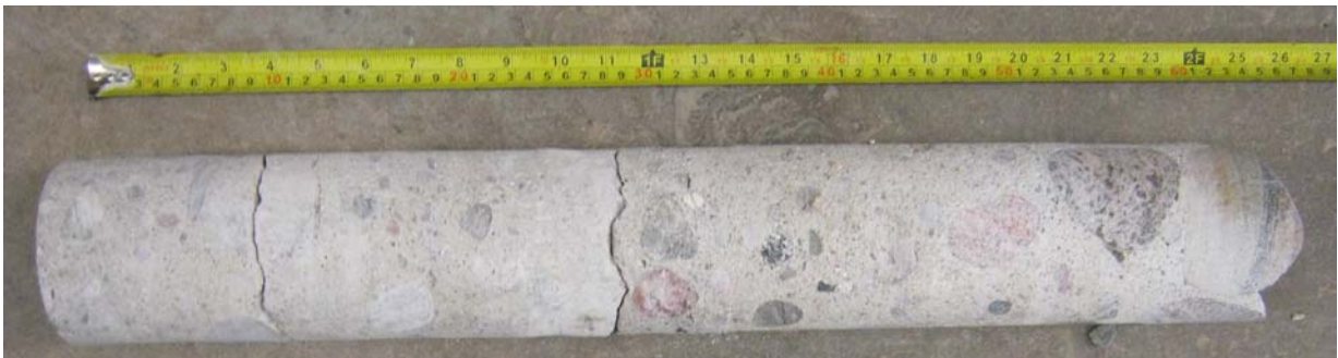
Picture 8: Dam D: Concrete core from Corehole CH-D01.
