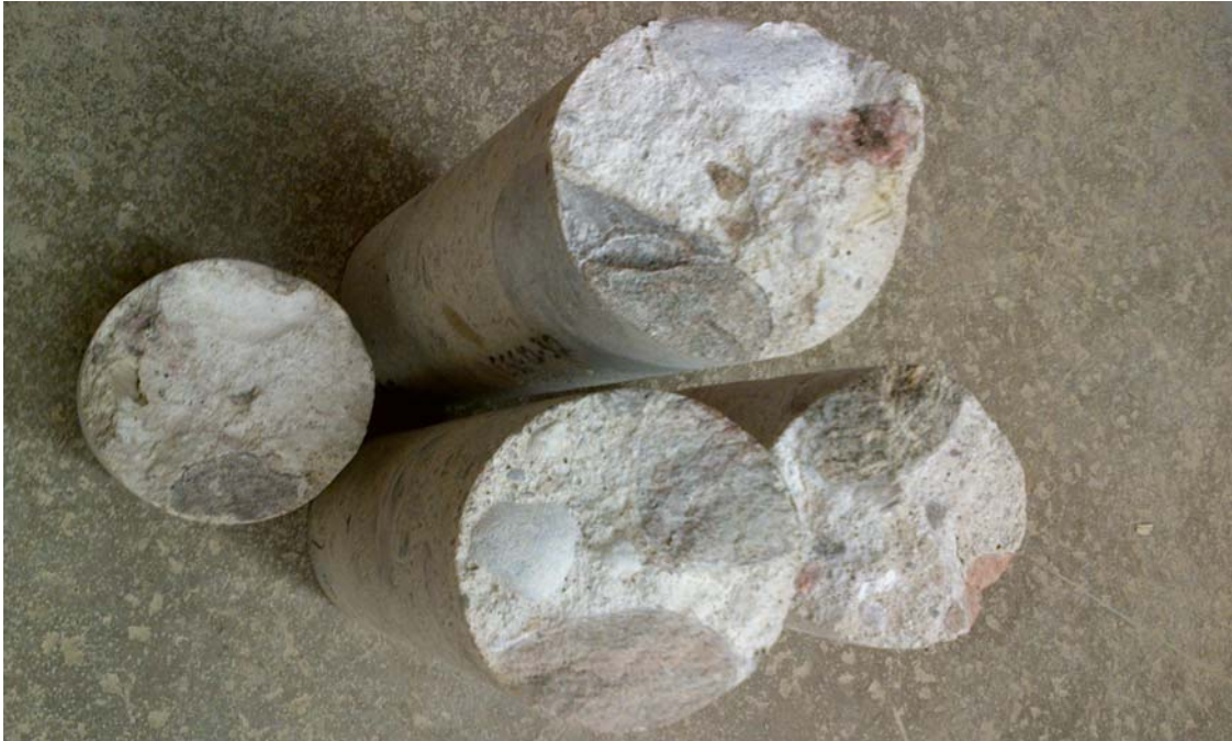
Picture 7: Concrete cores, Dam C, chalky white paste on faces of fractures.
