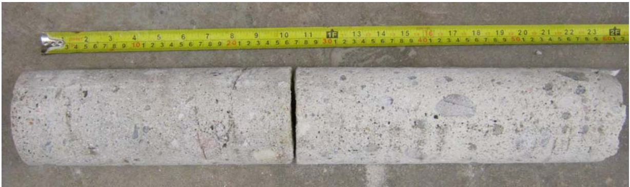
Picture 17: Dam G: Concrete core from Corehole CH-G02. Cold joint shown.
