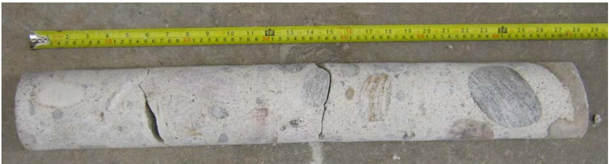
Picture 11: Dam E: Concrete core from Corehole CH-E01.
