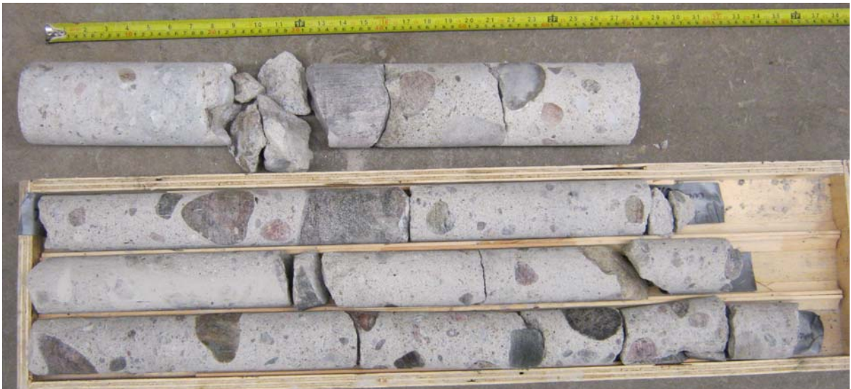
Picture 14: Lock 45: Concrete core from Corehole CH-L45-02. Upper patch/ repair.
