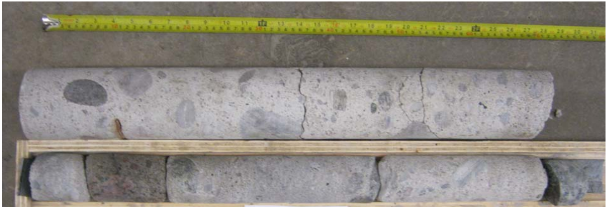
Picture 10: Dam D: Concrete cores from Corehole CH-D02.
