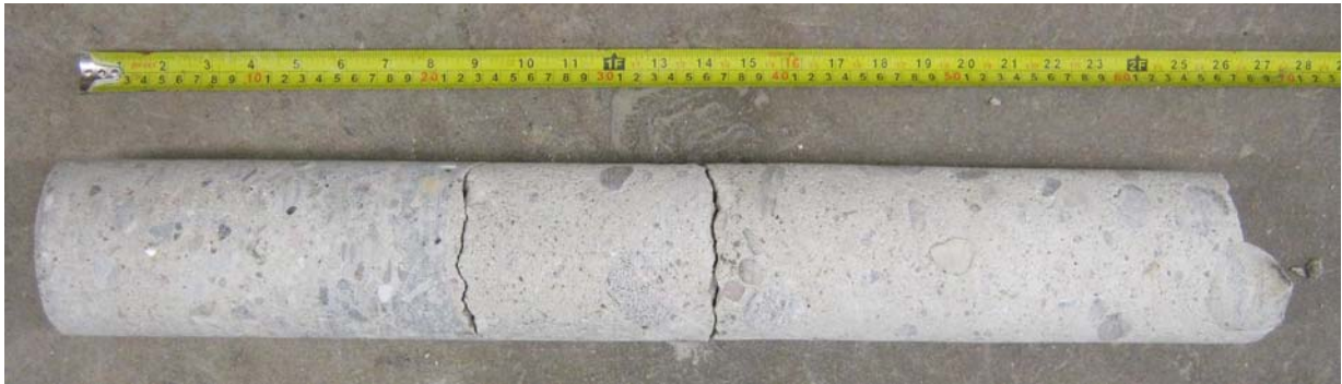
Picture 13: Lock 45: Concrete core from Corehole CH-L45-01. Upper patch/ repair.
