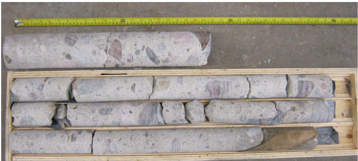
Picture 12: Dam E: Concrete core from Corehole CH-E02.
