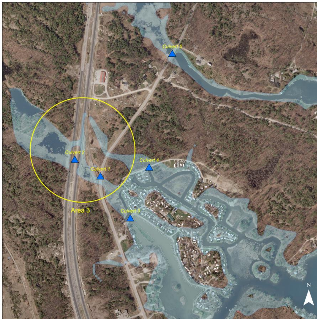
Figure 8.3 Openings in Reservoir Rim at 181.35 m (Area 3)
