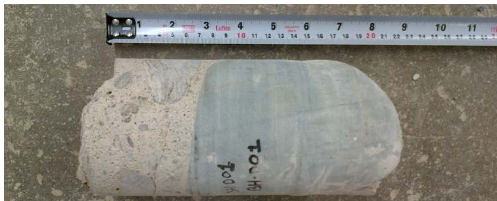
Picture 9: Dam D: Large aggregate at the bottom of the core sample, Corehole CH-D01.
