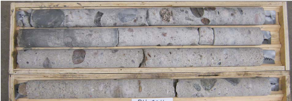
Picture 5: Dam C: Lower portion of the concrete core from Corehole CH-C03.
