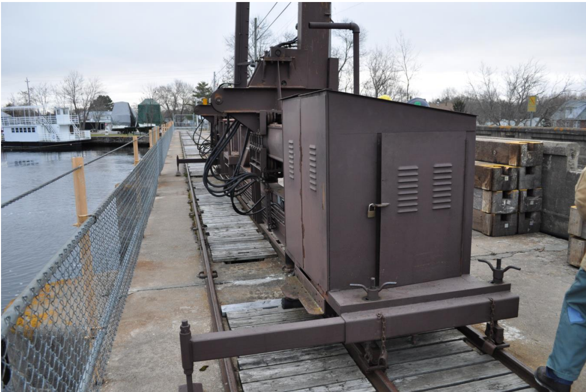
Photo 26: Hydraulic log lifter
