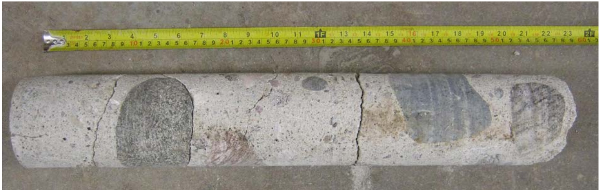
Picture 16: Dam G: Concrete core from Corehole CH-G01.
