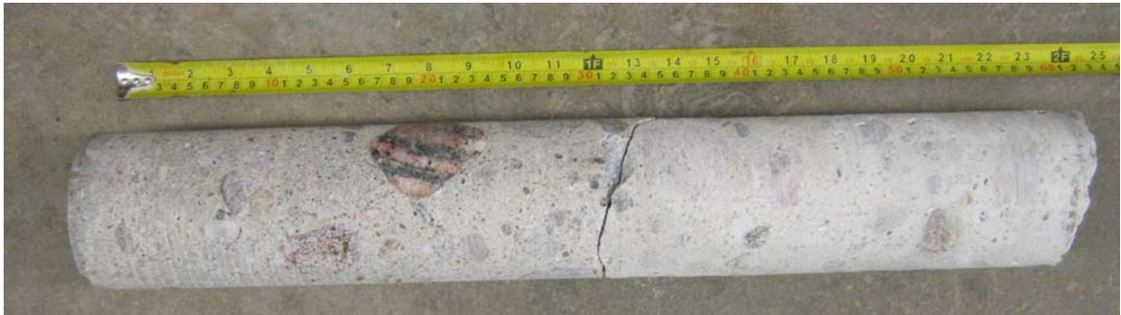
Picture 1: Dam C: Concrete core from Corehole CH-C01.
