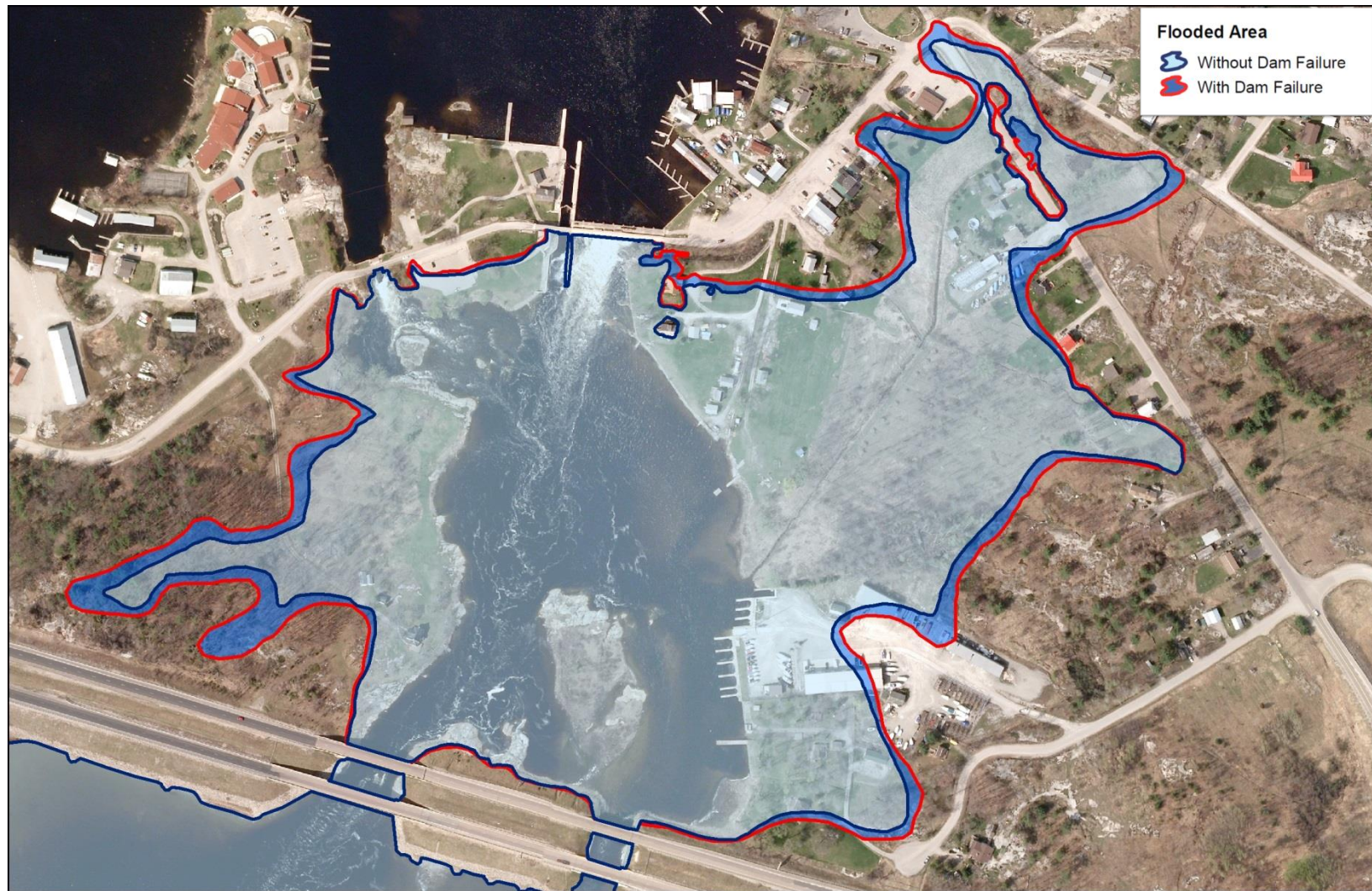
Figure I.5 Main Dam – Inundation mapping – PMF Scenario (With and Without Dam Failure)
