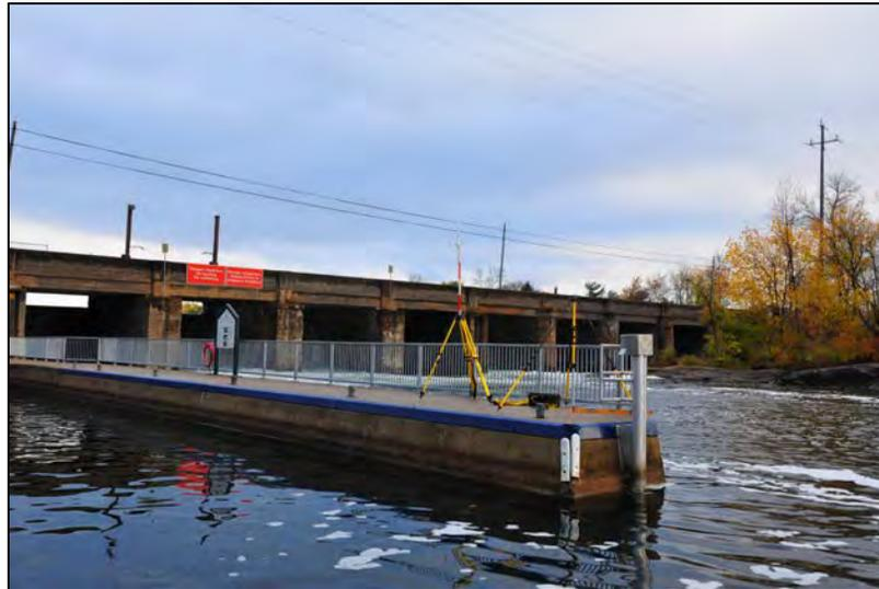
Figure 19: RTK-DGPS base station setup on Lock 45 Lower Approach Wall
