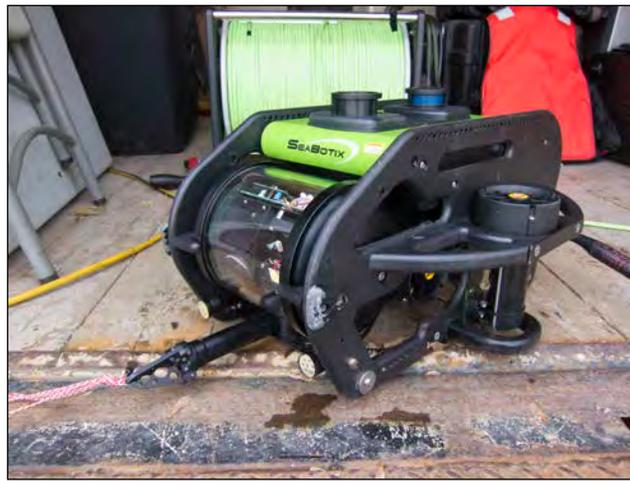
Figure 13: SeaBotix LBV300-5 prior to deployment
