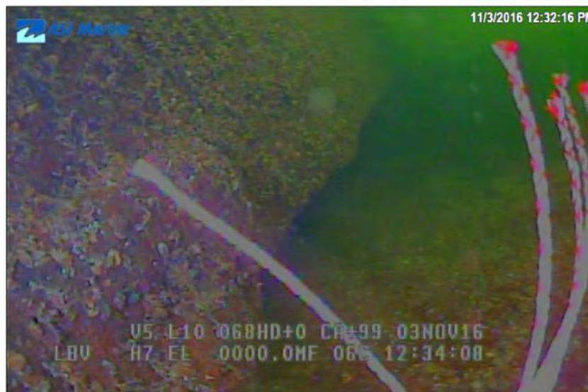
Figure 29: Undercutting observed beneath Gate 2 footing
