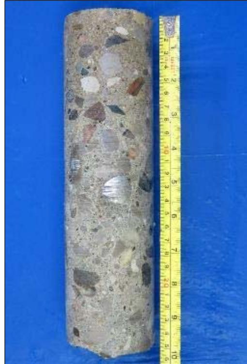
**CORE C3** (Lock 45/Main Dam common wall)
