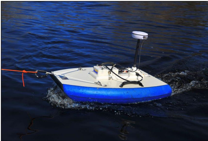
Figure 5: Sontek RiverSurveyor M9 ADCP installed on hydroboard
