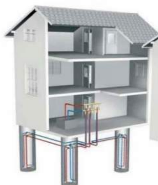
Figure 12: Geothermal pile foundations (Gordeyev et al.)
