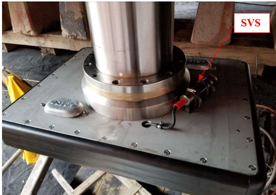
Figure 2: SVS mounting configuration on transducer pod assembly
