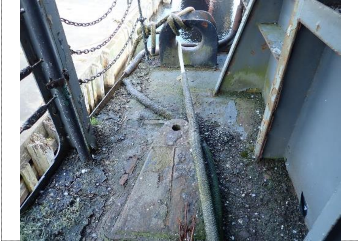
17. Stbd aft – emergency towing connection
