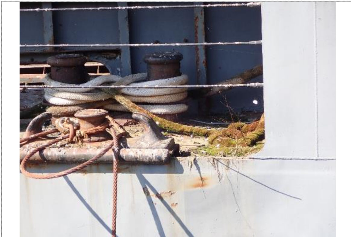
10. General condition of mooring ropes and wires
