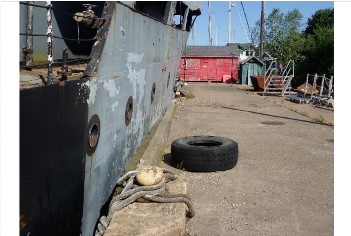
6. Stbd side looking forward – note condition of mooring ropes and minimal fendering
