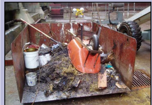
INADEQUATE waste grit storage.
