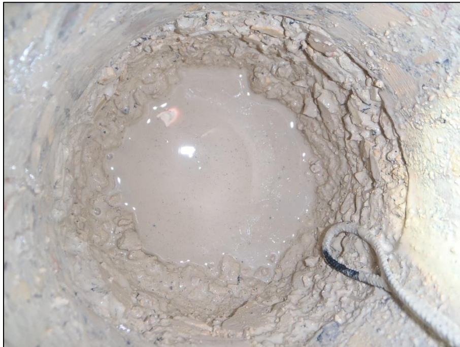
Photograph 4: Gravel leveling base below the concrete slab in Core #1
