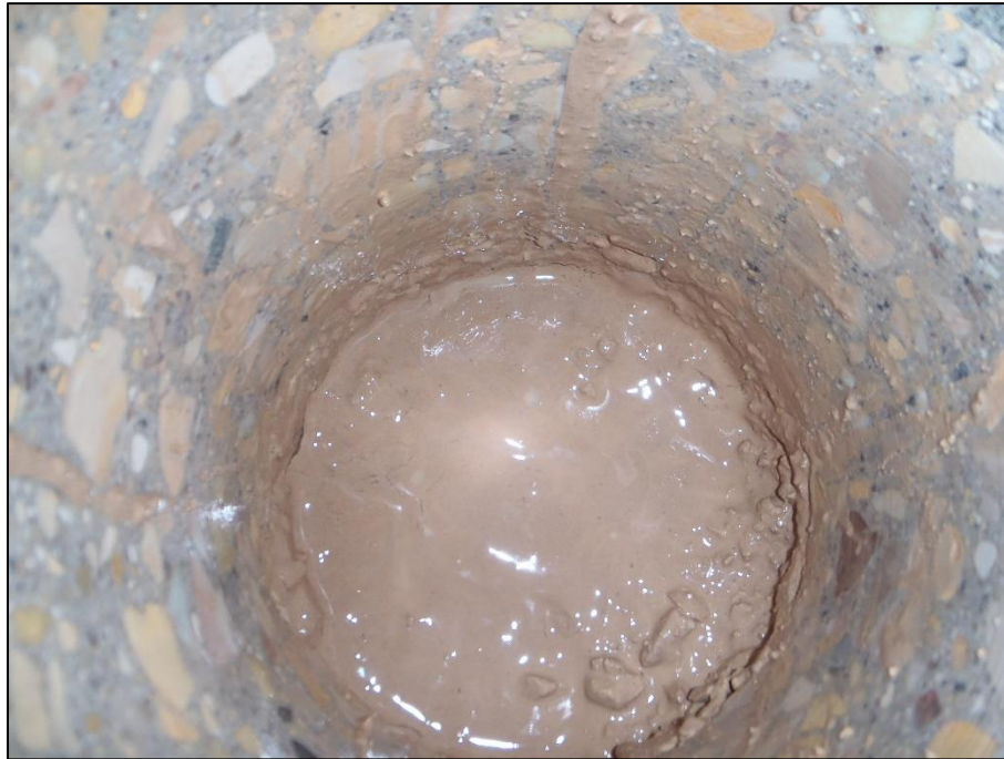
Photograph 5: Clay intermixed in crushed gravel below the concrete slab at Core #2
