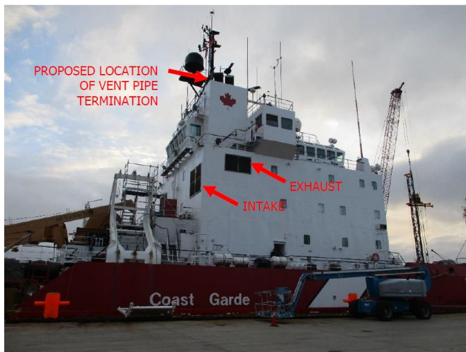
Photograph 11 - Terry Fox superstructure. Note location of casing and engine room intake and exhaust vents.
