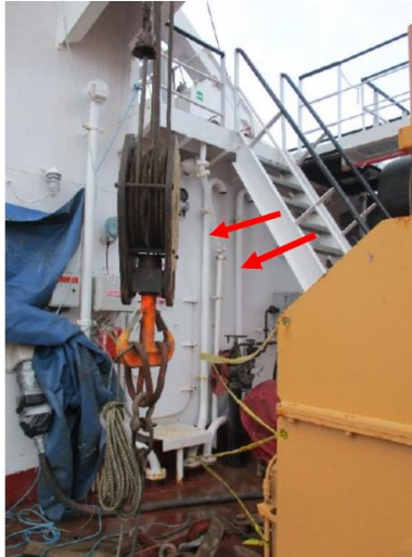
Photograph 3 - Aft deckhouse bulkhead showing location of existing vent pipes starboard side
