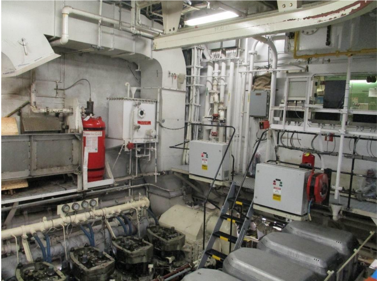
Photograph 1 - Aft engine room bulkhead showing location of existing vent pipes and vapour traps.
