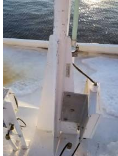
Drawing #2 & Photo #10 – Example of a Modified MF-HF Antenna Mount
