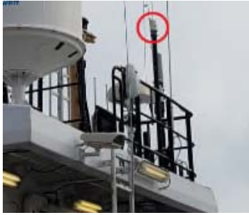
Photo #9 – Example of a Relocated Iridium Antenna
