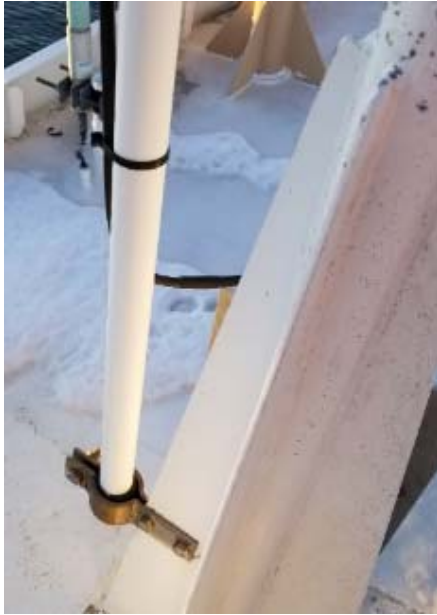
Photo #11 – Example of a Modified MF-HF Antenna Mount
