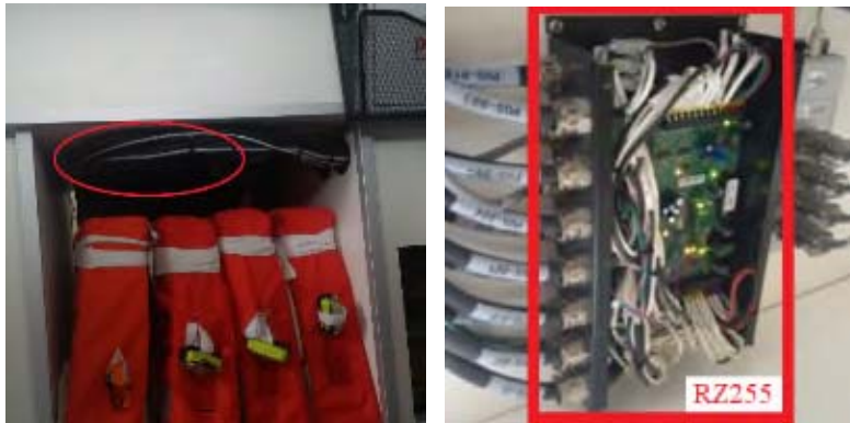
Photo #20 – RZ 255 NMEA Distribution Unit below Chart Table
