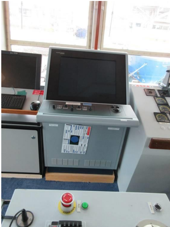
Pictures: X-Band Radar Console (Display B) and Associated Equipment
