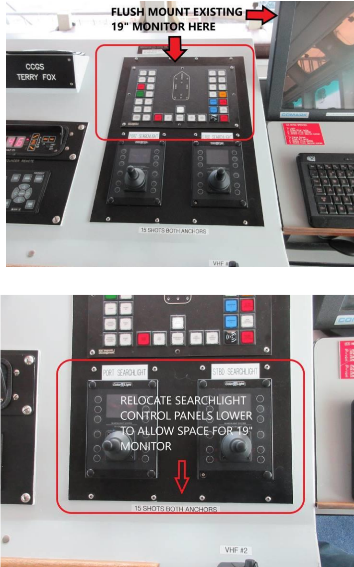
Picture: 19" Monitor Location and Searchlight Control Panels
