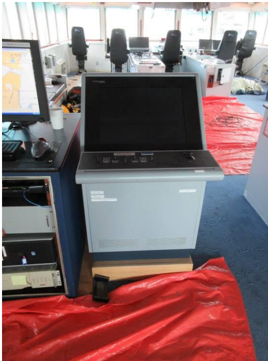
Pictures: S-Band Radar Console (Display A) and Associated Equipment
