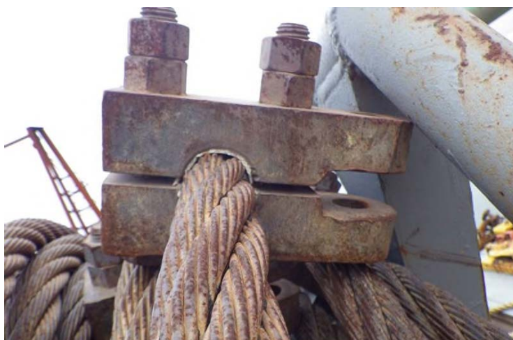
Figure 2: Clamps assembled on a section cable
