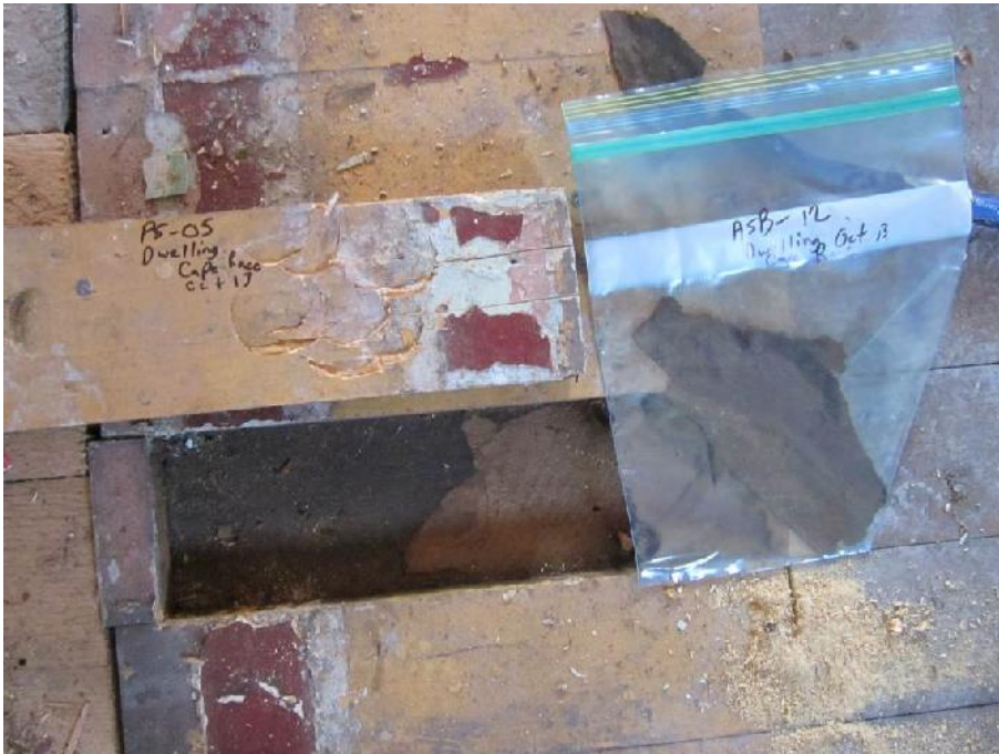
Photo 37: View of location of paint sample PS-05 (also tar paper sample AS-12) in Room 6 (floor).
