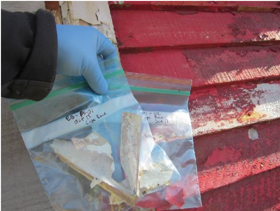
Photo 19: View of location of paint samples EQ-PS-1 and EQ-PS-2 (exterior wall). Note: SVG on the white paint sample.
