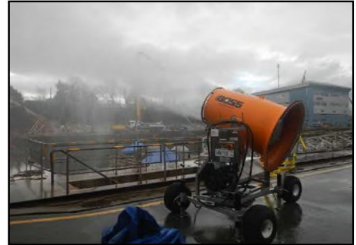
Dust suppression unit in operation.
