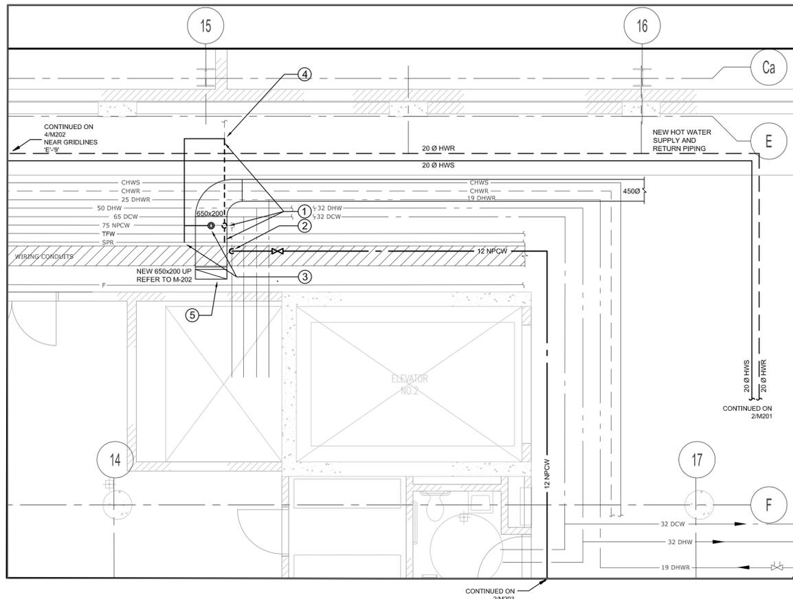
**1 PARTIAL 1-ST FLOOR PLAN - PIPING - DEMOLITION & NEW WORK**
