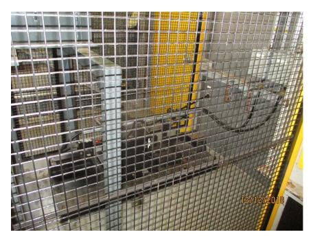
Photo E31 Span Resolvers. One single turn resolver and one multi-turn resolver have been connected to a gearbox which are attached to the tower pinion shaft. The resolvers and their junction box along with the gearbox are protected by a steel mesh cage as indicated.
