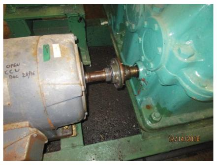
Photo M31 South Span Lock Machinery. The motor shaft, coupling hubs, and reducer input shaft is coated with a layer in rust inhibitor, which is protecting the components from corrosion.
