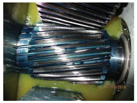
Photo M11 South Span Drive Reducer. The reducer gear teeth have minor damage that may be from particles passing through the mesh.
