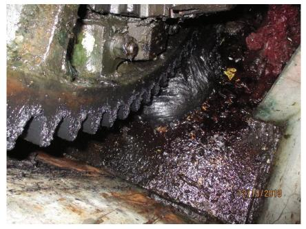
Photo M9 G2/P2-NE, Support Frame. There was an accumulation of old grease within the support frame under the G2 gear.
