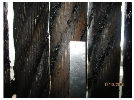
Photo M20 NE-OB Counterweight Ropes. The maximum counterweight rope wear flats were measured to be 5/8".
