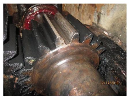
Photo M6 Pinion P2-SE-OB. The gear teeth in the acceleration zone were cleaned to bare metal for inspection.
