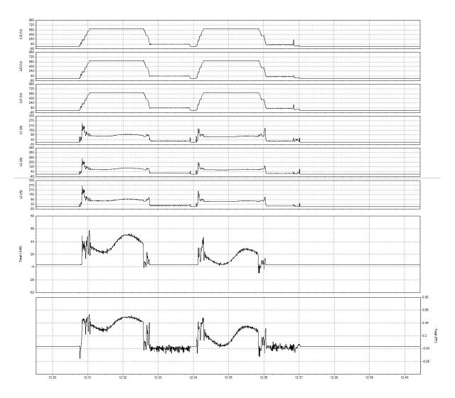
Figure E5: Voltage, Current, and Power Parameters (North Tower West Span Drive Motor – Generator Power).
