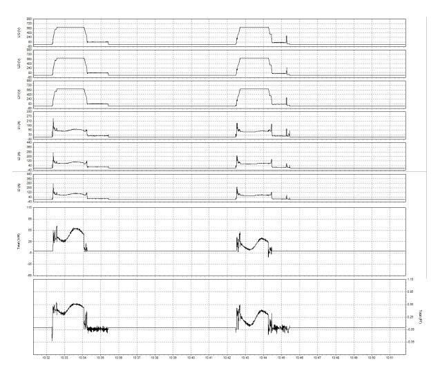
Figure E1: Voltage, Current, and Power Parameters (North Tower West Span Drive Motor – Normal Power).
