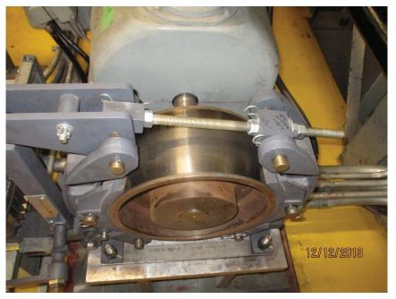
Photo M3 Motor Brake-SE. General view of the brake wheel friction surface. The brake wheel hub is unpainted.
