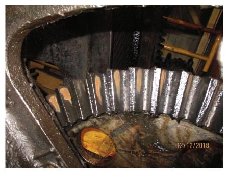
Photo M8 Gearset G2/P2-NW, Differential Gear. There was corrosion on some of the differential gear teeth due to inadequate lubricant
