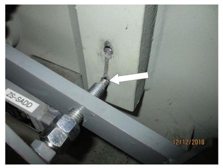
Photo M17 South Primary Reducer Auxiliary Drive Engagement Lever. Note the positioning bolt used to secure the lever in the engaged and disengaged position does not line up with the hole (arrow), preventing the bolt from being inserted in the hole with the lever locked in the disengaged position.
