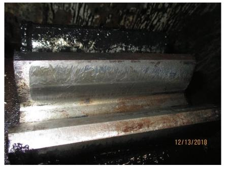
Photo M7 P1-NW-OB. Damage to the gear tooth caused by wire intrusion is wearing in.
