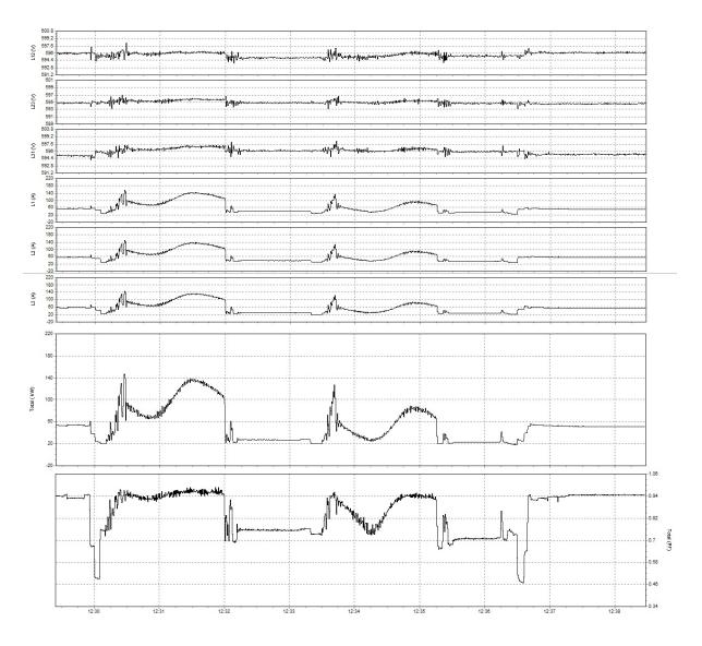
Figure E6: Voltage, Current, and Power Parameters (Generator Output).
