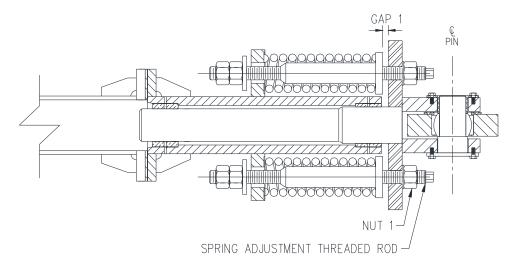
during the 2018 detailed inspection to ensure the preload has not changed since adjustment. All four corners were found to have remained the same.
