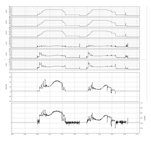
Figure E3: Voltage, Current, and Power Parameters (North Tower East Span Drive Motor – Normal Power).
