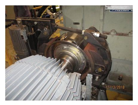
Photo M1 Machinery Brake - NW and Brake Wheel Coupling C3-NW. General view of the machinery brake assembly. Note the unpainted brake wheel coupling bolts.
