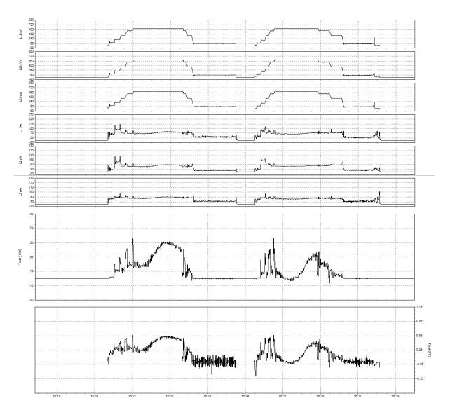
Figure E4: Voltage, Current, and Power Parameters (South Tower West Span Drive Motor – Normal Power).
