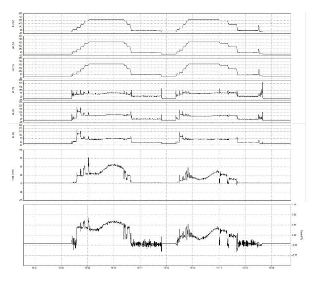
Figure E2: Voltage, Current, and Power Parameters (South Tower East Span Drive Motor – Normal Power).
