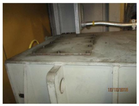
Photo M12 North Span Drive Reducer. The inspection cover screws have damaged threads.
