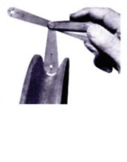
FIGURE 4 – Illustration of Sheave Groove Wear
