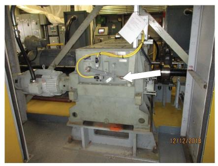
Photo M16 South Primary Reducer Auxiliary Drive Engagement Lever. Note the lever (arrow) is shown in the locked disengaged position. See Photo M17 for a close-up of the positioning bolt intended to additionally secure the lever in the disengaged position.
