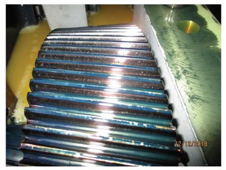
Photo M10 South Span Drive Reducer. The reducer gear teeth have minor damage that may be from particles passing through the mesh.
