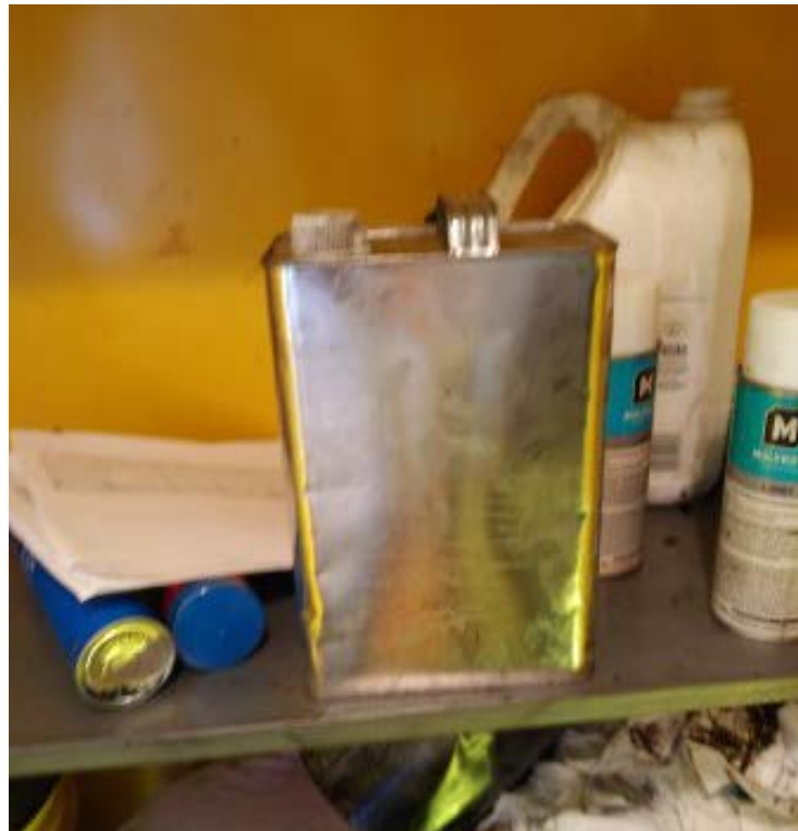
Figure 1: Example of unlabeled hazardous product (presumed) container in flammable storage cabinet of old workshop.
