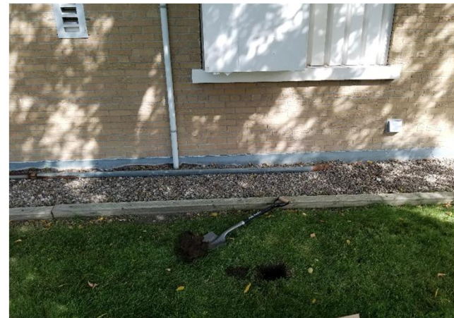
Location of soil sample TH2-A, depth 5 to 15 cm below grade. Soil sample was determined to have a total lead concentration of 19 mg/kg.
