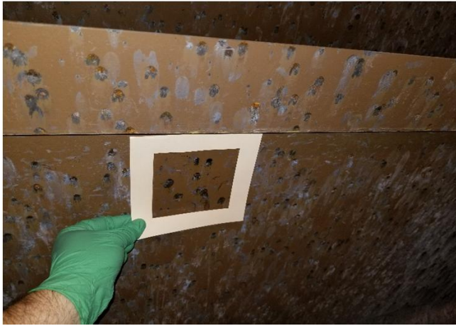
Sample LW-21 swipe from the wall of the bullet trap in the firing range was determined to have a total lead concentration of 2,840\mu\text{g}/100\text{cm}^2 .
