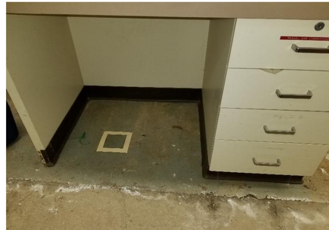
Sample LW-25 swipe from the concrete floor in the observation room north of the firing range was determined to have a total lead concentration of 1,130\mu\text{g}/100\text{cm}^2 .
