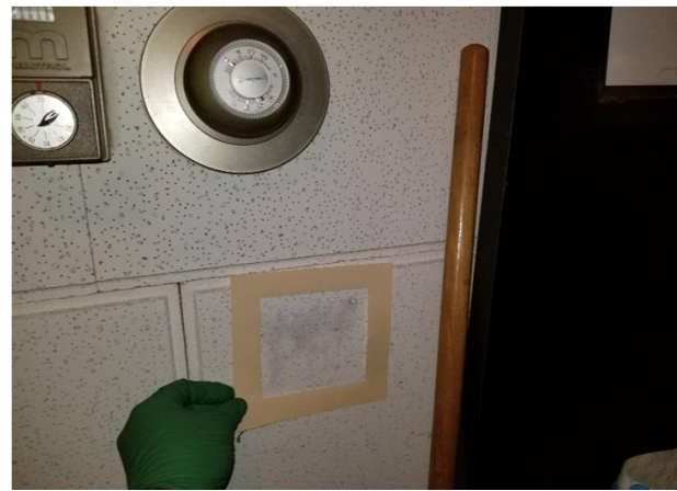
Samples LW-16 and LW-32 swipes from the wall beside the east firing position in the firing range were determined to have total lead concentrations of 43.9\mu\text{g}/100\text{cm}^2 and 148\mu\text{g}/100\text{cm}^2 respectively.
