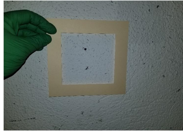
Sample LW-22 swipe from the east wall down range in the firing range was determined to have a total lead concentration of 1,110\mu\text{g}/100\text{cm}^2 .
