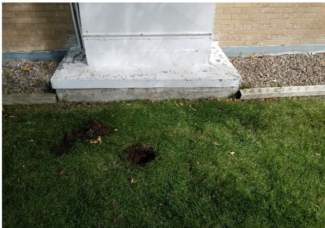
Location of soil sample TH1-A depth 5 to 15 cm below grade. Soil sample was determined to have a total lead concentration of 22 mg/kg.
