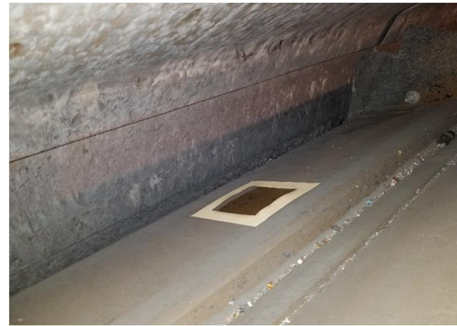
Sample LW-34 swipe from the base of the bullet trap in the firing range was determined to have a total lead concentration of 14,100µg/100cm 2 .
