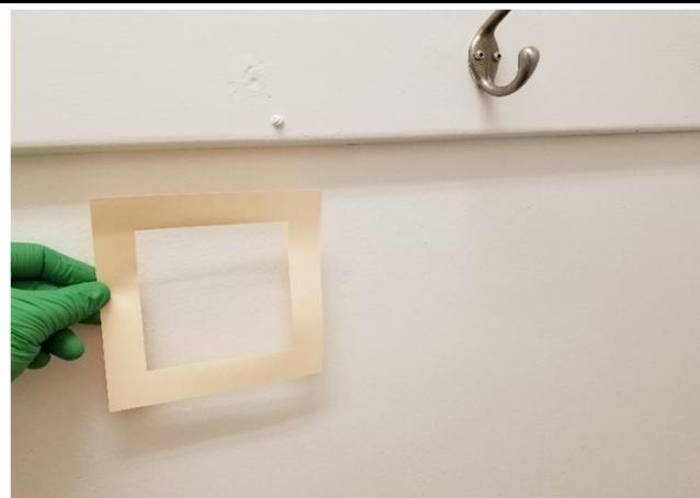
Sample LW-06 swipe from west gypsum board wall in the freezer room was determined to have a total lead concentration of 5.96\mu\text{g}/100\text{cm}^2 .
