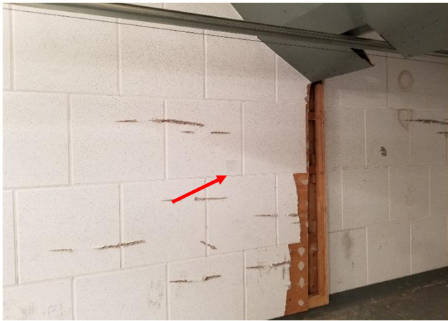
Sample LW-33 swipe from the east wall near the centre of the firing range was determined to have a total lead concentration of 55.6µg/100cm 2 .
