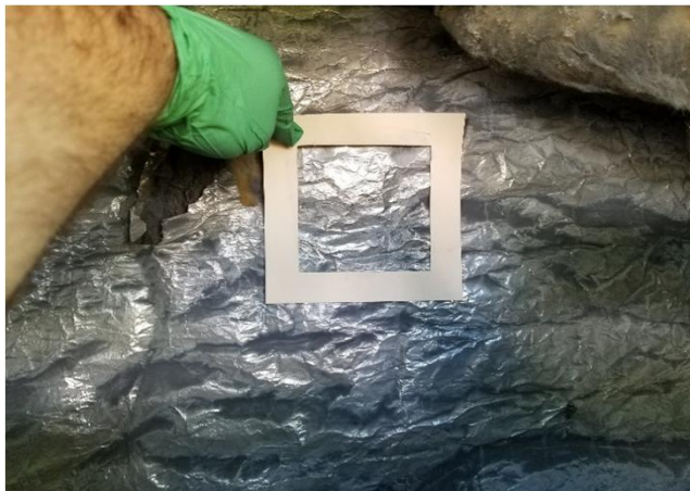
Sample LW-03 swipe from the interior wall (fibreglass insulation) of the south exterior duct was determined to have a total lead concentration of 22,000\mu\text{g}/100\text{cm}^2 .
