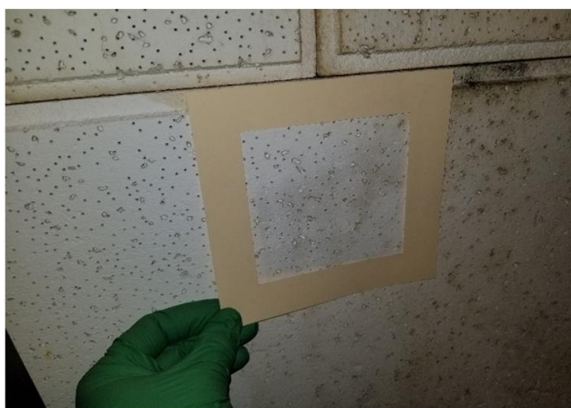
Sample LW-15 swipe from the wall beside the west firing position in the firing range was determined to have a total lead concentration of 20.0\mu\text{g}/100\text{cm}^2 .
