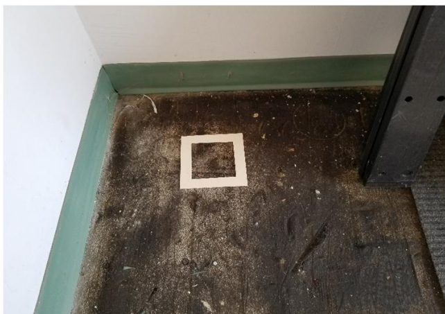
Sample LW-05 swipe from concrete floor in the northwest corner of the north garage bay was determined to have a total lead concentration of 16.2\mu\text{g}/100\text{cm}^2 .
