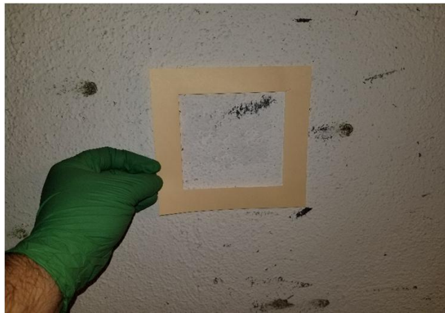
Sample LW-23 swipe from the west wall down range in the firing range was determined to have a total lead concentration of 3,400\mu\text{g}/100\text{cm}^2 .
