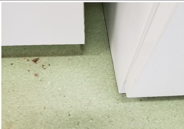
Sample LW-05 swipe from concrete floor in the northwest corner of the north garage bay was determined to have a total lead concentration of 16.2\mu\text{g}/100\text{cm}^2 .
