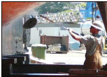
A small vessel is power washed on the North Landing Wharf (NLW).
