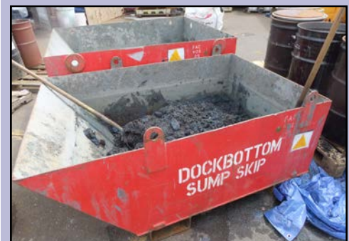
ADEQUATE waste grit storage.
