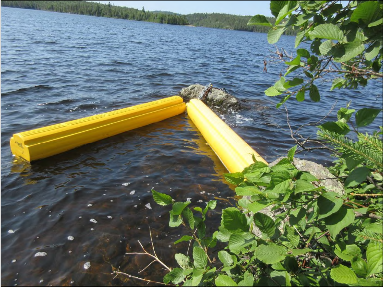
Figure 6: Close-up view of waterway barrier in water, attached to an anchor rock.
