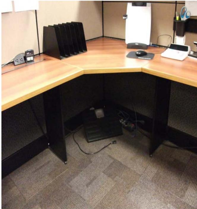
Configuration #2– workstations with work surfaces (typically 2 work surfaces) that have no corner work surface but have a metal corner piece added to the work surfaces creating a 45degree angle. These work surfaces do not require any modifications to the work surfaces. Work surfaces need to be fused together to create a one-piece height adjustable work surface.
