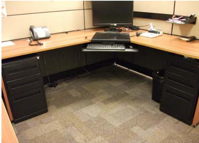
Configuration #3 - workstations that require some minor modifications to the work surfaces. Centre work surfaces need to have a metal plate added in order to fill in the keyboard cut-out that is currently there. All work surfaces need to be fused together to create a one-piece height adjustable work surface.
