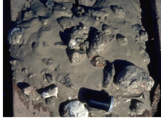
d) Gravelly silty sand till when thawed illustrating high water content
