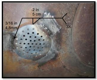
2.2. The last part to complete will be to weld the hatches and stowage compartment closed. For the Commander and Loader hatches, weld three plates in order to secure the hatch. Cut the locking part of the handle and weld in place. (Appendix 3 need to be completed before this step).
