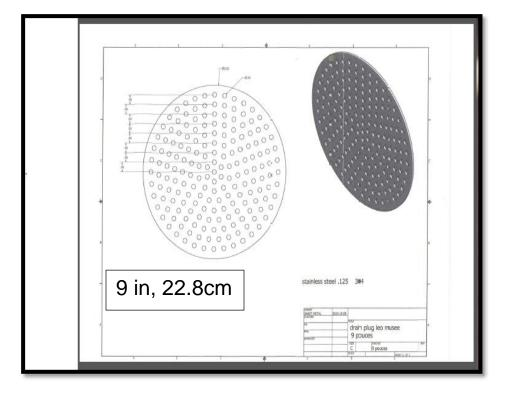
2.1.3.2. Install the 9 inches plate (22.8 cm) # 108083353 at the back as shown below. Weld in three locations at angle with 3/16 (4.8mm) diameter and 2.5 in (6.3cm) long.
