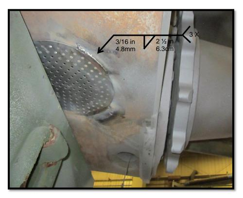
2.1.3.3. Install on the opposite side the 9 inches plate (22.8 cm) # 108083353 at the back as shown below. Weld in three locations at angle with 3/16 (4.8mm) diameter and 2.5 in (6.3cm) long.
