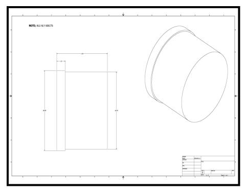
5.10. The plugs will be installed and welded in place
