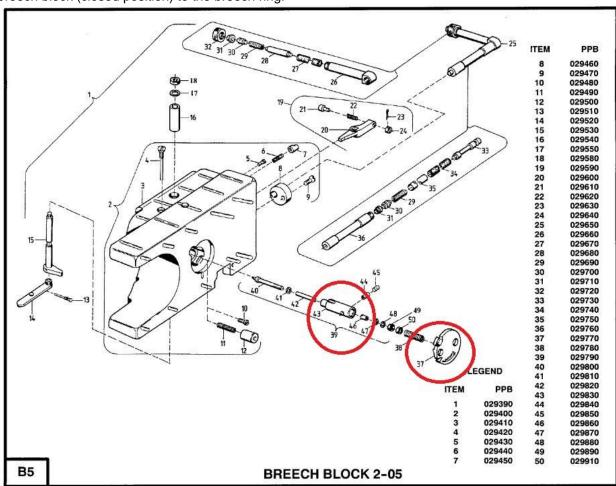
5.5. Replace the cap item 37 and weld the cap to the breech block, replace the breech block and weld the breech block (closed position) to the breech ring.
