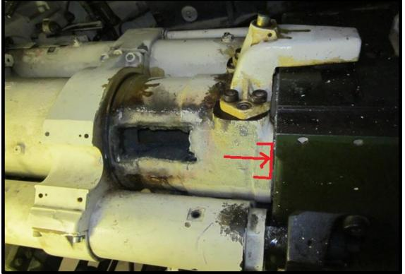
5.4. Remove the breech block, remove the cap item 37, remove and discard needle assy item 39, see diagram at para 5.6 below.
