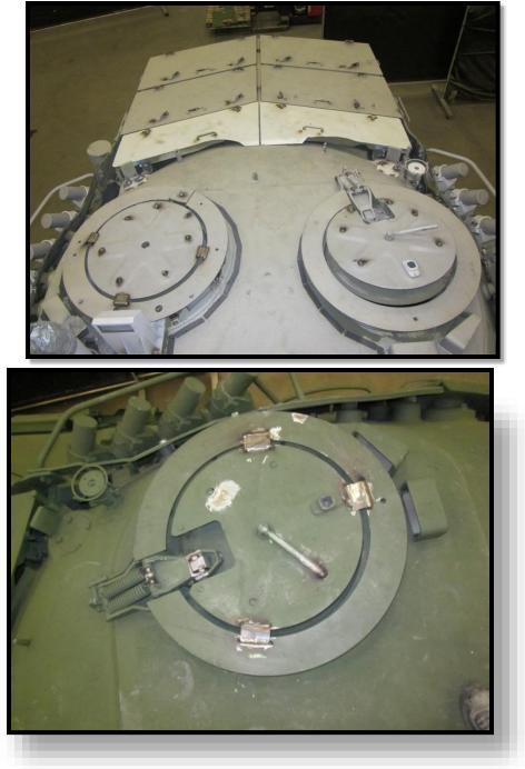
2.3. For the Drivers hatch, close the hatch and weld the hatch locking mechanism in place.
