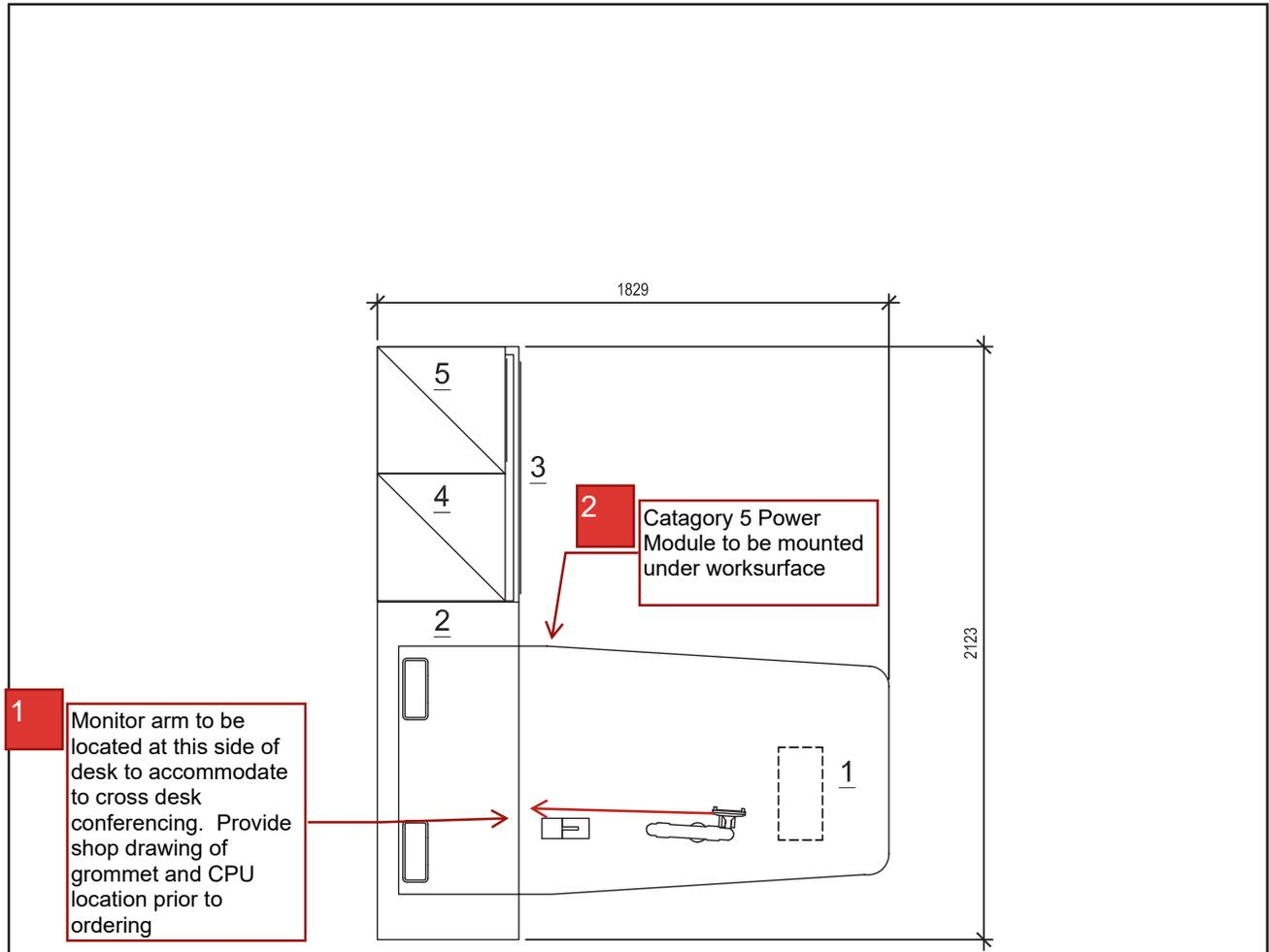
**1** Monitor arm to be located at this side of desk to accommodate to cross desk conferencing. Provide shop drawing of grommet and CPU location prior to ordering
