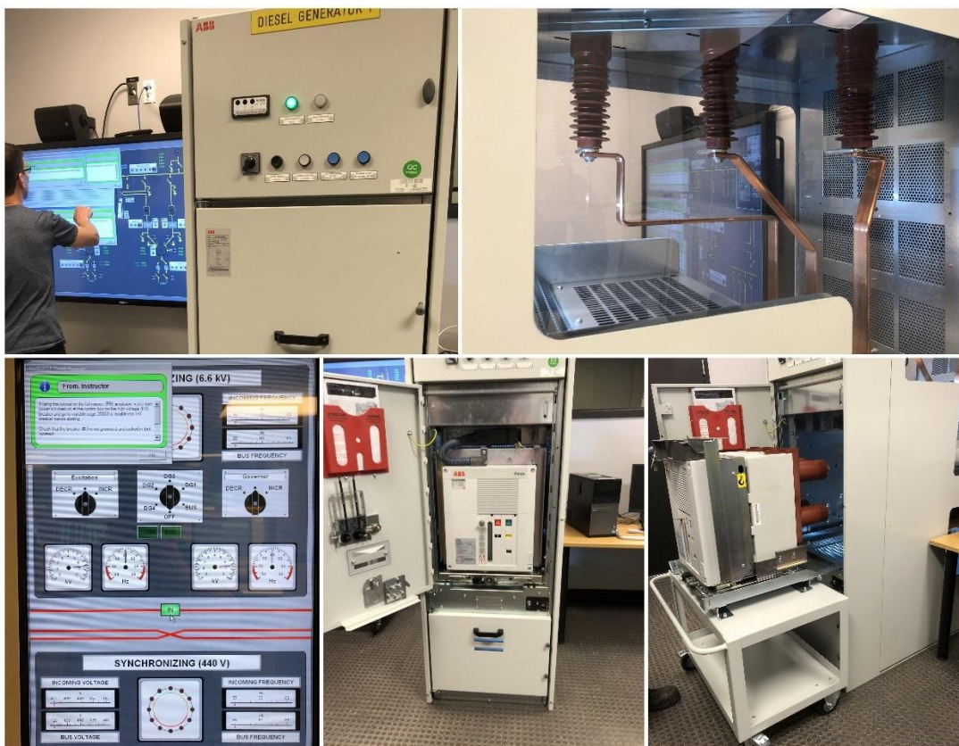
Figure 6-5: Shore-Based Individual Trainer - High Voltage Trainer
