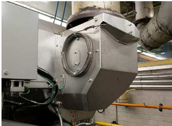
Picture 1. Example of a pre-wired sensor including the cable temporarily located close to the turbo charger
