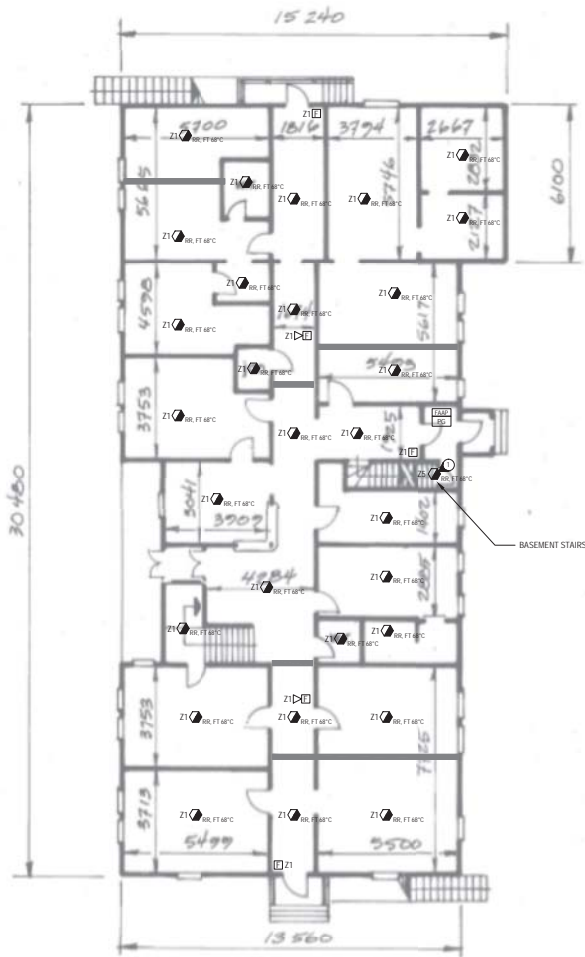
2 E110 NEW FIRE ALARM LAYOUT - GROUND FLOOR - ZONE 1 SCALE: 1:100
