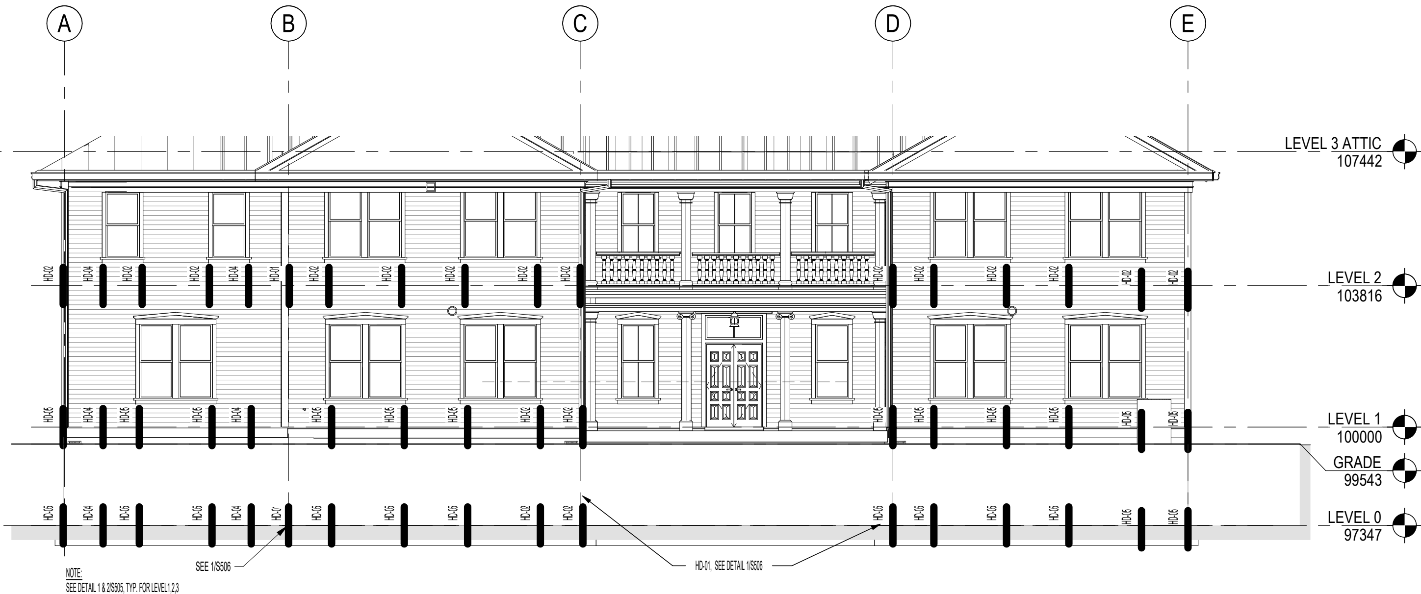
4 GL-1 - HOLDOWN LAYOUT DIAGRAM
