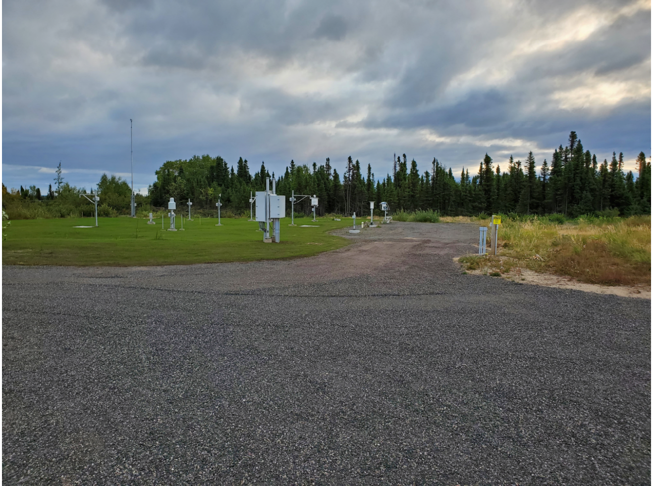
Instrument Compound, snow blow / plow area to the right of the sensors – the gravel portion of the driveway. Do not plow or snow blow snow towards the instruments.
