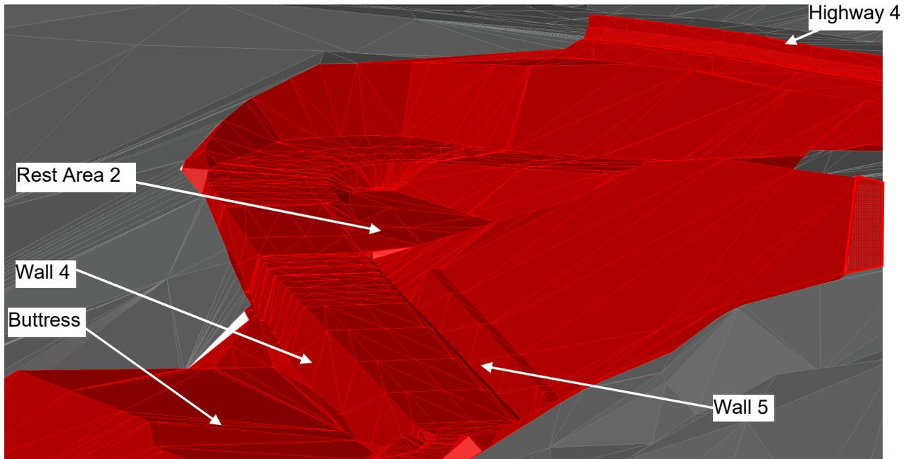
**Figure A2-1A** 3D Rendering of proposed trail looking northwest at upper switchback and Rest Area 2. Buttress to left, high to right. Image provided by Parsons.
