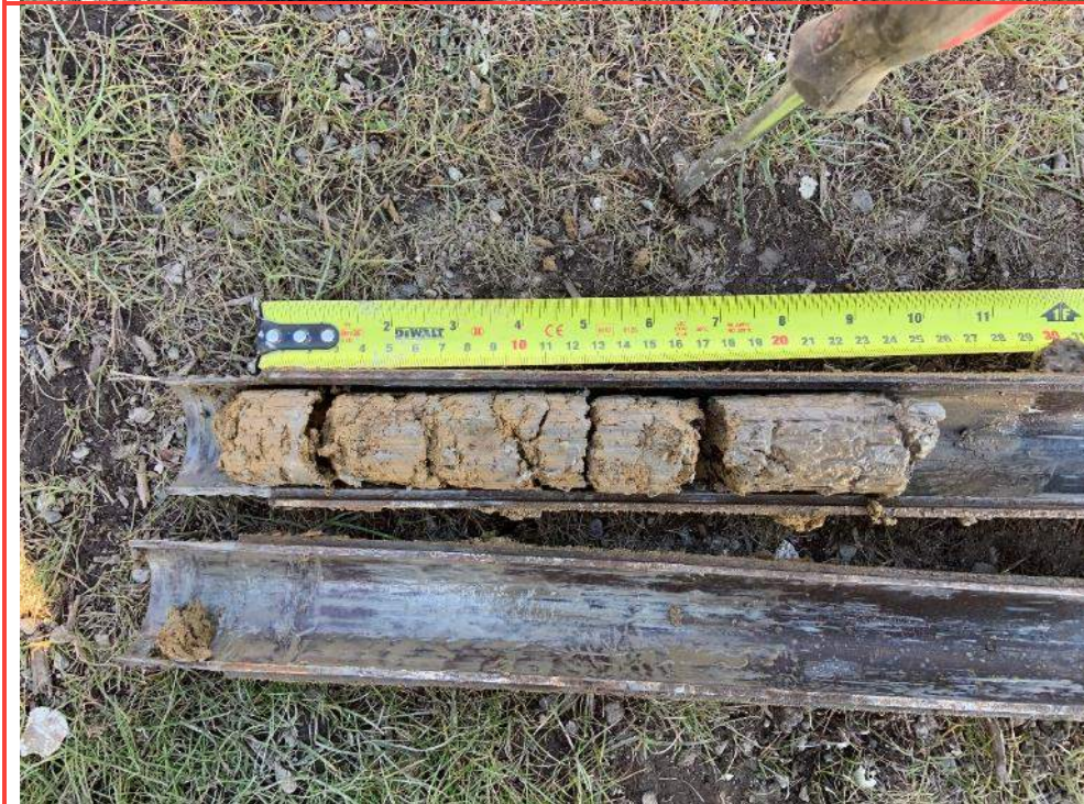
Photo 58: SPT sample at 3.9m from BH20-02.
