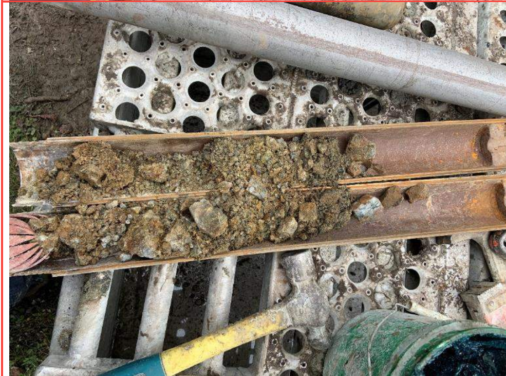
Photo 48: SPT sample from sand and gravel till within BH20-01A.
