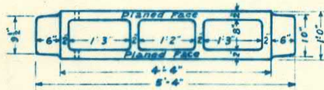
TOP VIEW OF CENTRE CASTING
