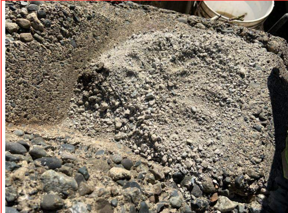
Photo 42: Light grey sand and gravel retrieved from ODEX drilling of BH20-01.
