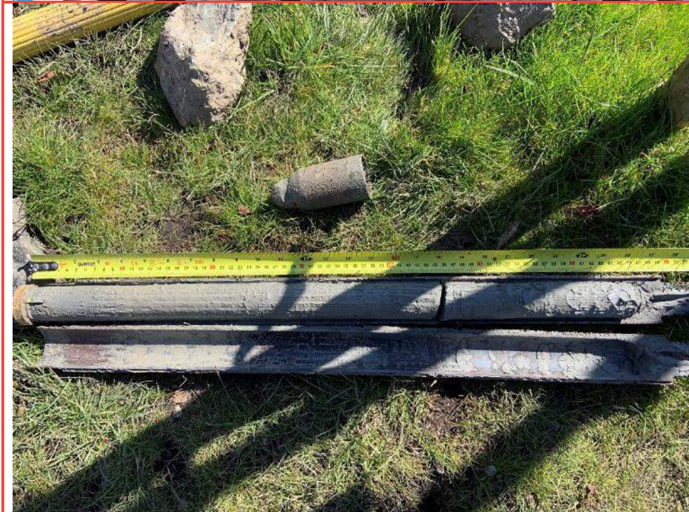
Photo 54: SPT sample at 12.2m from BH20-03.
