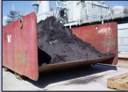
Store waste grit in appropriate containers.
