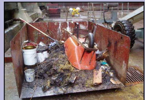
INADEQUATE waste grit storage.
