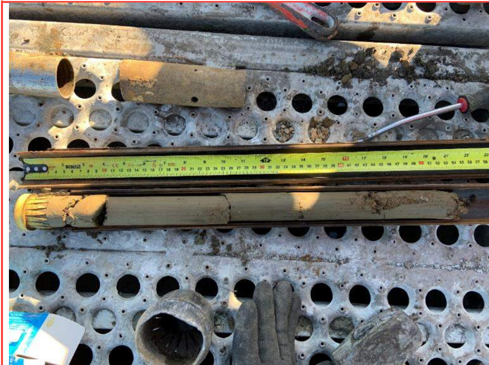
Photo 53: SPT sample at 7.3m from BH20-03
