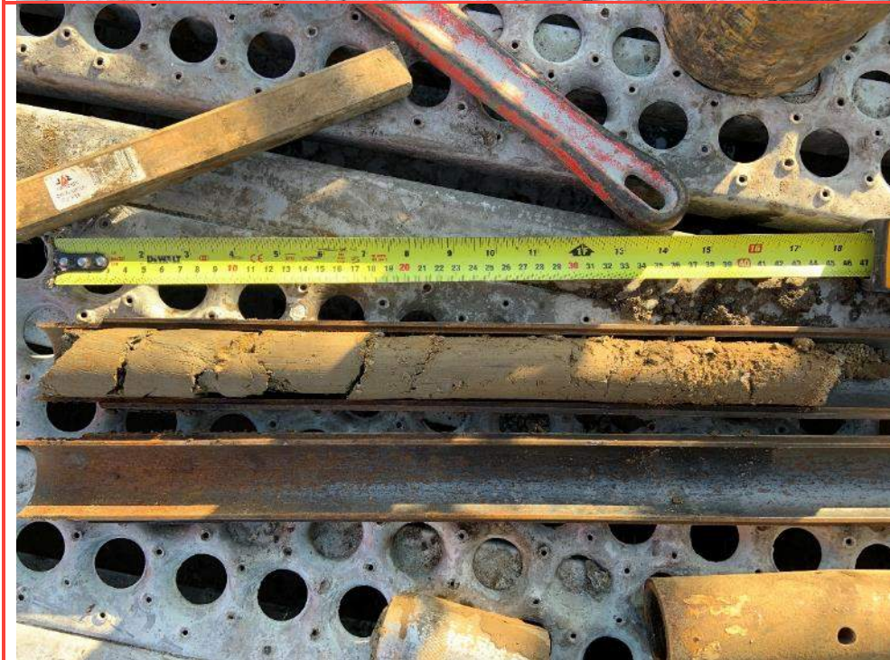
Photo 52: SPT sample at 6.7m from BH20-03
