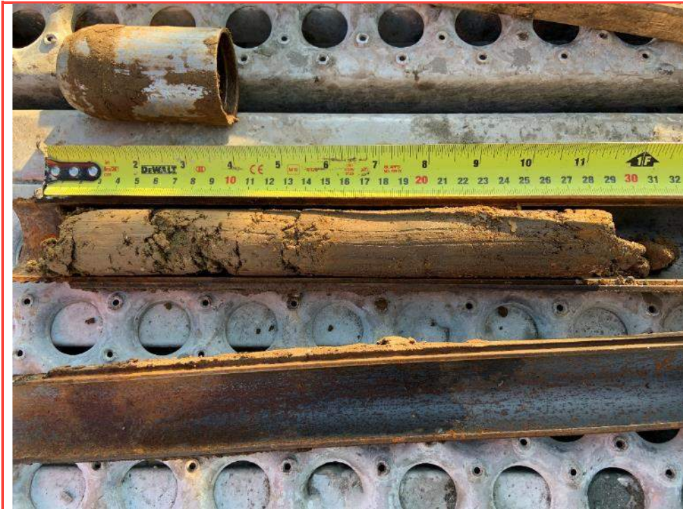
Photo 51: SPT sample at 6.1m from BH20-03
