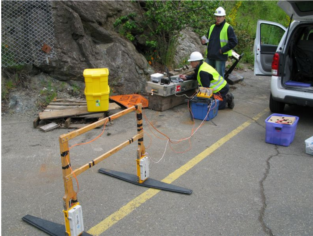
Photo 1: Assembling 100 MHz equipment
