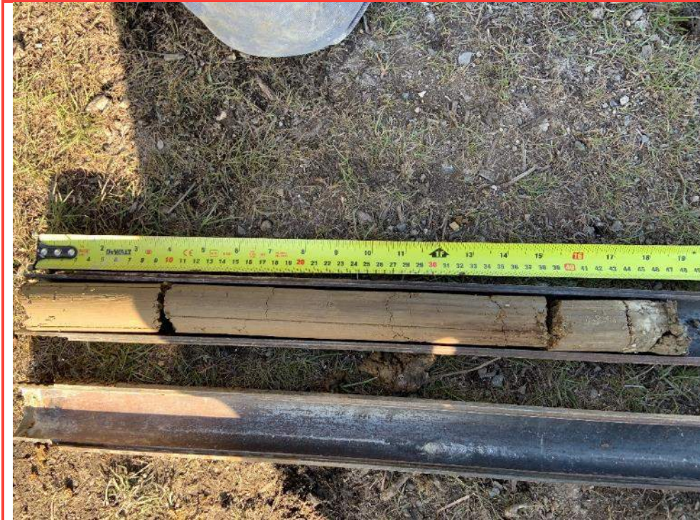
Photo 59: SPT sample at 4.9m from BH20-02.
