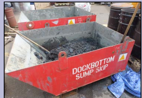
ADEQUATE waste grit storage.
