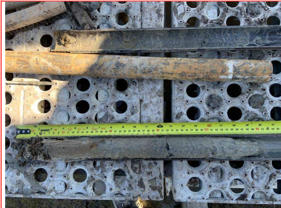
Photo 55: SPT sample at 13.2m from BH20-03.
