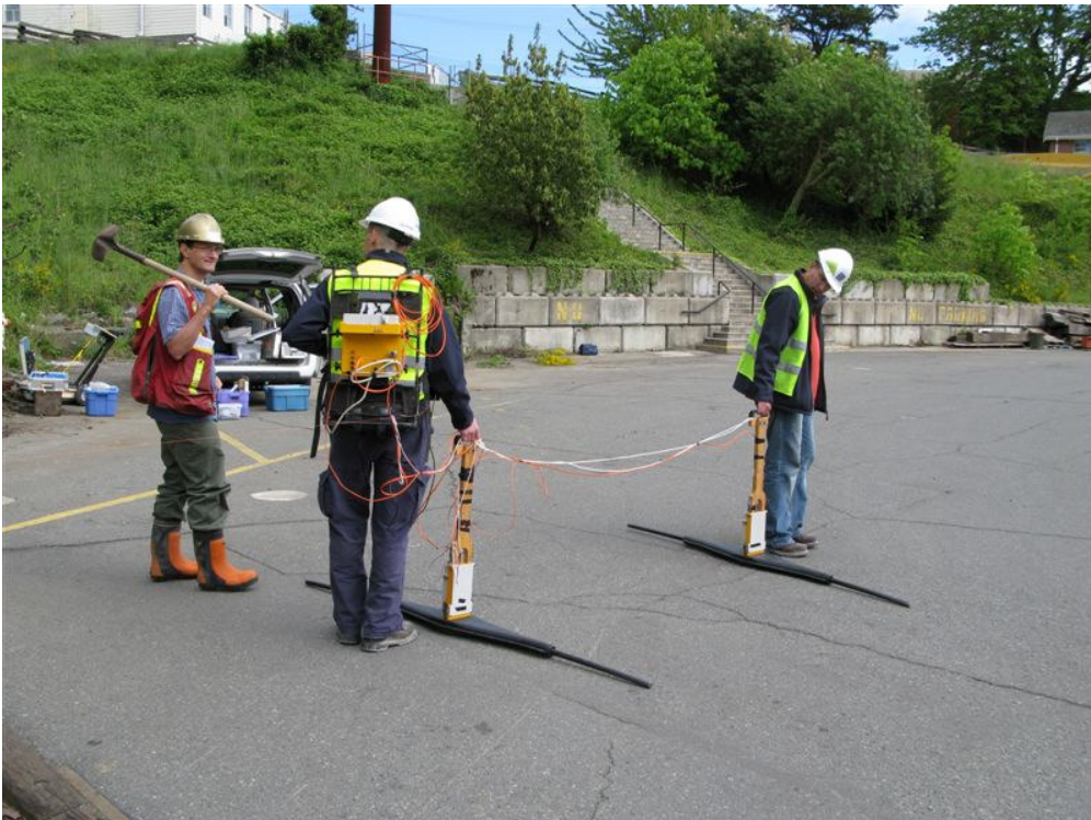
Photo 4: Carrying 50 MHz equipment along east end of drydock
