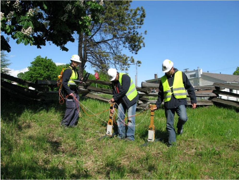
Photo 3: Carrying 100 MHz equipment on slope.
