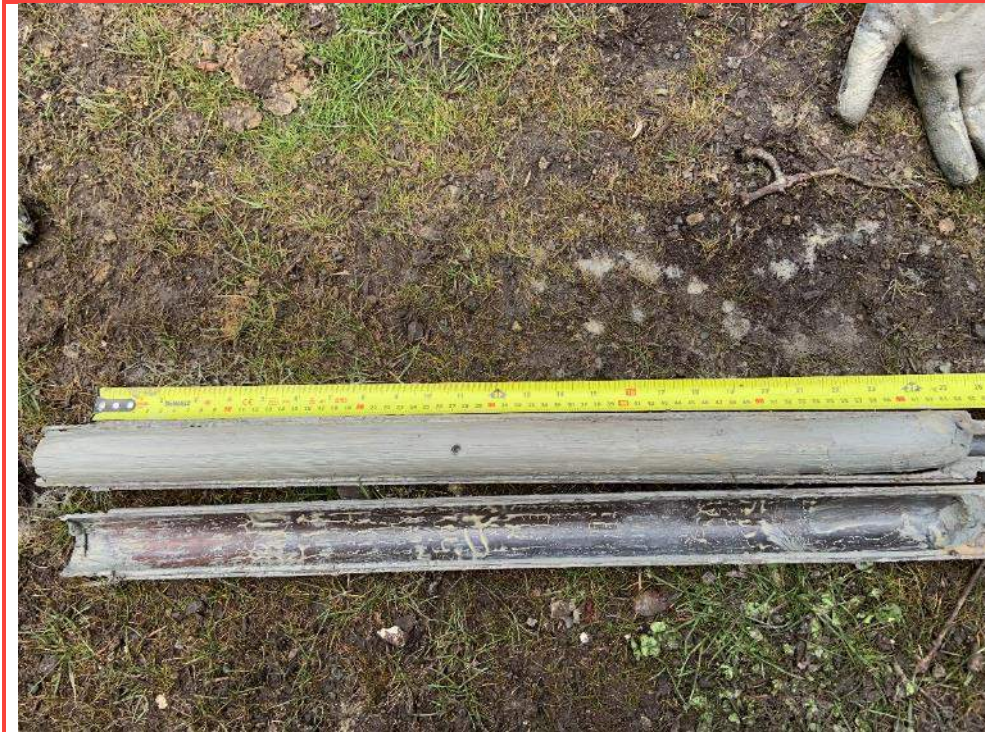
Photo 61: SPT sample at 9.1m from BH20-02.
