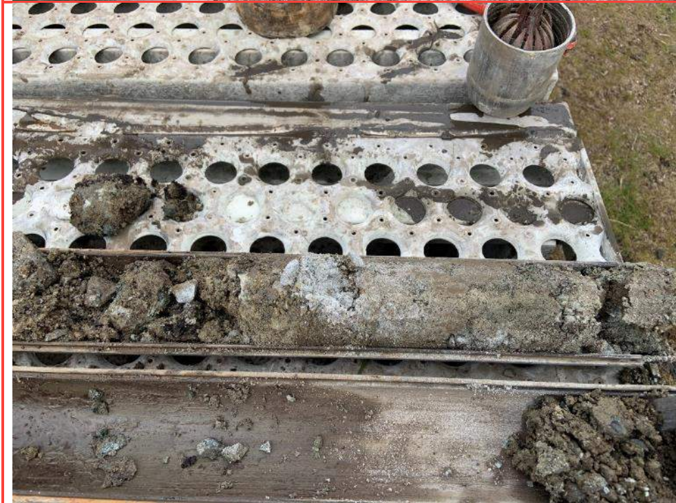
Photo 50: SPT sample at 4.0m from BH20-03
