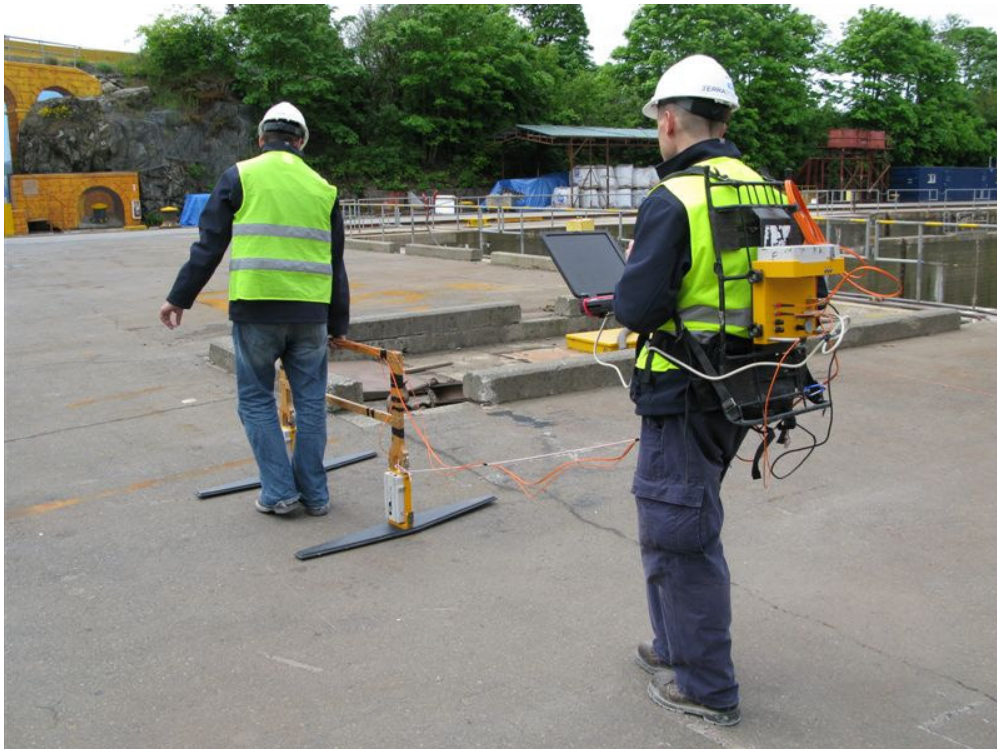
Photo 2: Carrying 100 MHz equipment across east end of dry dock
