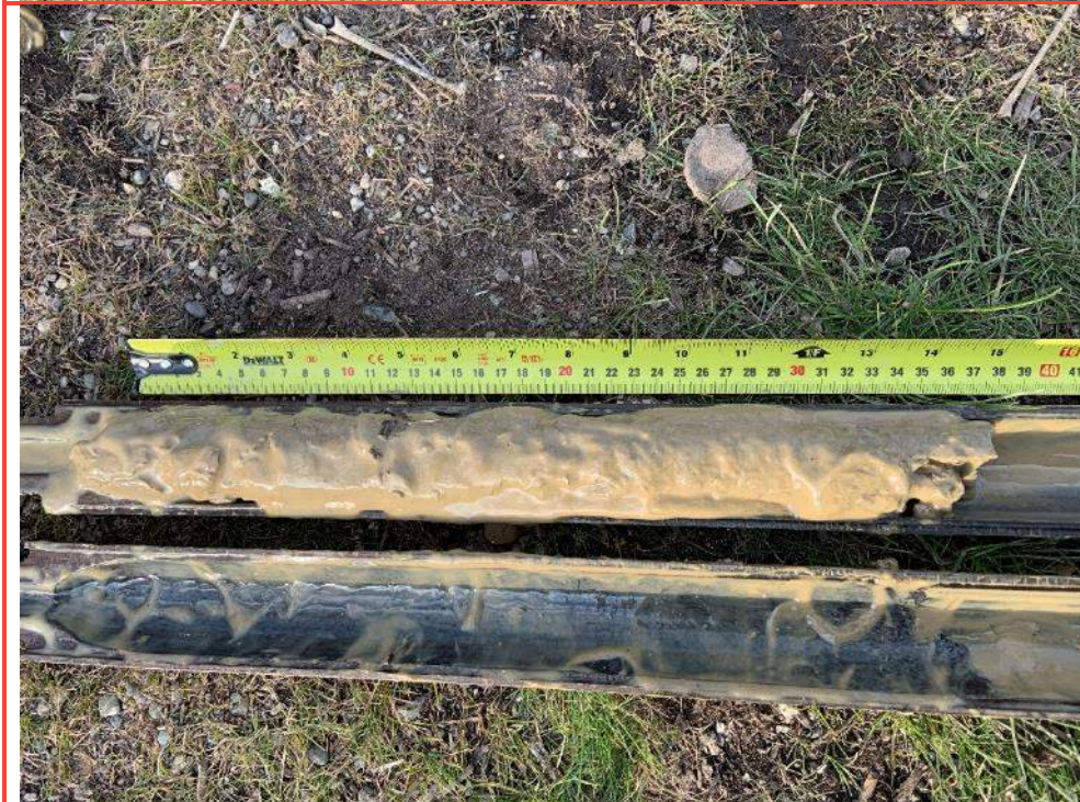
Photo 60: SPT sample at 6.1m from BH20-02.
