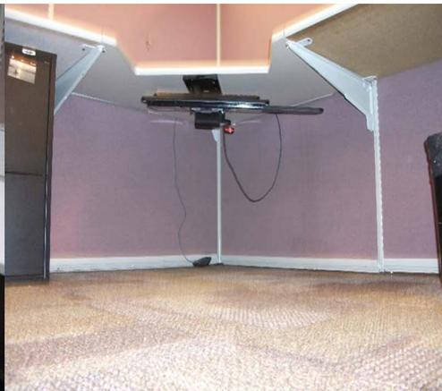
Configuration #4 - workstations that require some modifications to the work surfaces. Centre work surfaces currently have a height adjustable keyboard table. Options and/or solutions will need to be provided in order to create a fused together one-piece height adjustable work surface.
