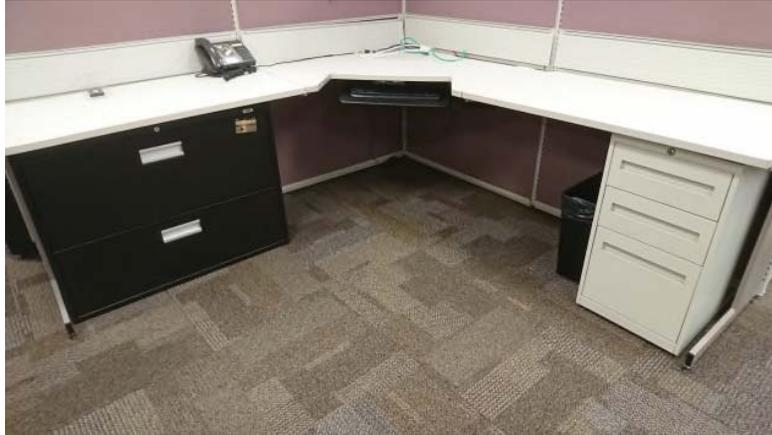
Configuration #2 - workstations that require some modifications to the work surfaces. Centre work surfaces currently have a height adjustable keyboard table. Options and/or solutions will need to be provided in order to create a fused together one-piece height adjustable work surface.
