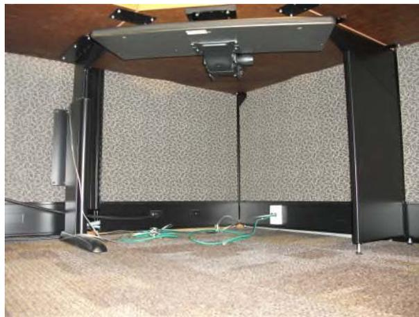
Configuration #2– workstations with work surfaces (typically 2 work surfaces) that have no corner work surface but have a metal corner piece added to the work surfaces creating a 45degree angle. These work surfaces do not require any modifications to the work surfaces. Work surfaces need to be fused together to create a one-piece height adjustable work surface.
