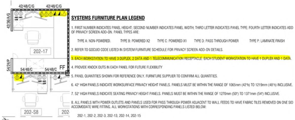
In the images above, highlighted yellow are the power/data/voice provided from the panels. The 2 additional power symbols that are not highlighted come from ACC2, a workstation accessory (a surface-mounted power module with AC and USB). Note this is indicated in furniture plans (see plan and furniture schedule below for reference). Refer to revised drawings and Table 1 issued as part of this amendment.
