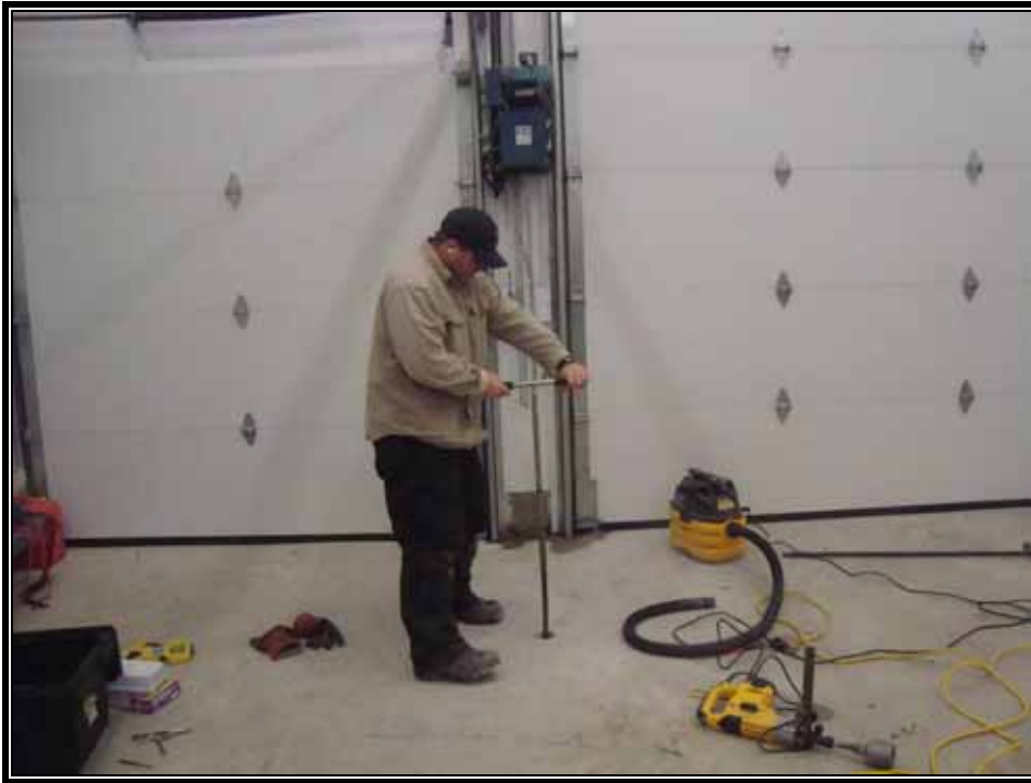
Photo 9: Soil sampling LEWI-58590-09-TH01-01 performed in the garage of the St. Lewis Field Office.
