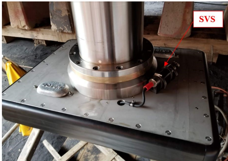
Figure 1: SVS mounting configuration on transducer pod assembly
