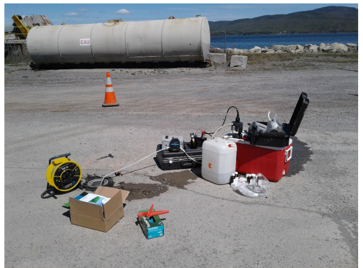
PHOTO 42 Sampling of observation well P003-68 – June 7, 2019
