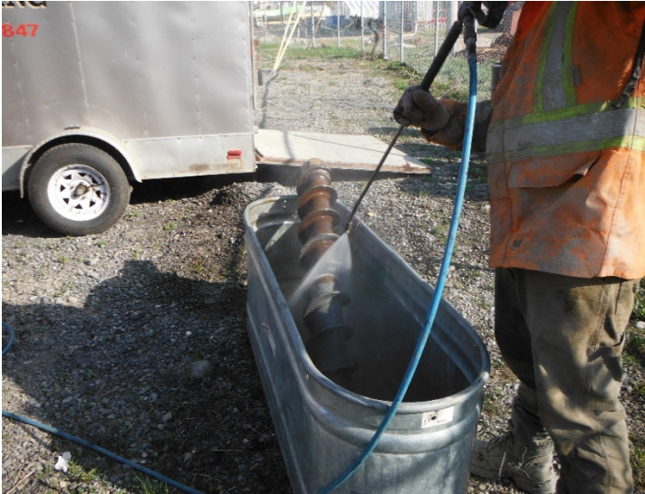
PHOTO 51 Methodology for cleaning augers
