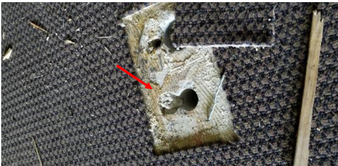
Photo 17: Carpet mastic, associated with carpet materials in the first floor former conference room contains 0.91% Chrysotile asbestos.
